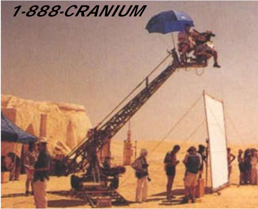
In its longest mode, the Giraffe covers a scene from minus 17 feet to 31 feet, extending manned camera capability well beyond the competition. The Giraffe's unique design makes it unbelievably quick to assemble using a single pocket-size ratchet. One Grip with an assistant can unload, set-up and be ready to roll in approximately ten minutes. The Giraffe is built of Aerospace alloys, stainless steel, with
