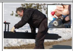
Attach the Balance Rod for Outrigger 150cm to the square end and lock with Quickpin.
