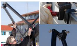
Attach the horizontal connecting rod and lock with Quickpin.
