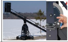
Mount first side of trapezoid to Central Pivot Section. The side of the trapezoid with a receiving pin should face towards the Counterweight Basket.
