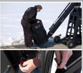
• Level out Counterweight Basket with turnbuckle.
