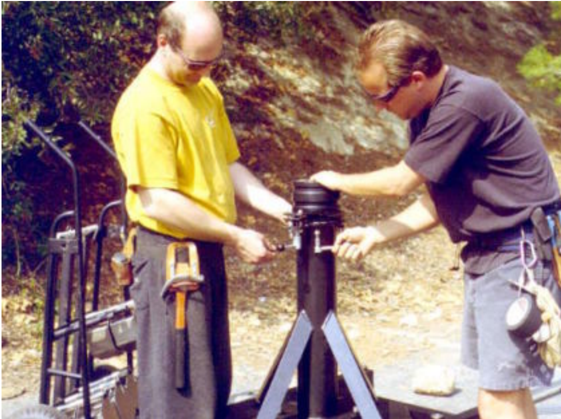
Mode 1 - Remote - Step 10: Tighten 4 bolts that hold bearing into mini post.
