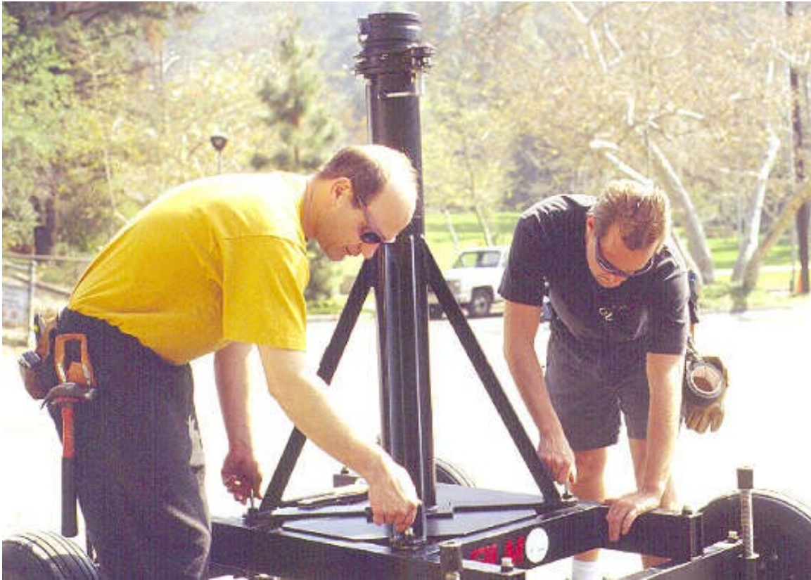
Mode 1 - Remote - Step 3: Unbolt main post.
