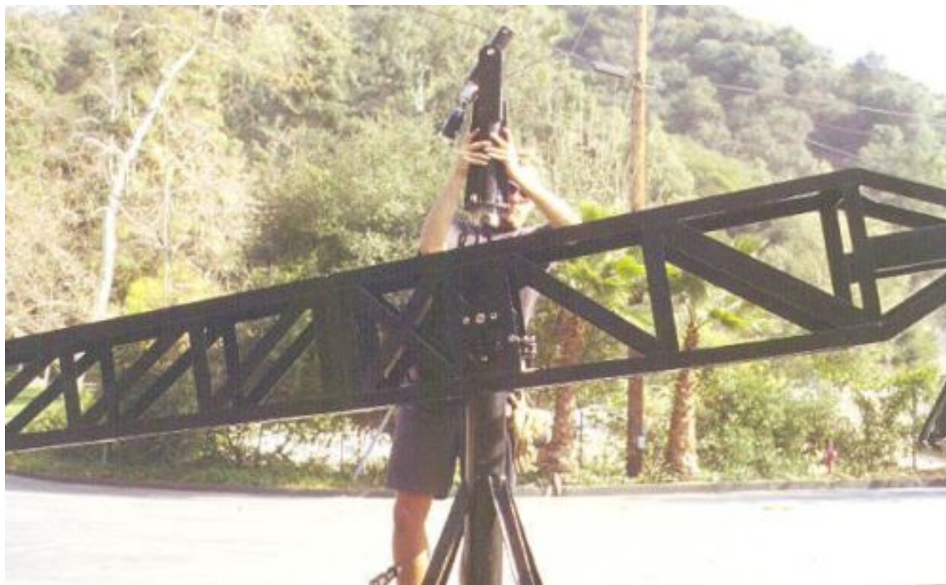
Mode 5 - Remote only - Step 5: Attach pylon assembly onto main post with 4 bolts, captivating the horizontal main shaft (make sure threaded end of pylon faces forward so you can level the Operating platform later!)
