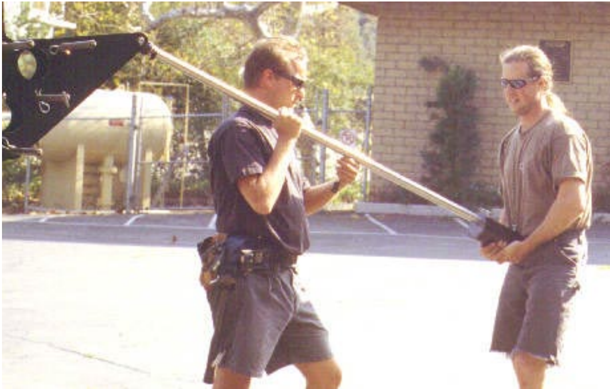
Mode 1 - Remote - Step 15: Attach Rod A (mini rod) to weight box with the quikpin , then add the sliding trim weight. Now attach Rod A to the pylon on the other side with the quikpin.
