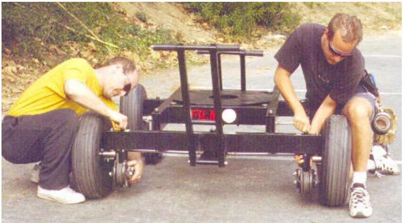
Dolly wide mode - Step 6: Bolt track wheels to crane base crossbar just inside Ruff wheel.
