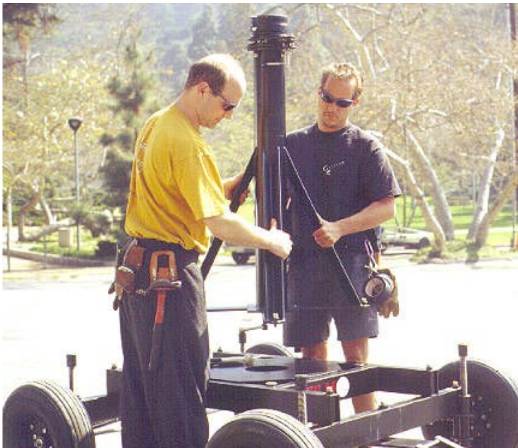
Dolly narrow mode - Step 2: Remove main post.
