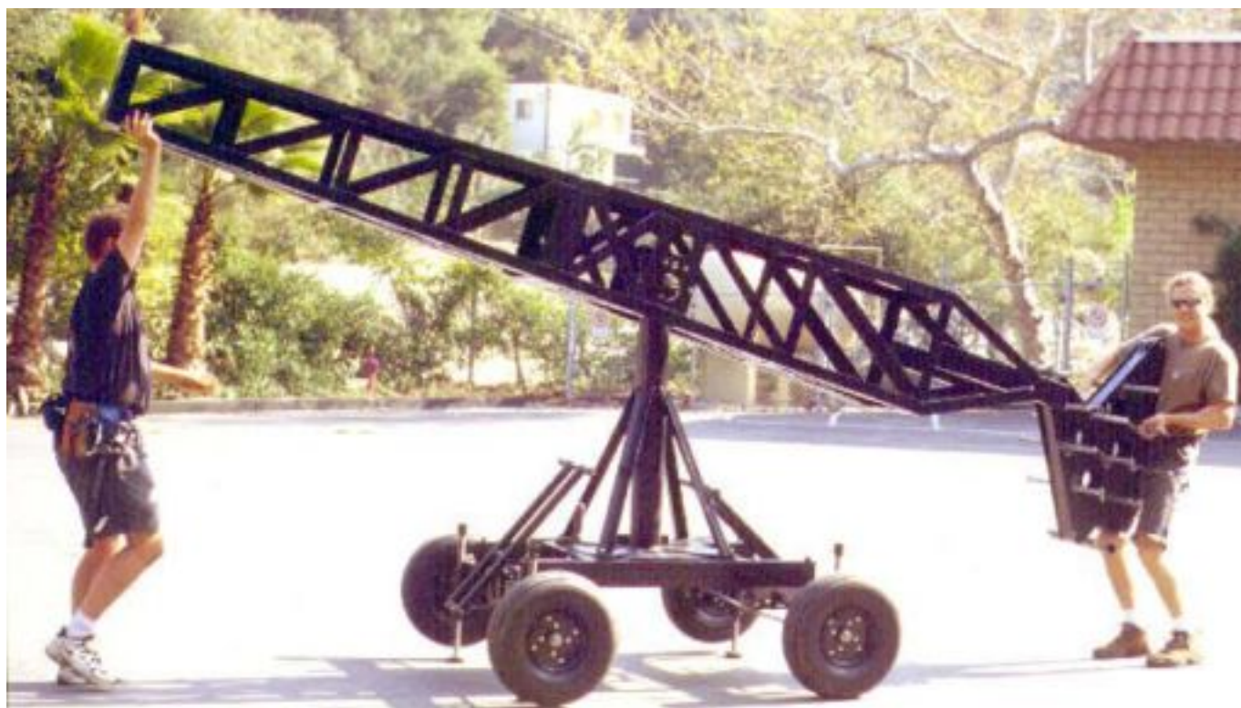
Mode 2 - Remote - Step 6: Add weight box into the slots on the back of Boom #1 and tighten the two retaining bolts (make sure that the weight box shaft isn't resting on the 2 retaining bolts.
