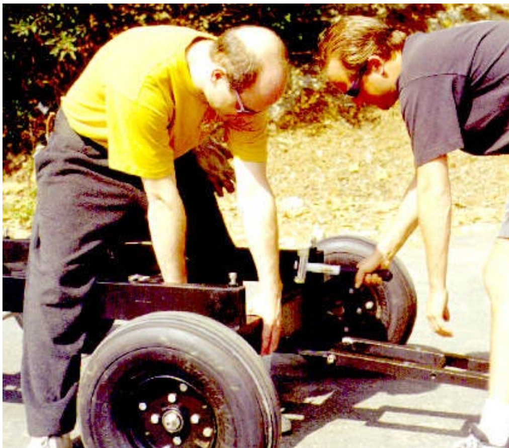
Dolly narrow mode - Step 7: Remove main crossbar (may need plastic mallet to remove).
