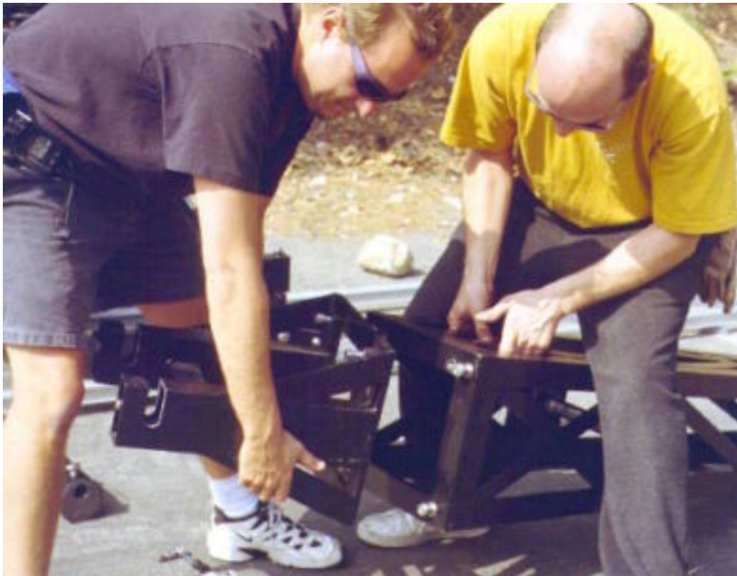
Mode 1 - Remote - Step 11: Attach mini bucket to the back of Boom #3 with 2 retaining bolts on mini bucket.
