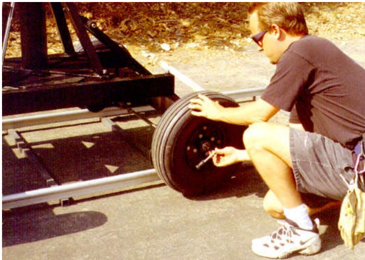
Dolly wide mode - Step 8: Unbolt Ruff wheel (rubber wheel).
