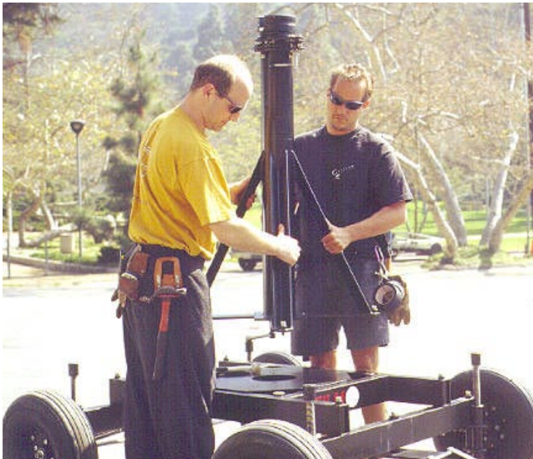
Dolly wide mode - Step 2: Remove main post
