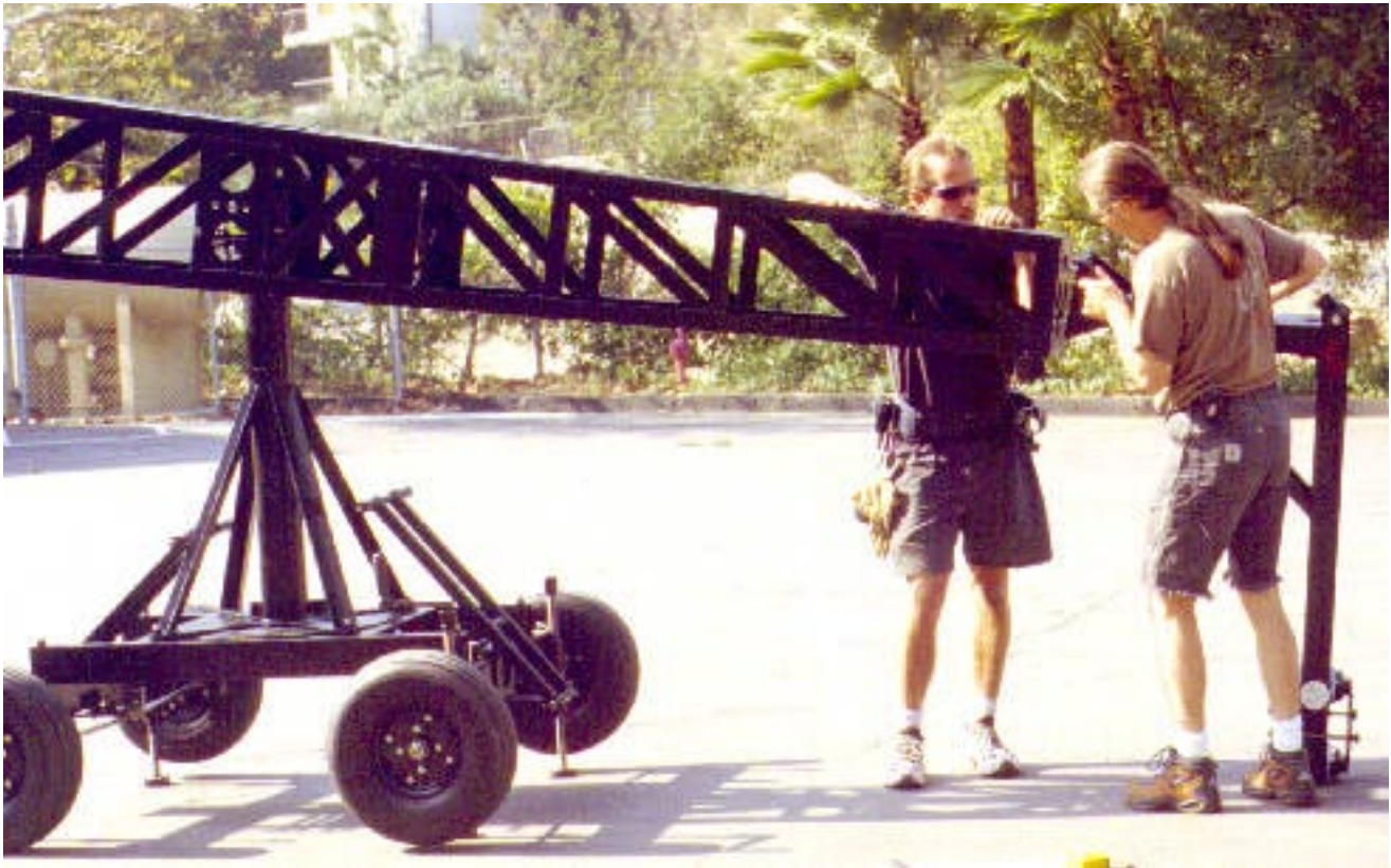
Mode 2 - Remote - Step 11: Secure 2 retaining bolts inside of Boom #2.
