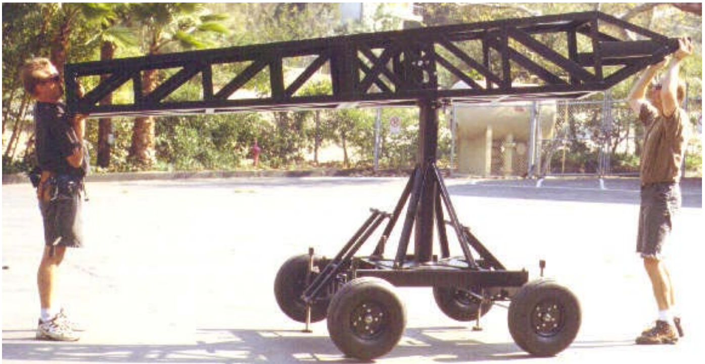
Mode 5 - Remote only - Step 4: Place horizontal main shaft from Boom #1 onto the main post and place the front of Boom #2 onto a ladder for support.
