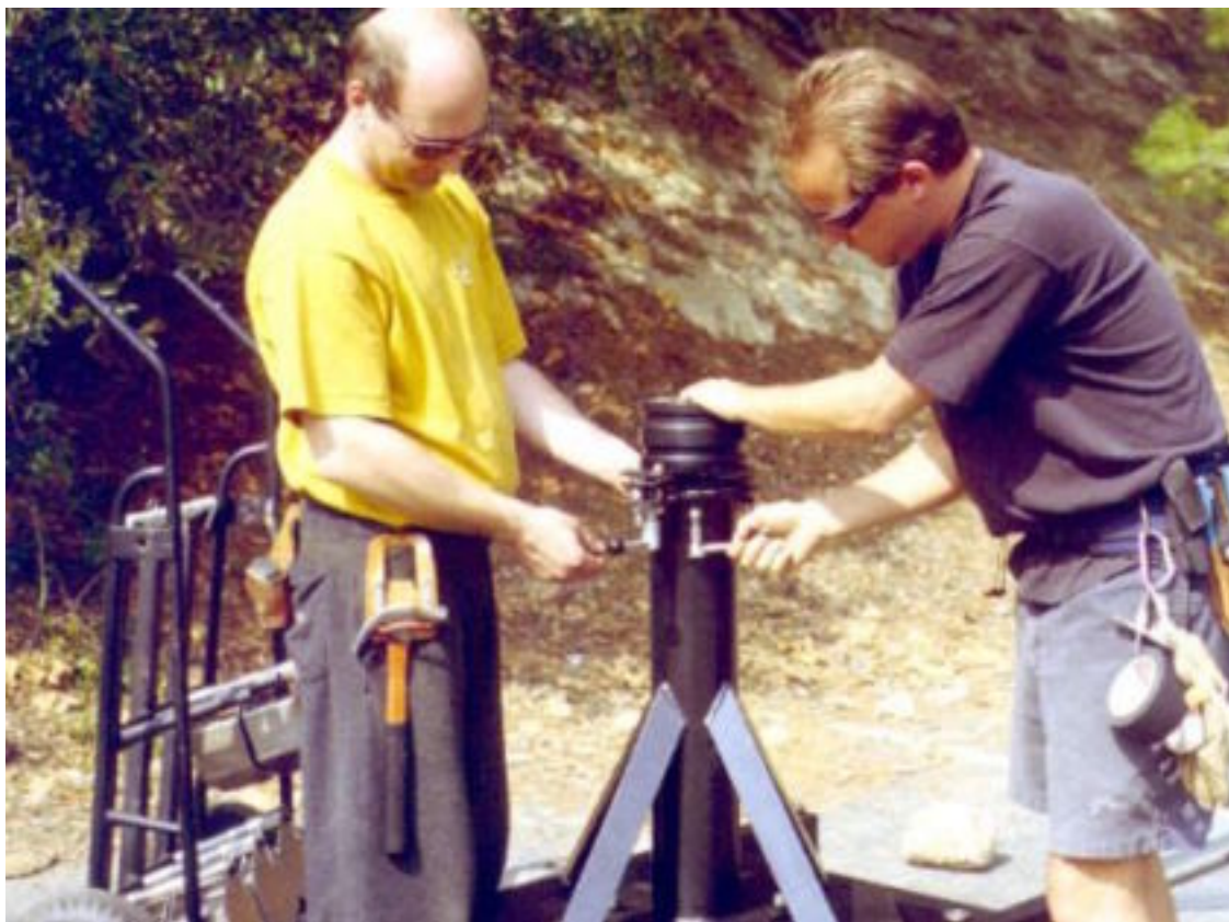
Mode 1+ - Remote Only - Step 10: Tighten 4 bolts that hold bearing into mini post.
