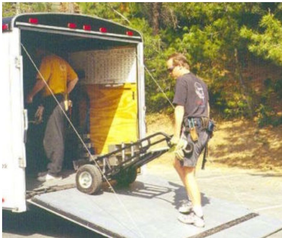
Trailer - Step 7: Unstrap 2" ratchet from weight carts, then disconnect them from each other (make sure you always put weight cart with connectors in middle of two without!)
