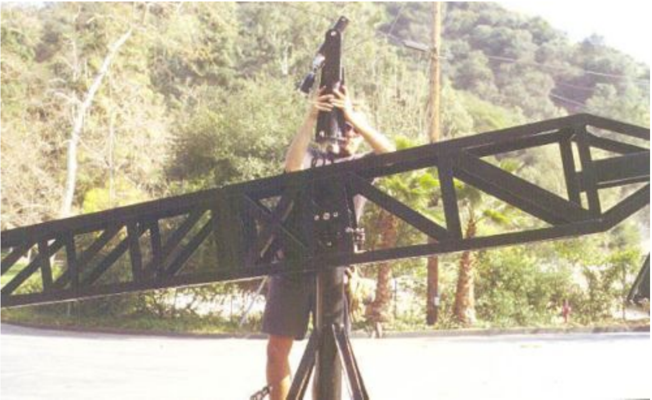
Mode 2 - Operating Platform - Step 5: Attach pylon assembly onto main post with 4 bolts, captivating the horizontal main shaft (make sure threaded end of pylon faces forward so you can level the Operating platform later!)
