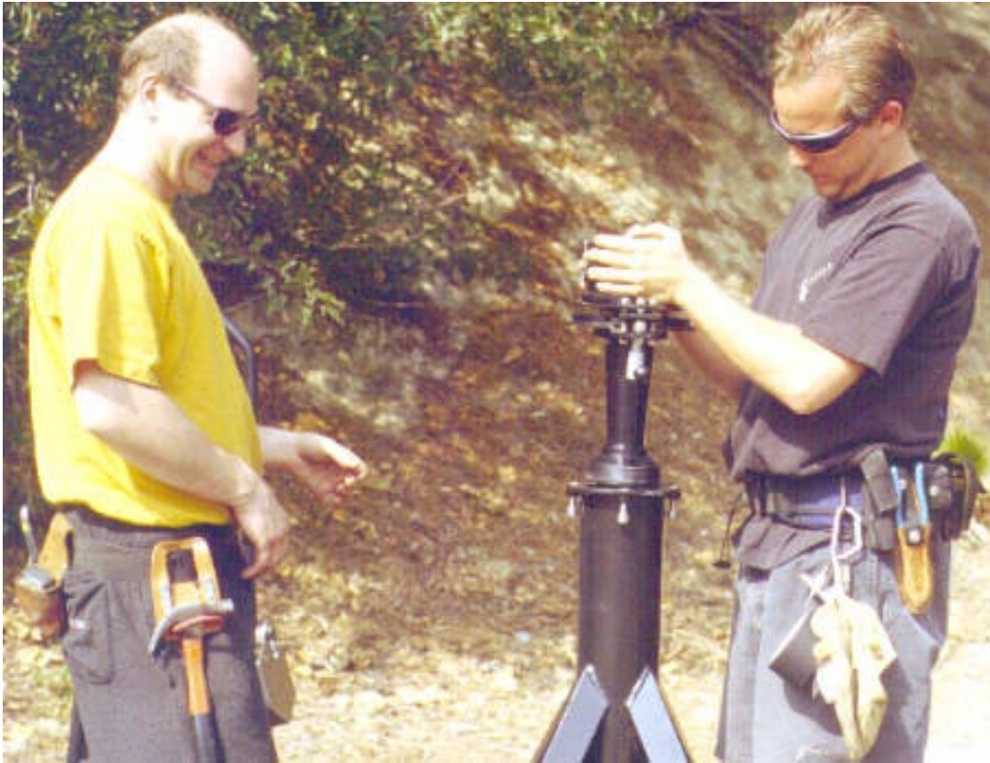
Mode 1 - Operating Platform - Step 9: Take main bearing (removed from inside of main post) and place inside mini post.
