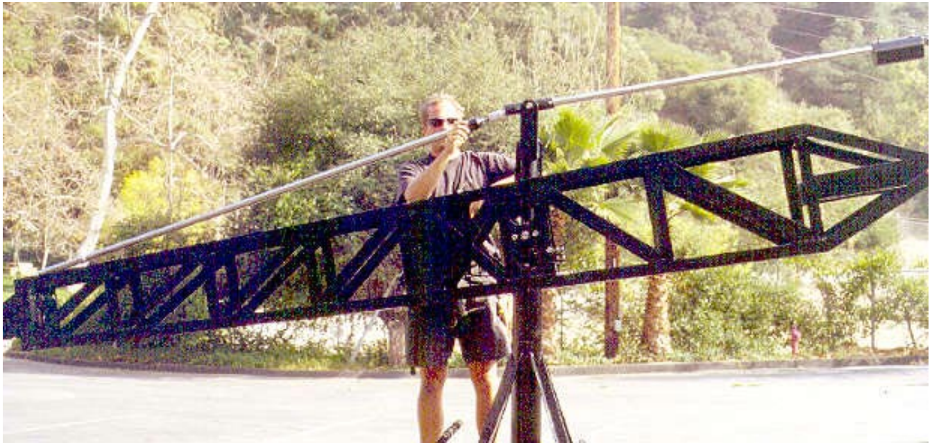
Mode 2 - Operating Platform - Step 9: Attach Rod # 2 to the front of the pylon (at post) with the quikpin.
