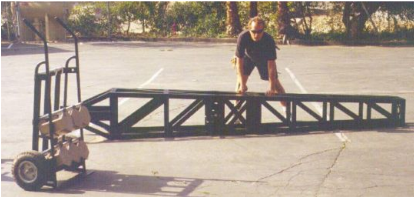
Mode 2 - Operating Platform - Step 2: Securely fasten 2 retaining bolts inside of Boom #1.
