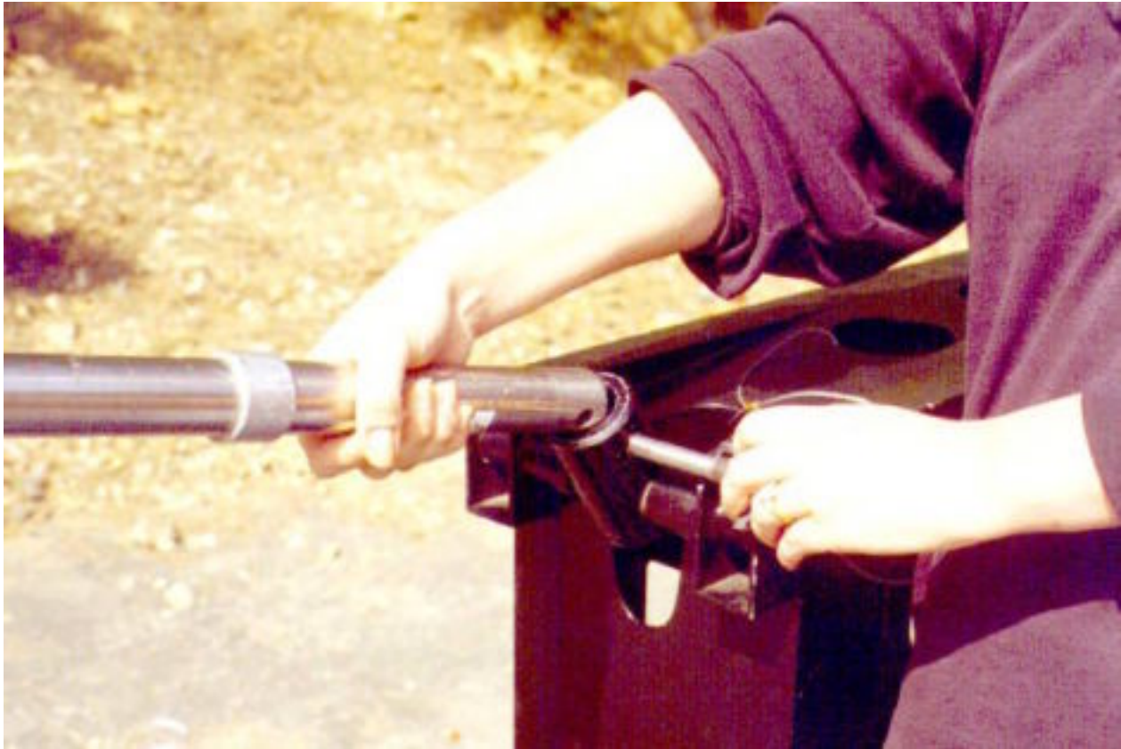
Mode 5 - Remote only - Step 21: Attach the front of Rod #4 to the remote head section with the quikpin.
