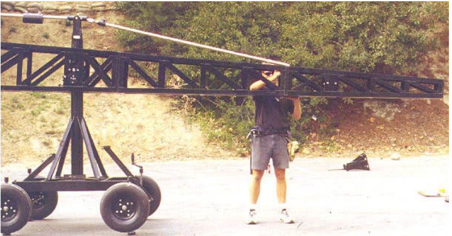
Mode 3 - Operation Platform - Step 11: Secure 2 retaining bolts found inside Boom #2.
