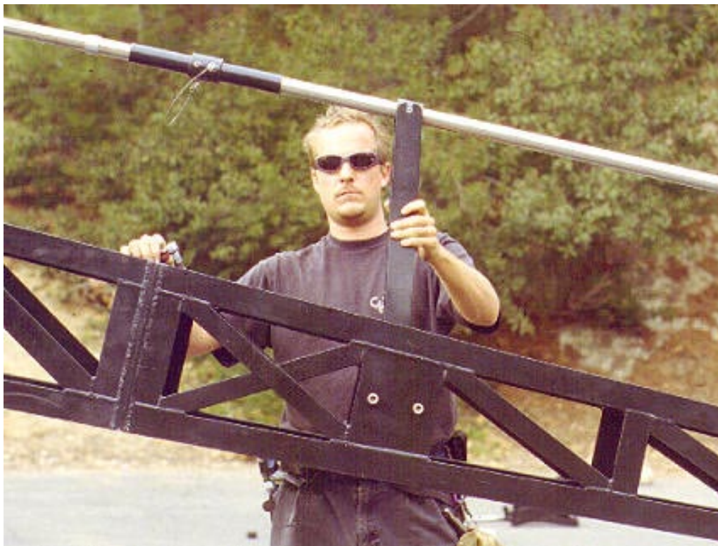
Mode 4 - Operating Platform - Step 14: Click Rod #3 into the top of the rod support bracket.
