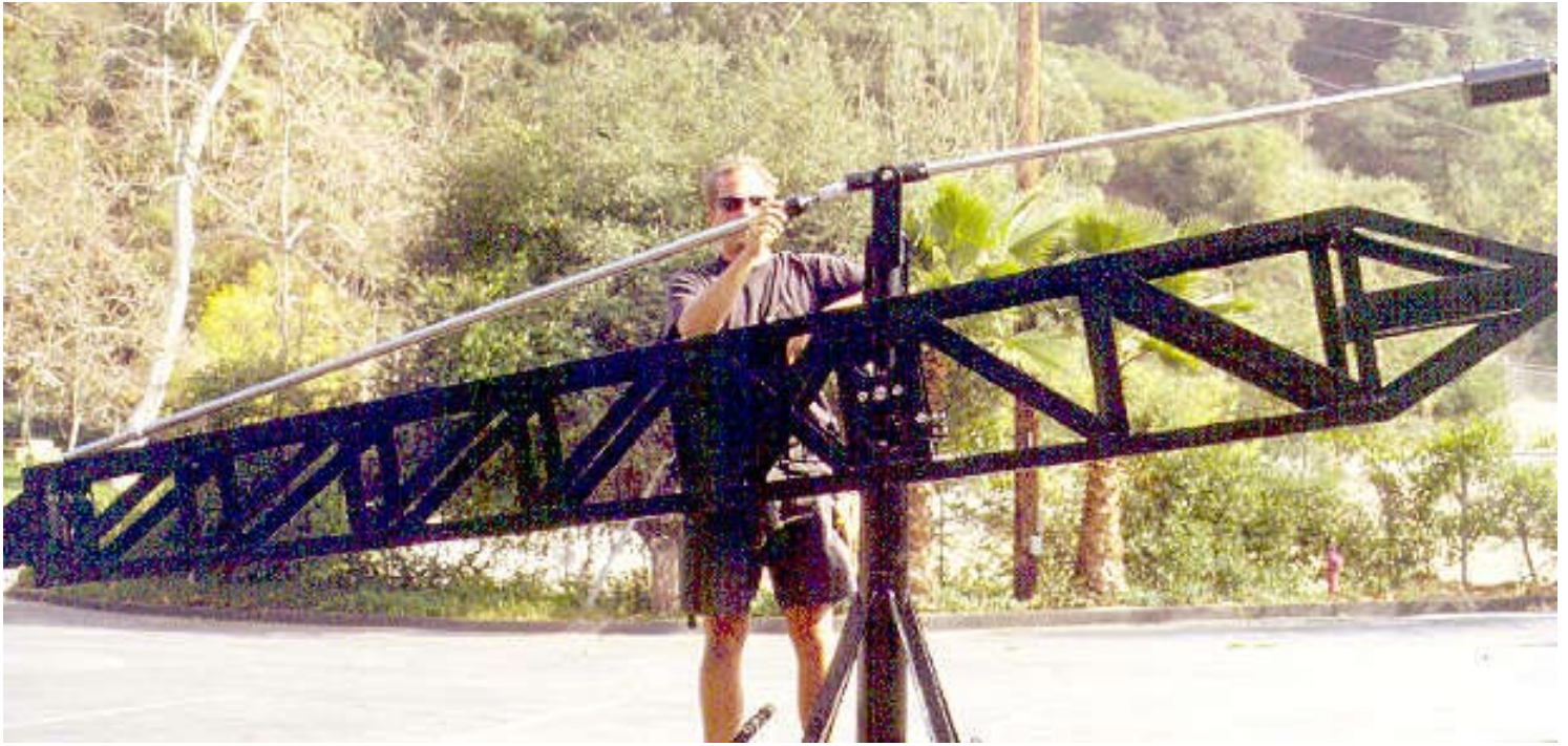
Mode 3 - Remote - Step 9: Attach Rod # 2 to the front of the pylon (at post) with the quikpin.
