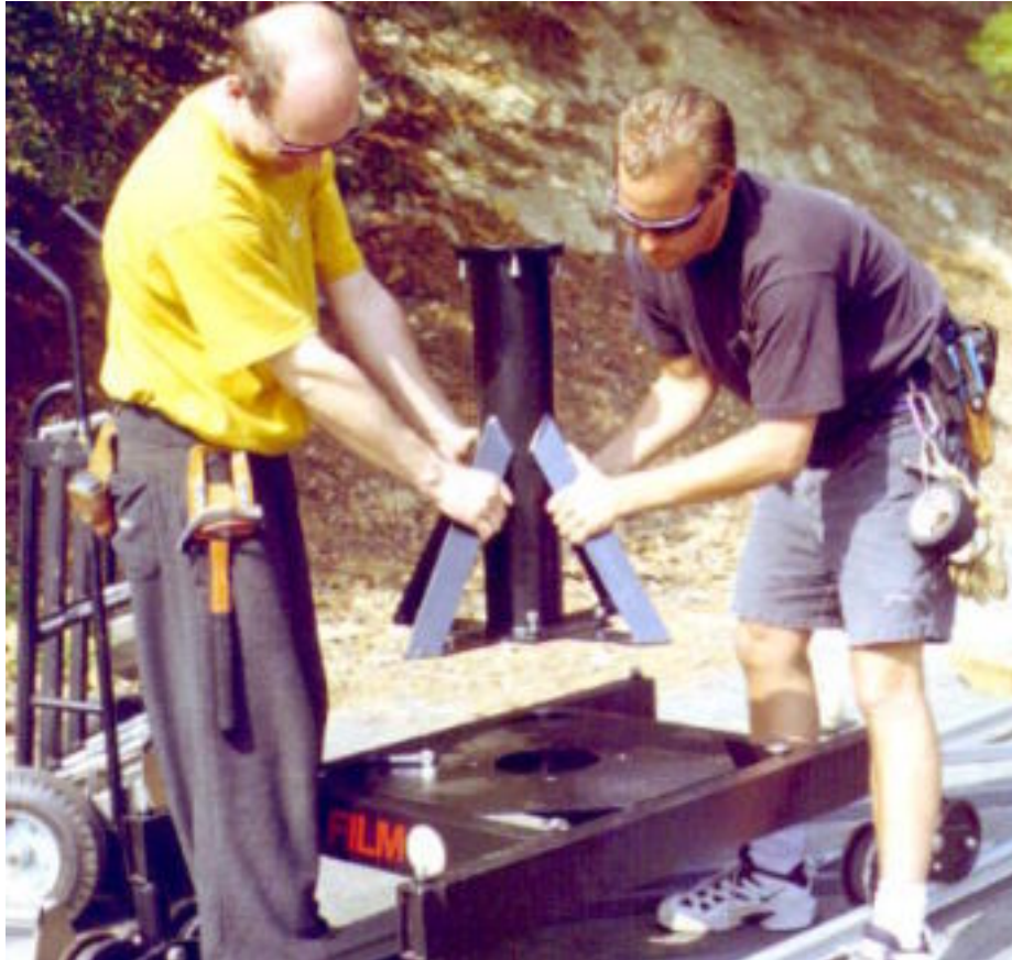
Mode 1 - Operating Platform - Step 8: Attach mini post to narrow crane base with 4 bolts.
