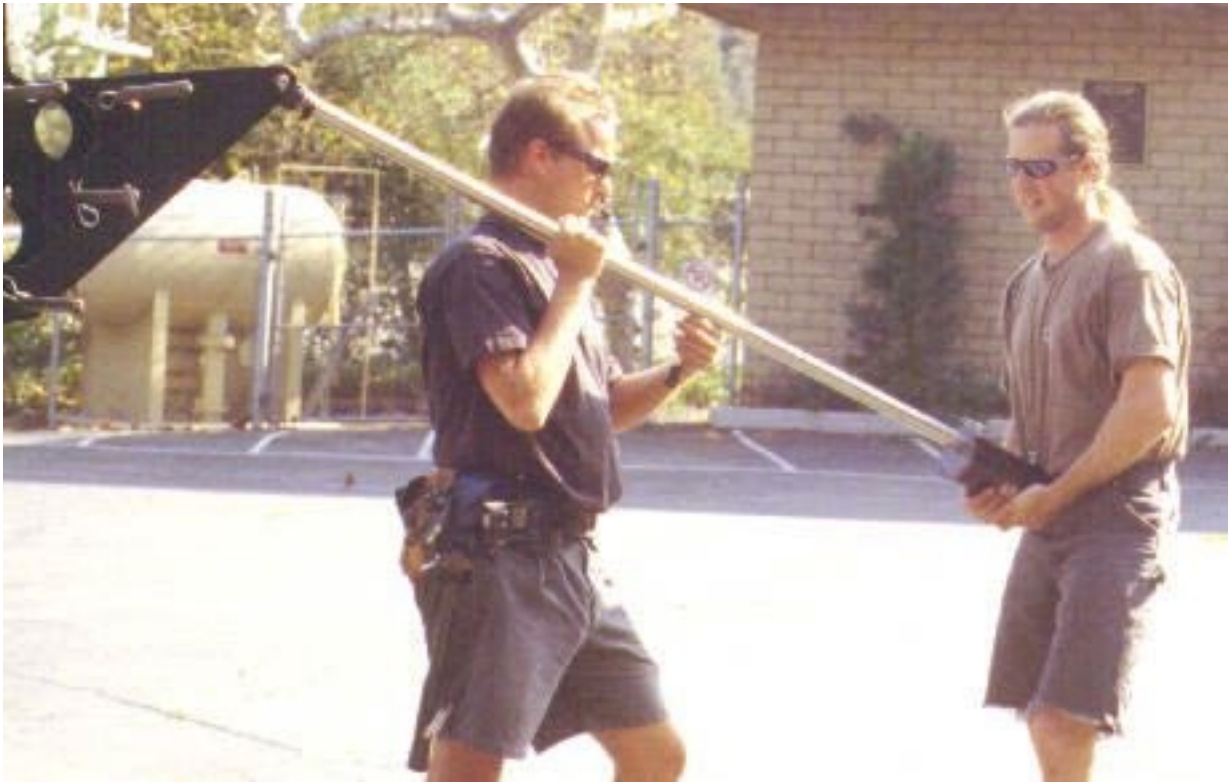
Mode 1+ - Remote Only - Step 15: Attach Rod A (mini rod) to weight box with the quikpin, then add the sliding trim weight. Now attach Rod A to the pylon on the other side with the quikpin.
