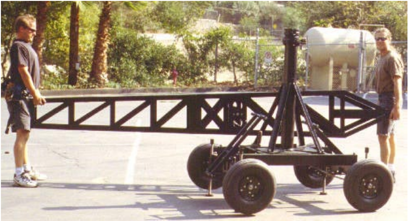
Mode 5 - Remote only - Step 3: Lift joined Boom #1 and Boom #2.
