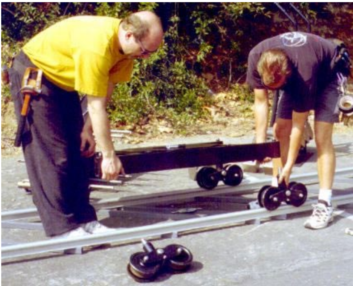
Mode 1+ - Remote Only - Step 6: Attach track wheels to narrow base where main crossbar attached before its removal.
