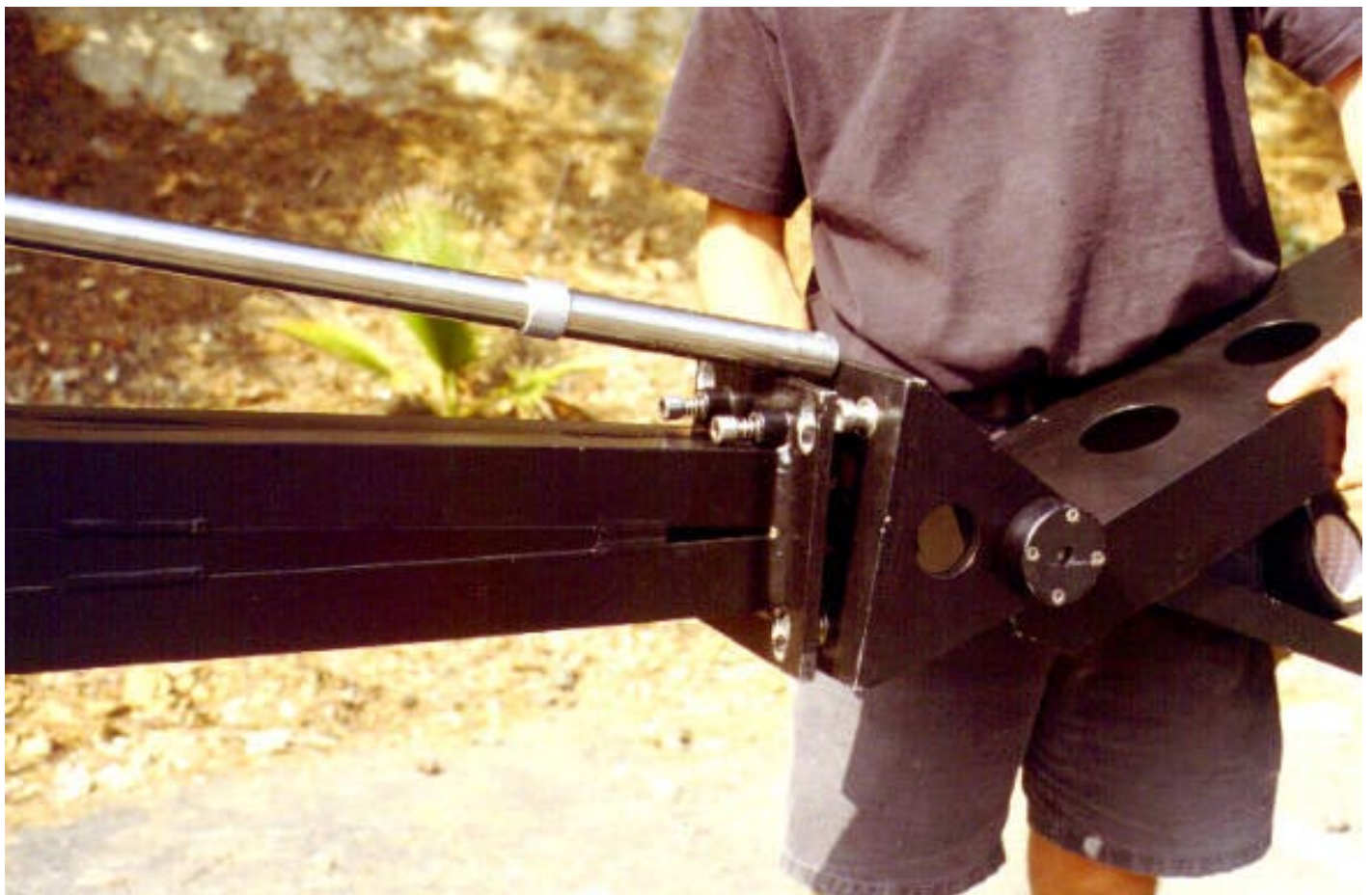
Mode 4 - Remote - Step 18: Secure remote head section with 2 retaining bolts found on the outside front of Boom #4.
