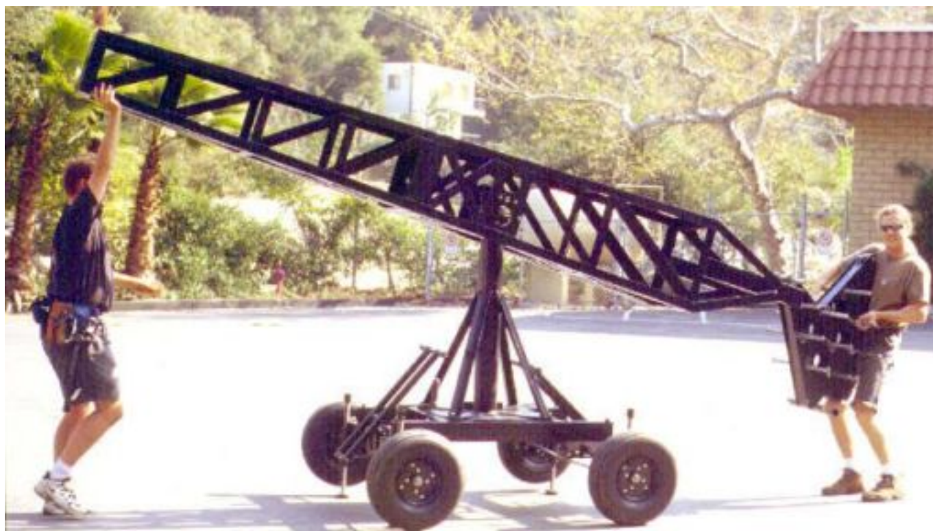
Mode 4 - Remote - Step 6: Add weight box into the slots on the back of Boom #1 and tighten the two retaining bolts (make sure that the weight box shaft isn't resting on the 2 retaining bolts).
