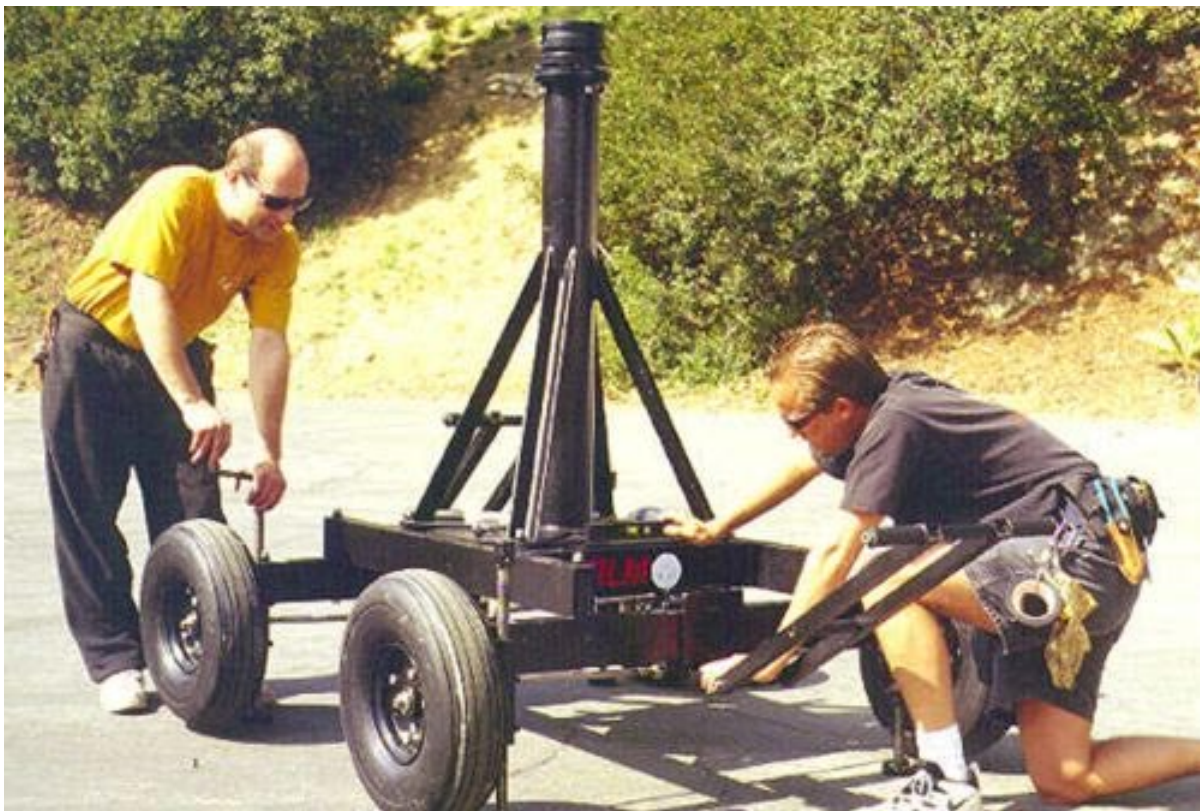
Leveling - Step 6: Level across base cranking corresponding jacks.
