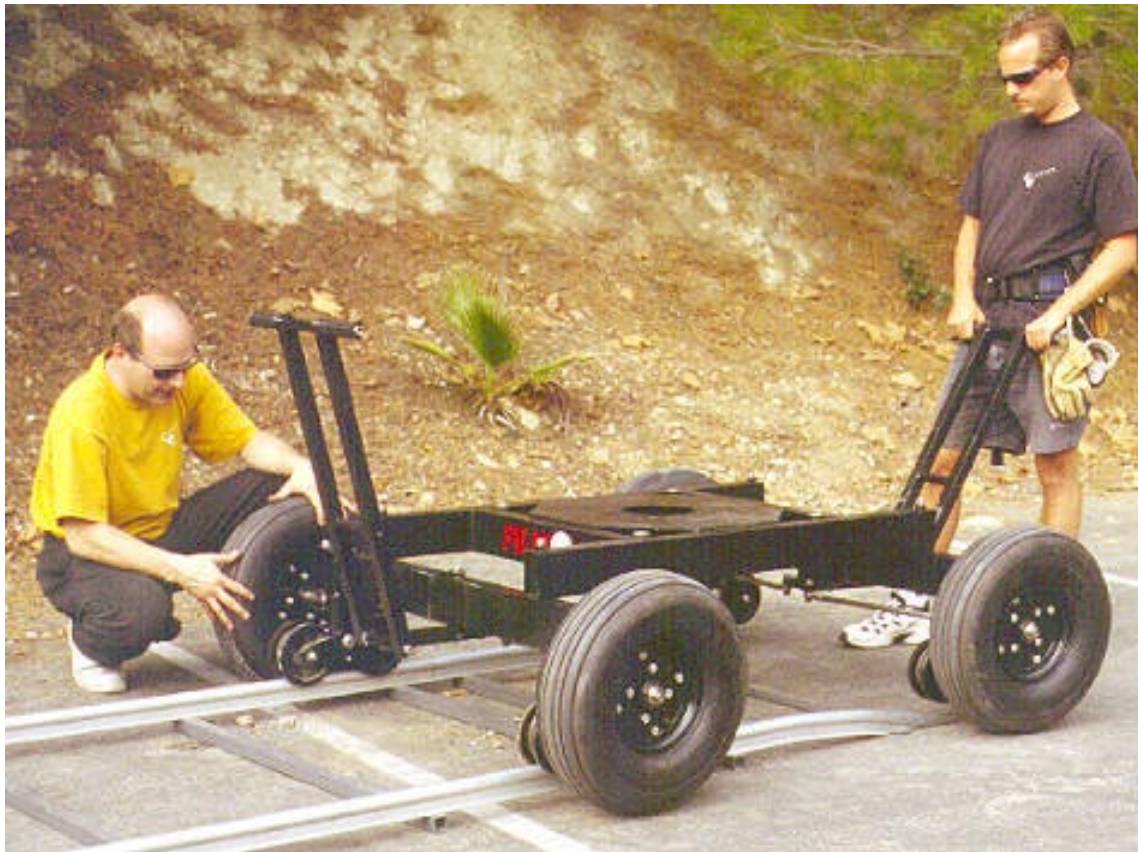
Dolly wide mode - Step 7: Place Dolly onto crane-width (3'3") track.
