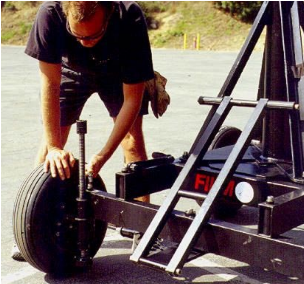
Leveling - Step 3: Tighten bolt snugly with wrench (don't overtighten!)
