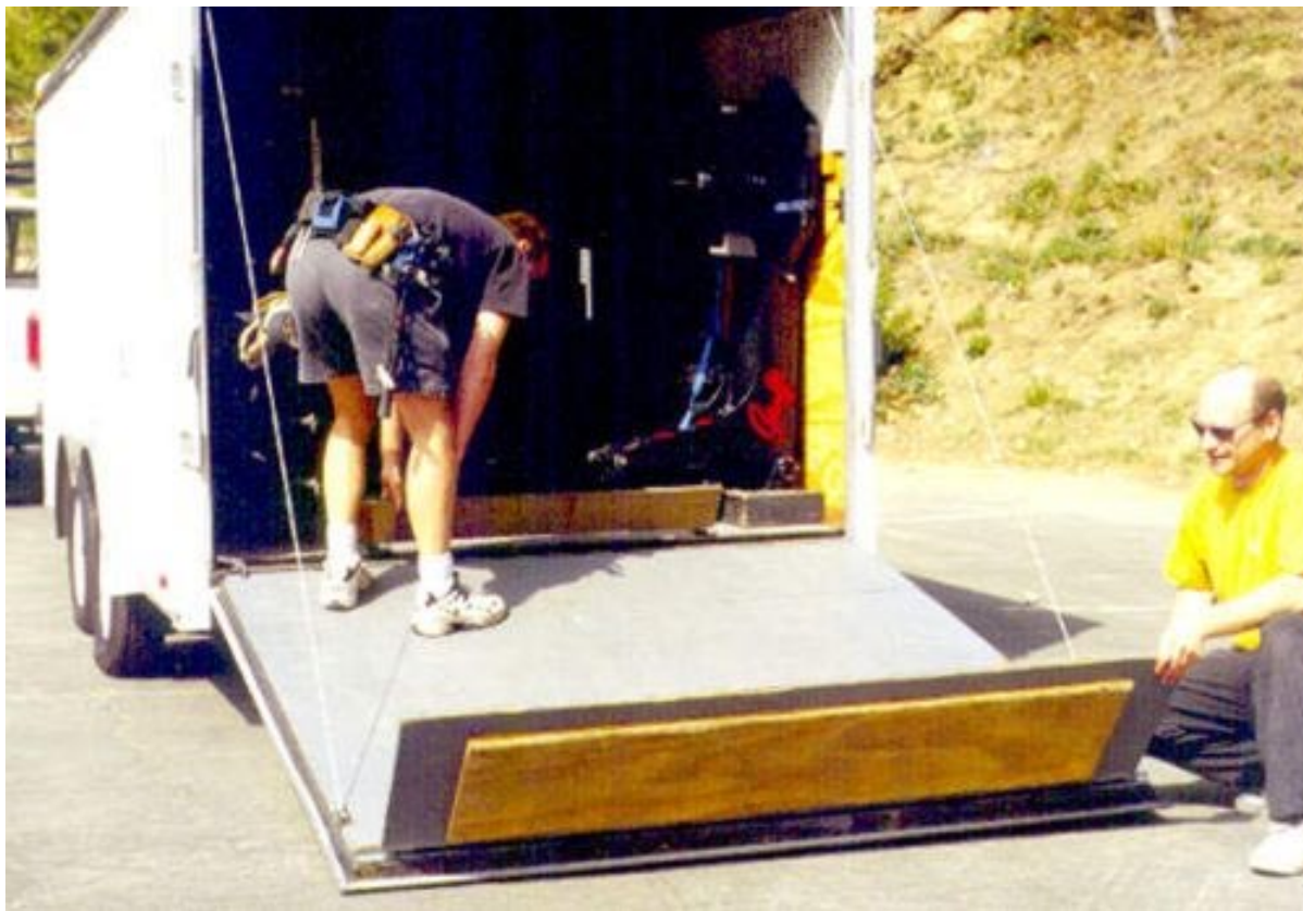
Trailer - Step 4: Fold down top and end ramps for a smooth exit!
