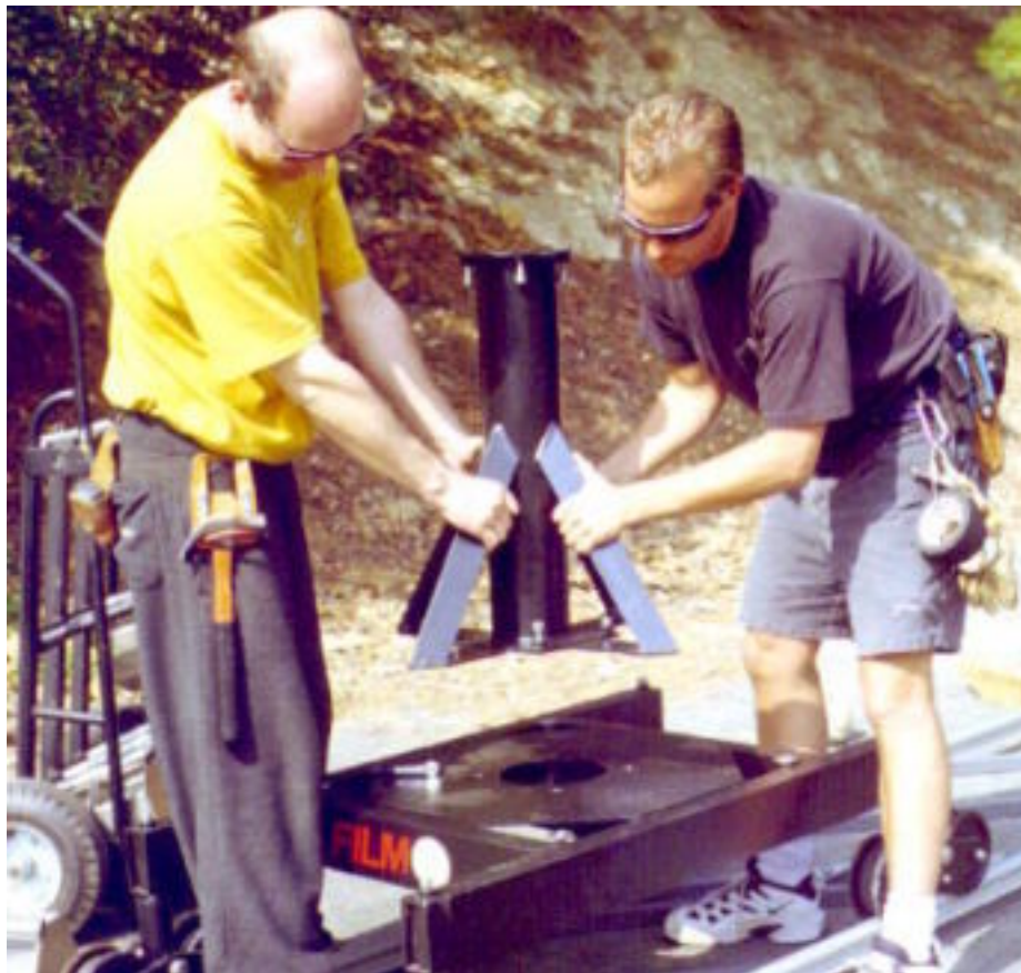
Mode 1 - Remote - Step 8: Attach mini post to narrow crane base with 4 bolts.
