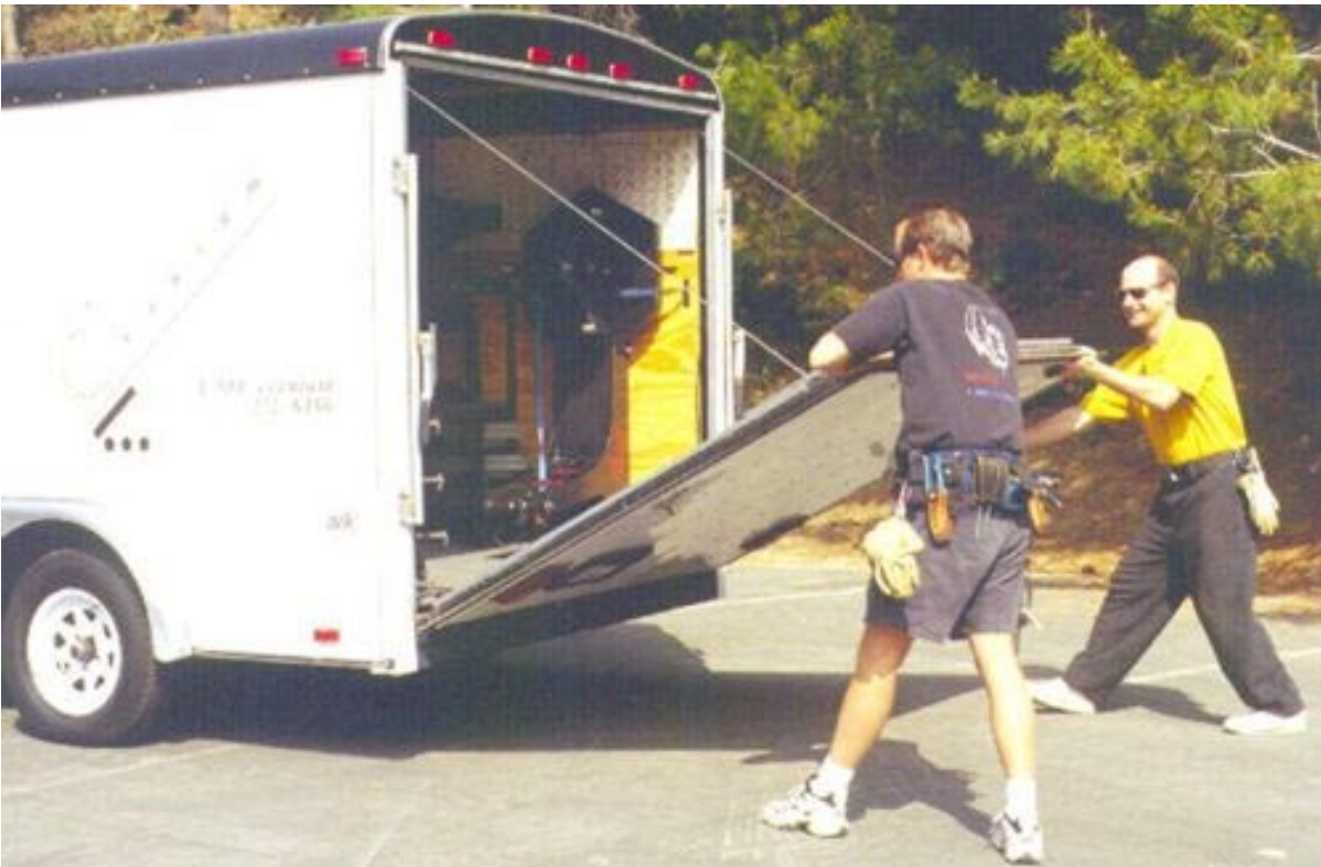
Trailer - Step 3: Open combo lock and fold down ramp (always leave at least 15 feet of space behind trailer so you can safely remove crane and contents!)
