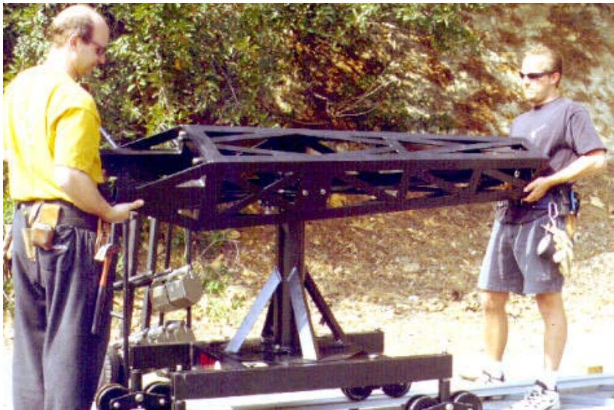
Mode 1 - Remote - Step 12: Place Boom #3 with mini bucket attachment onto mini post making sure to angle Boom #3 so it fits over the mini post- place it onto the horizontal main shaft inside Boom #3.
