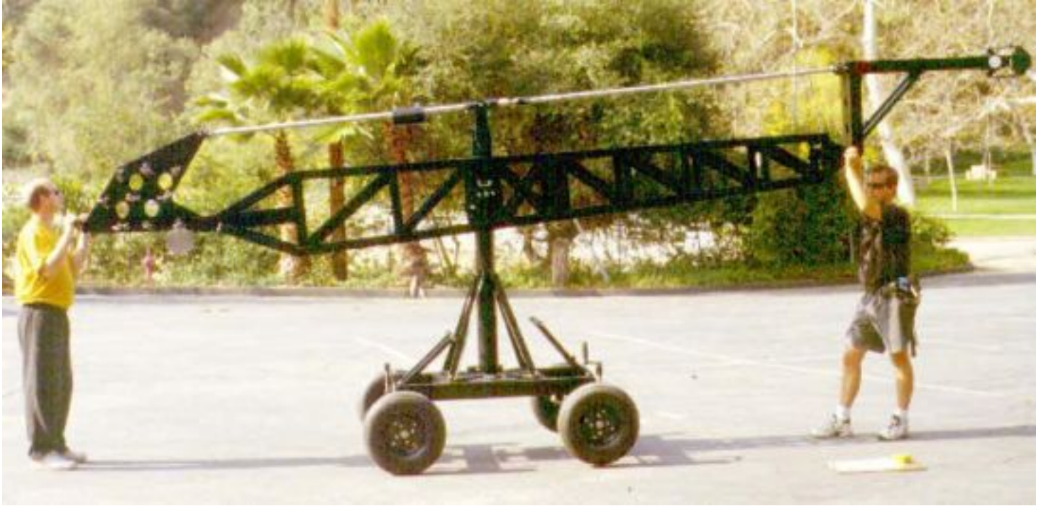
Mode 2 - Remote - Step 13: Finished Mode 2 remote (always keep the arm in balance as you build crane in any mode). End of steps.
