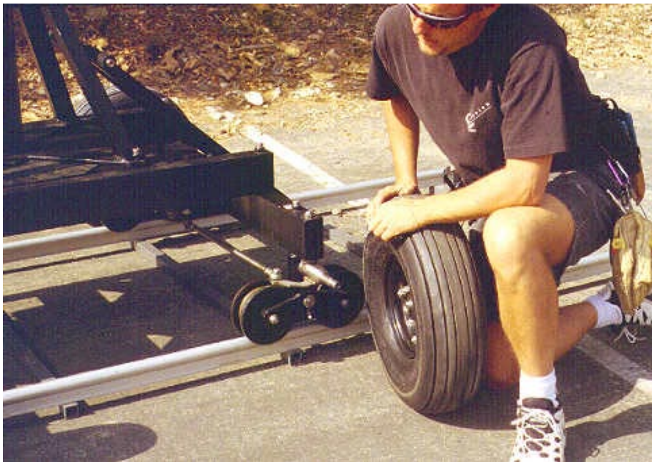
Dolly wide mode - Step 9: Remove Ruff wheel so it can't interfere with wedges under track. (End of steps)
