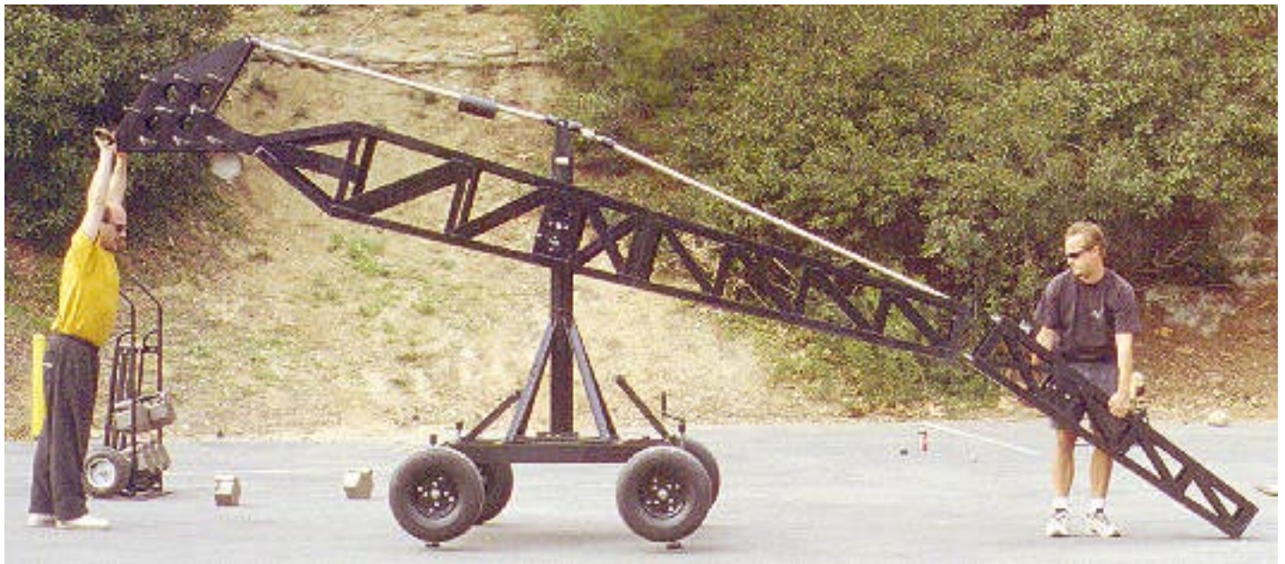
Mode 3 - Remote - Step 10: Attach Boom #3 to the front of Boom #2.
