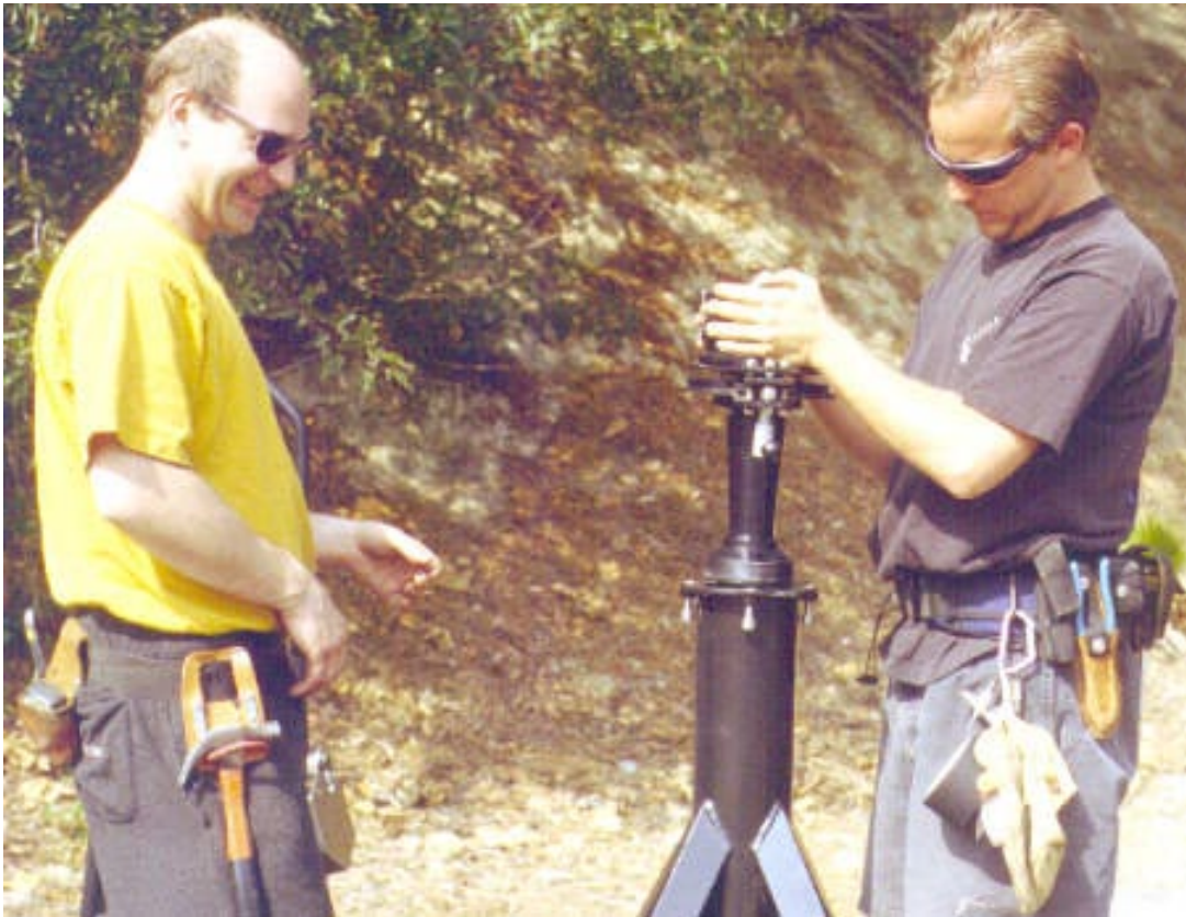
Mode 1 - Remote - Step 9: Take main bearing (removed from inside of main post) and place inside mini post.
