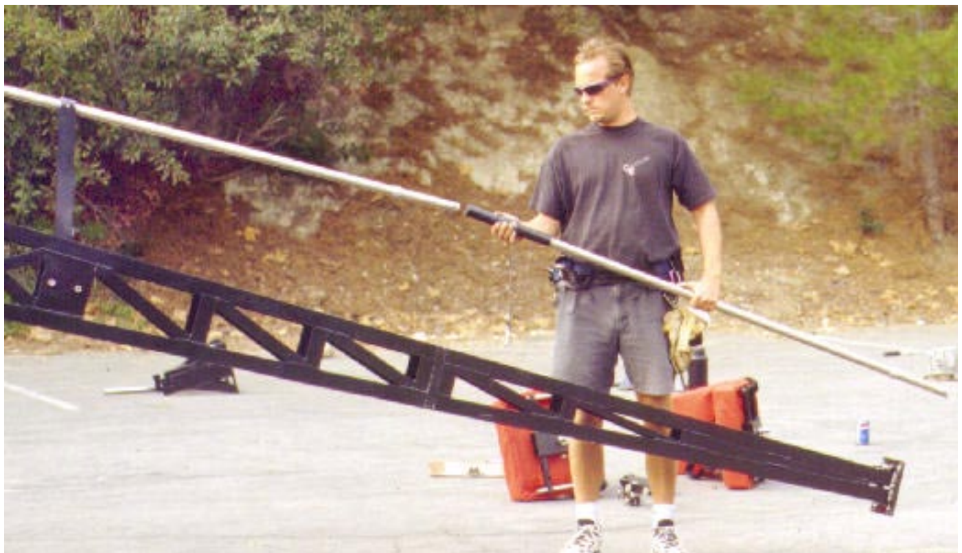
Mode 4 - Remote - Step 16: Attach Rod #4 to the front of Rod #3 with the quikpin.
