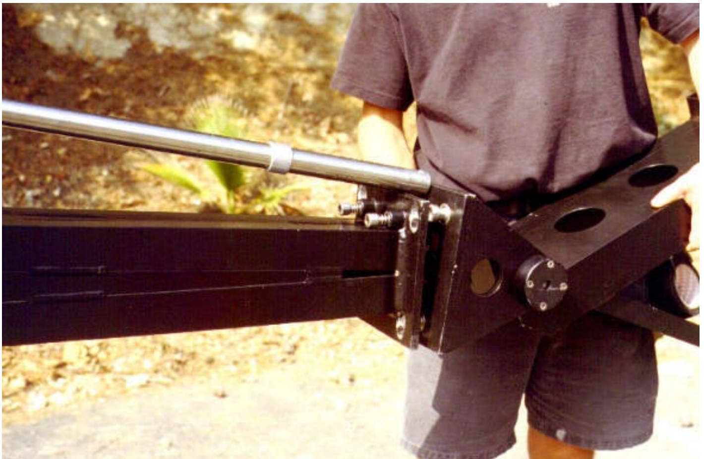
Mode 2 - Operating Platform - Step 10: Attach the Operating platform to the front of Boom #2 and secure it with the 2 retaining bolts on the inside of Boom #2.
