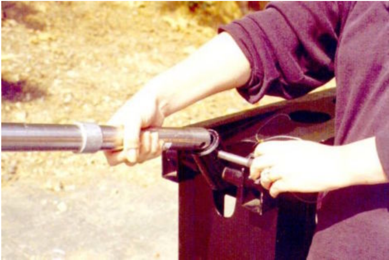
Mode 1+ - Remote Only - Step 19: Add Quick pin to remote nose section.
