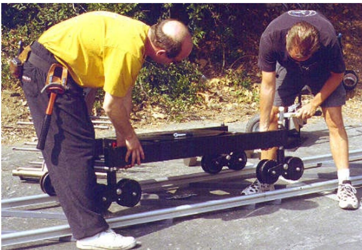
Dolly narrow mode - Step 8: To disassemble, reverse steps- unthread track wheel bolt several turns (easier when weight is on dolly) and lift base. Tap bolt with plastic mallet until track wheel disengages from base. Unthread bolt the rest of the way by hand.
