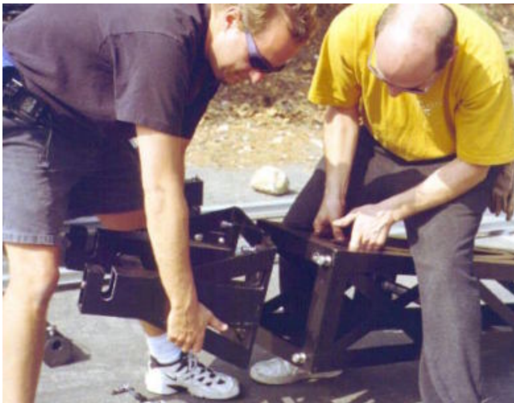
Mode 1 - Operating Platform - Step 11: Attach mini bucket to the back of Boom #3 with 2 retaining bolts on mini bucket.
