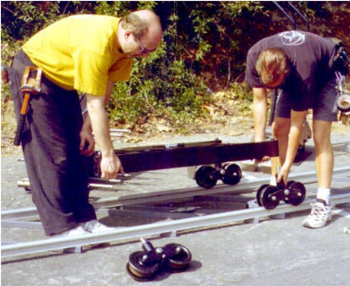
Dolly narrow mode - Step 9: Attach track wheels to crane base where main crossbar cones fit into main base. End of steps.
