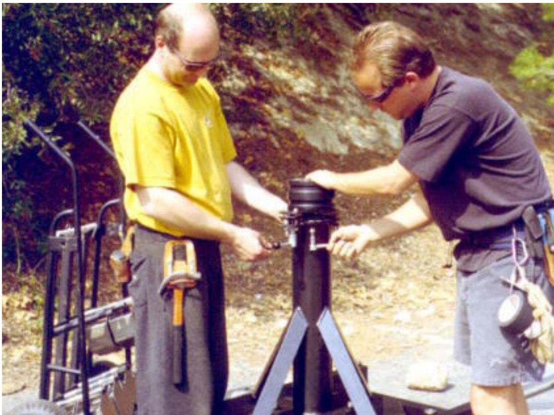
Mode 1 - Operating Platform - Step 10: Tighten 4 bolts that hold bearing into mini post.
