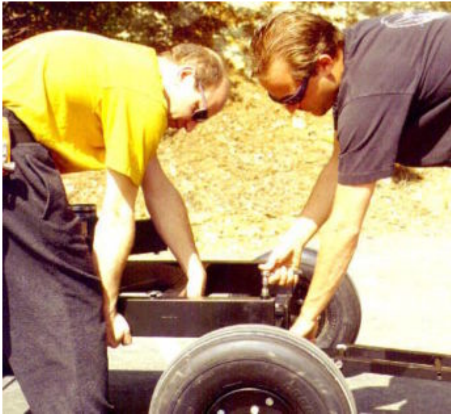
Mode 1 - Operating Platform - Step 1: Unbolt main crossbar from crane base.
