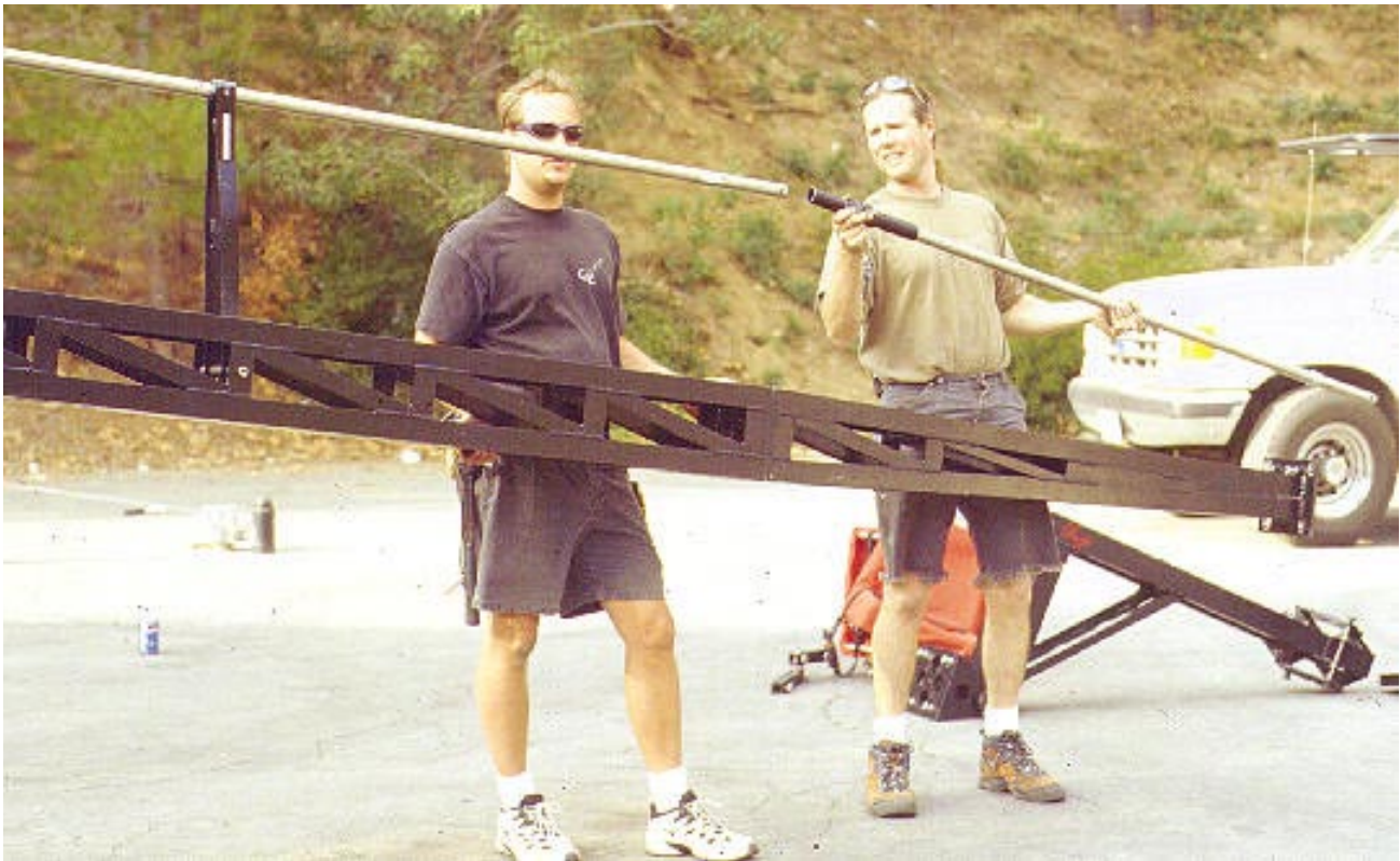
Mode 5 - Remote only - Step 19: Attach Rod #4 to the front of the Remote rod with the quickpin.
