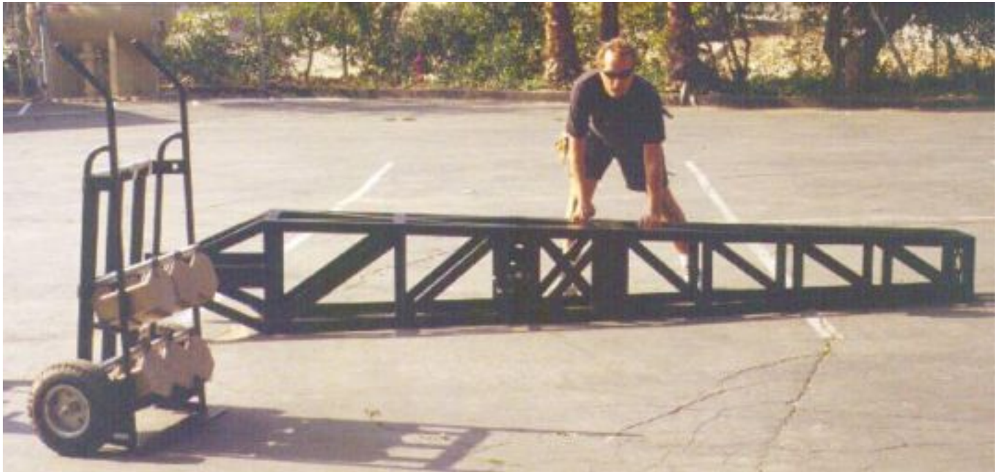
Mode 2 - Remote - Step 2: Securely fasten 2 retaining bolts inside of Boom #1.
