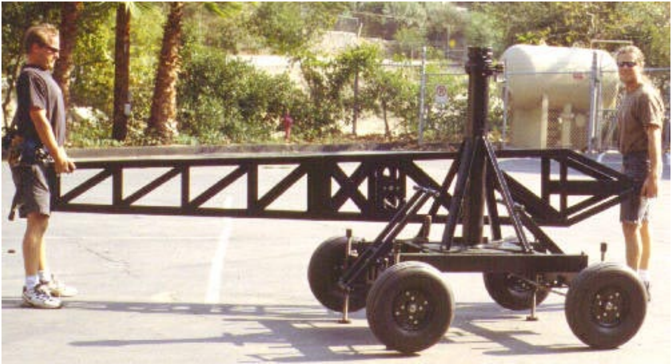
Mode 3 - Remote - Step 3: Lift joined Boom #1 and Boom #2.
