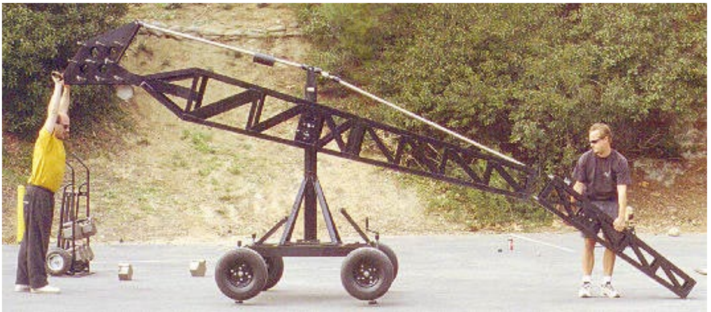
Mode 5 - Remote only - Step 10: Attach Boom #3 to the front of Boom #2.
