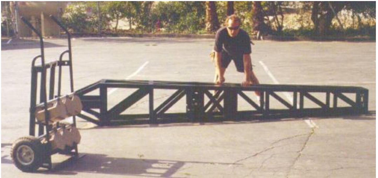
Mode 4 - Operating Platform - Step 2: Securely fasten 2 retaining bolts inside of Boom #1.
