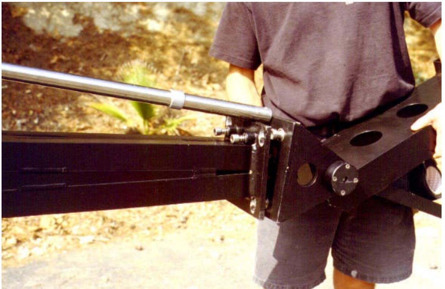
Mode 2 - Remote - Step 10: Attach remote head section.
