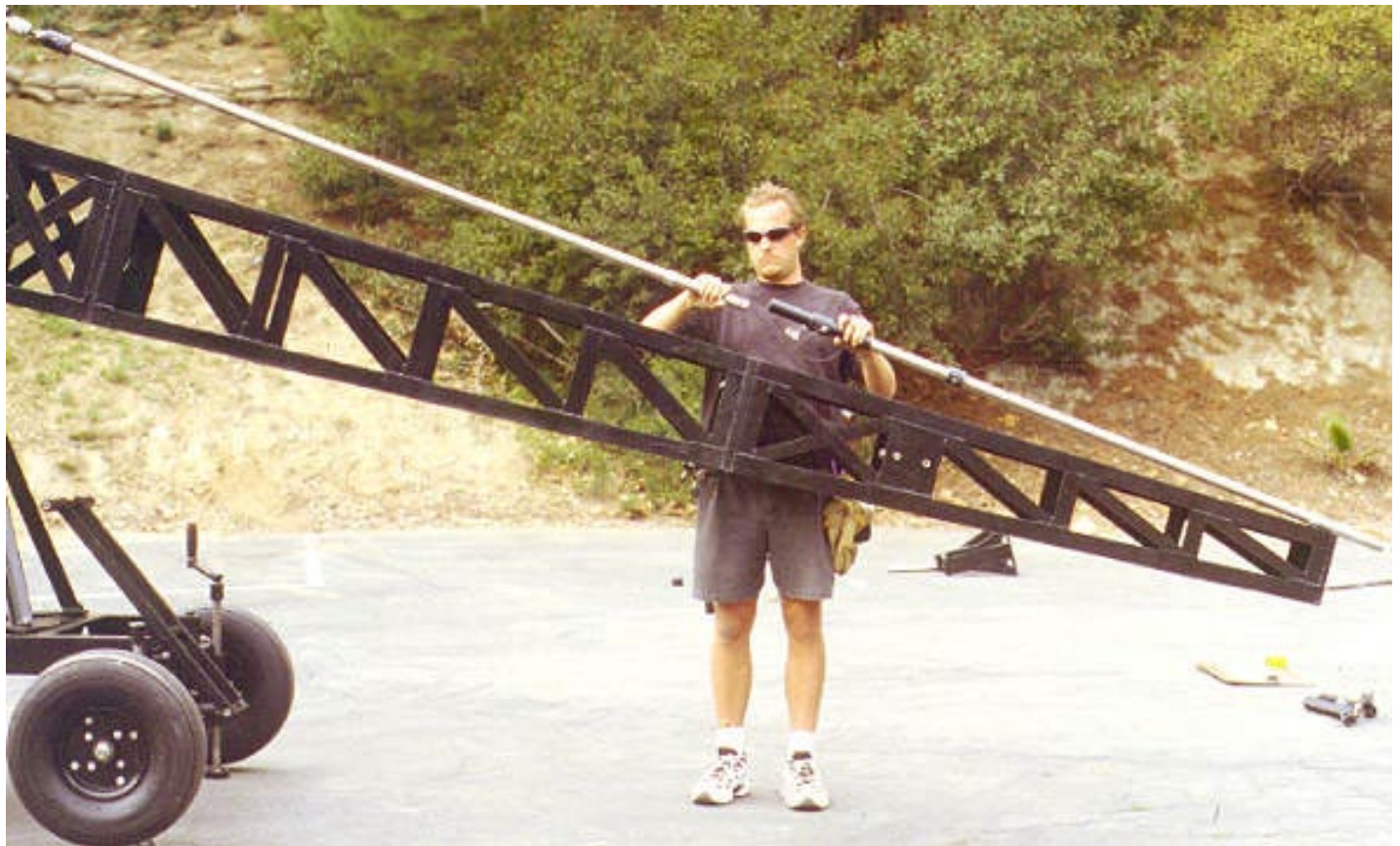
Mode 3 - Operation Platform - Step 12: Add Rod #3 to the front of Rod #2 and secure with the quikpin.
