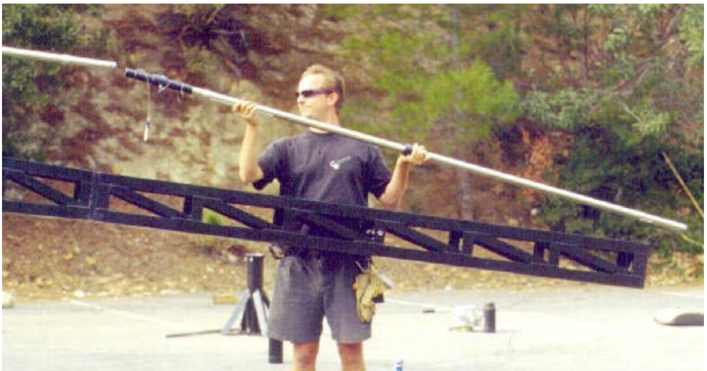
Mode 5 - Remote only - Step 16: Attach Remote rod to the front of Rod #3.
