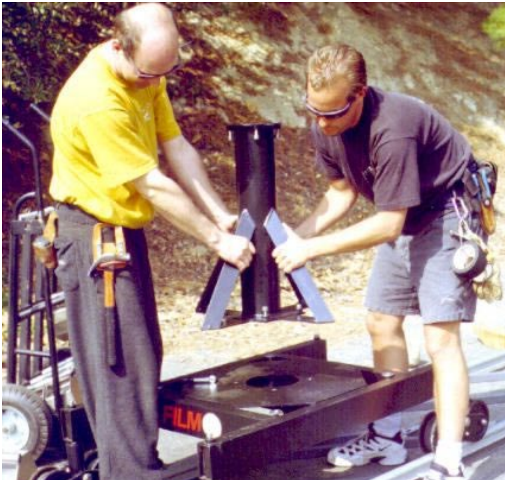
Mode 1+ - Remote Only - Step 8: Attach mini post to narrow crane base with 4 bolts.
