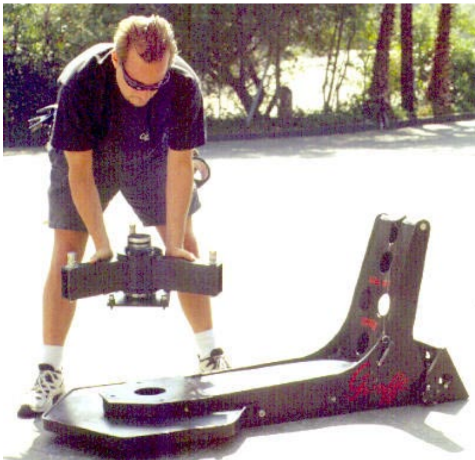
Dolly wide mode - Step 4: Remove swivel seat unit.
