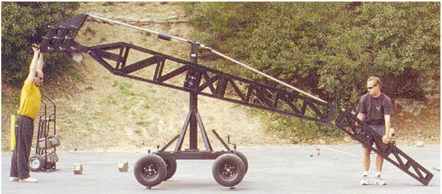
Mode 4 - Operating Platform - Step 10: Attach Boom #3 to the front of Boom #2.
