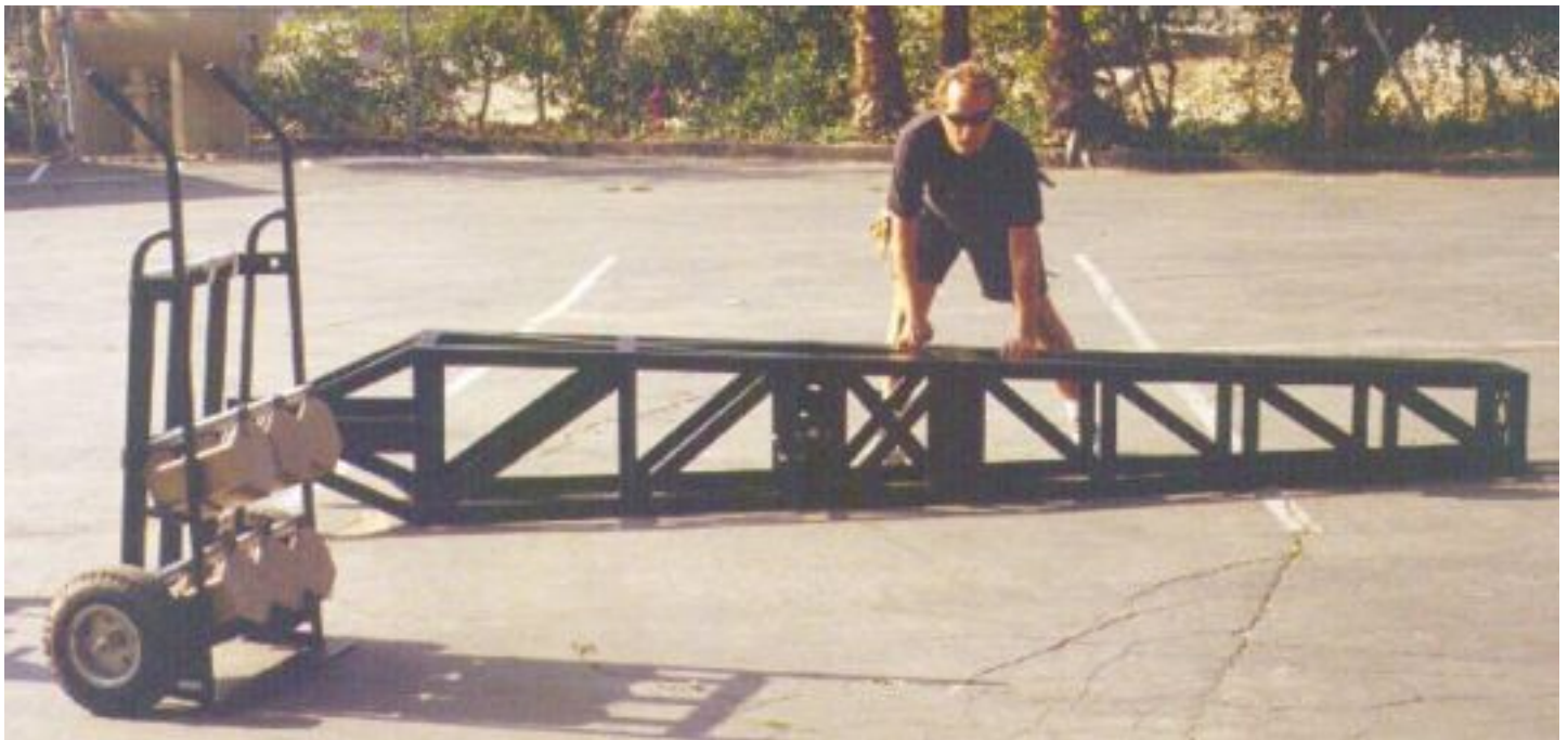
Mode 3 - Operation Platform - Step 2: Securely fasten 2 retaining bolts inside of Boom #1.
