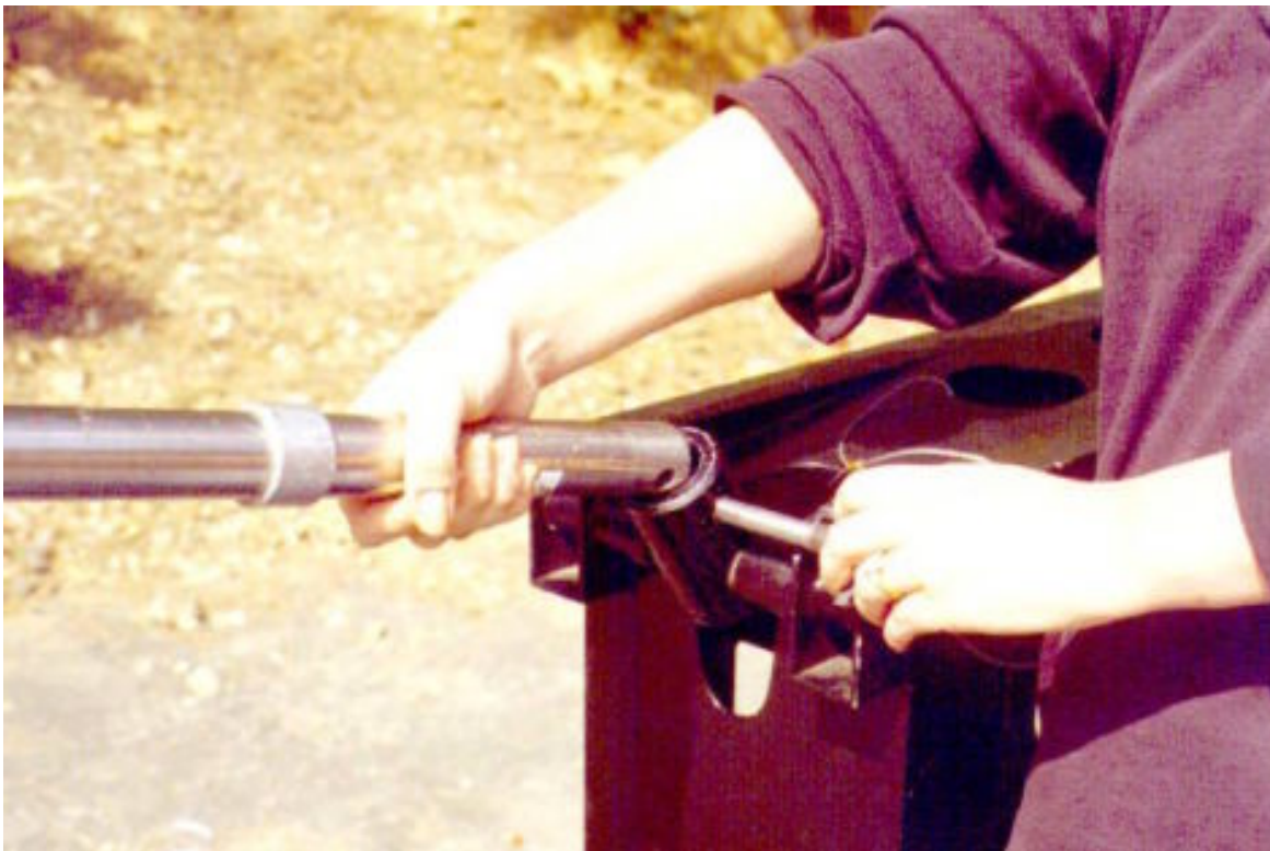
Mode 2 - Operating Platform - Step 12: Attach Rod #2 to the Operating platform with the quik pin.
