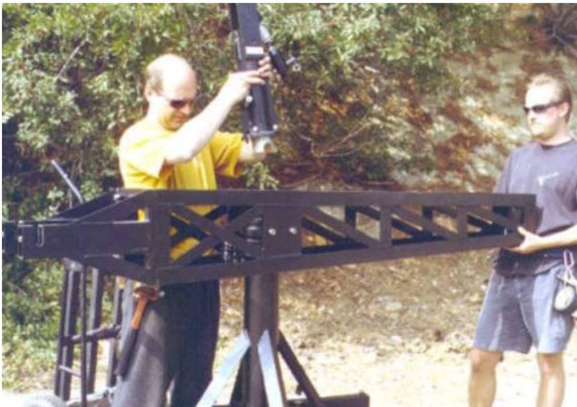
Mode 1+ - Remote Only - Step 13: Attach Pylon assembly to mini post with 4 bolts in pylon. Horizontal shaft is then trapped into place. (Be sure that threaded end of the pylon rod section is facing towards the front- so you can level operating platform later!)
