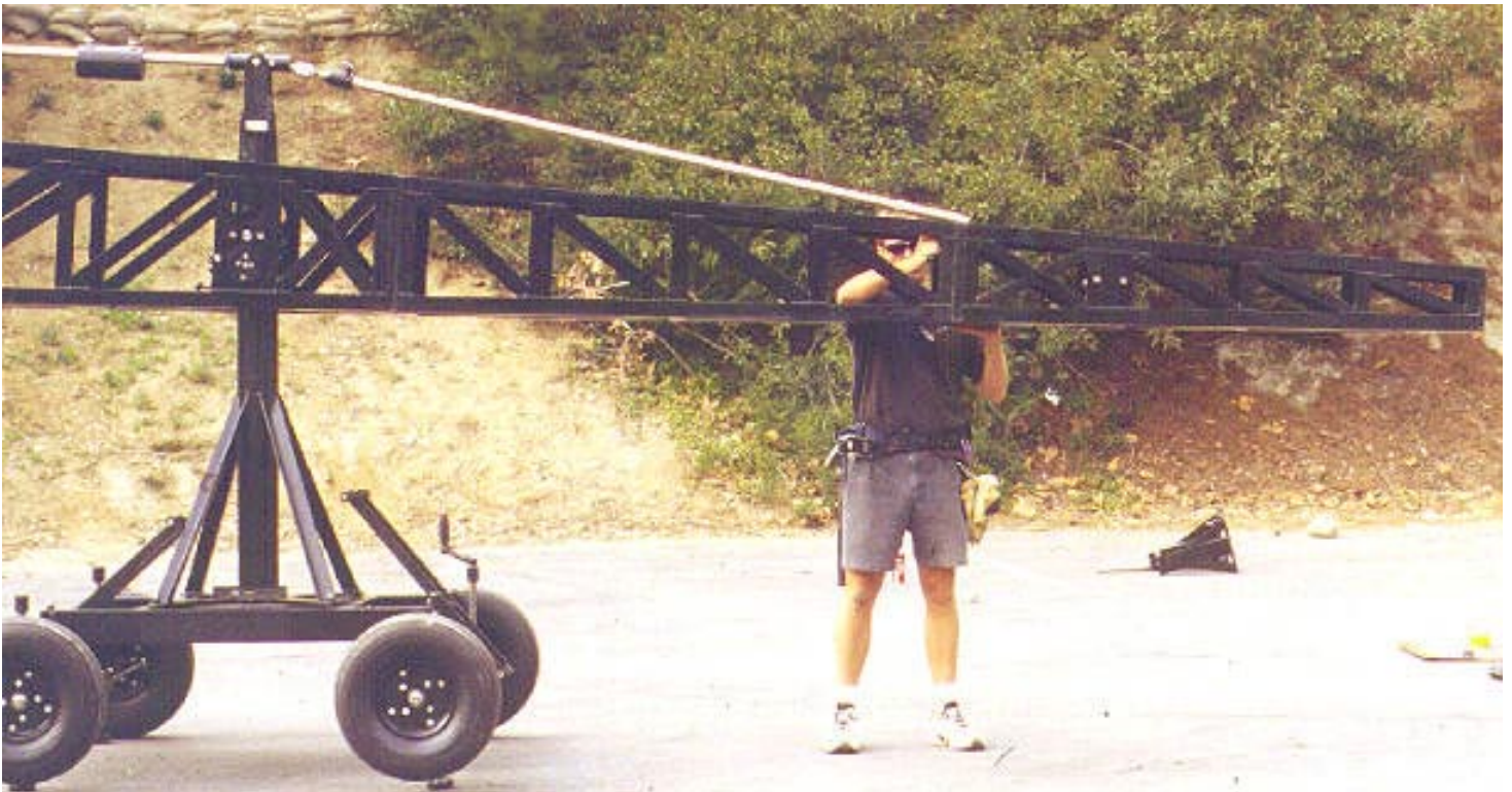
Mode 4 - Operating Platform - Step 11: Secure 2 retaining bolts found inside Boom #2.
