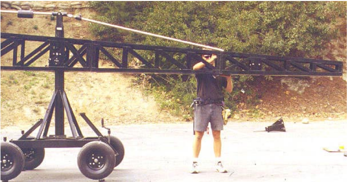
Mode 4 - Remote - Step 11: Secure 2 retaining bolts found inside Boom #2.
