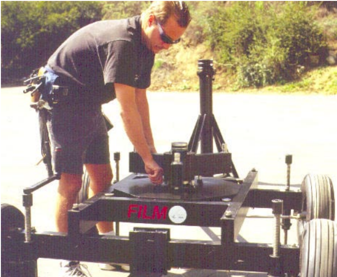
Dolly narrow mode - Step 5: Place, then bolt swivel seat unit to the crane base.
