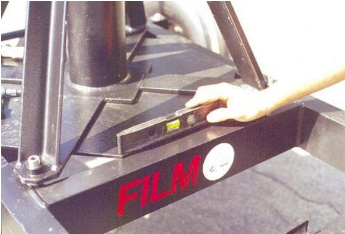
Leveling - Step 7: close-up of crane base.
