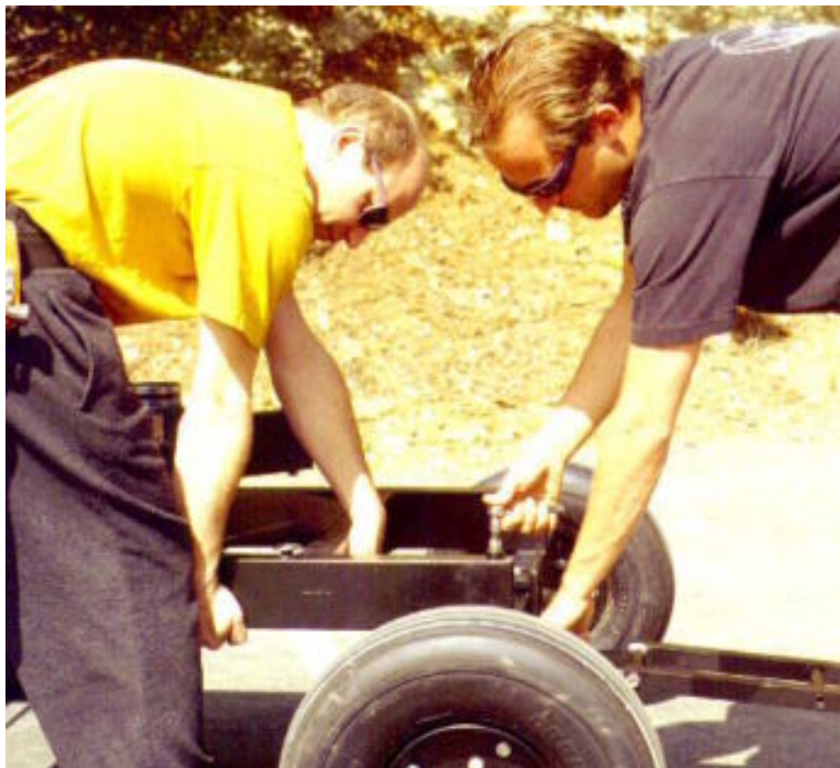
Dolly narrow mode - Step 6: Unbolt main crossbar (section that contains steering mechanism) from the crane base.
