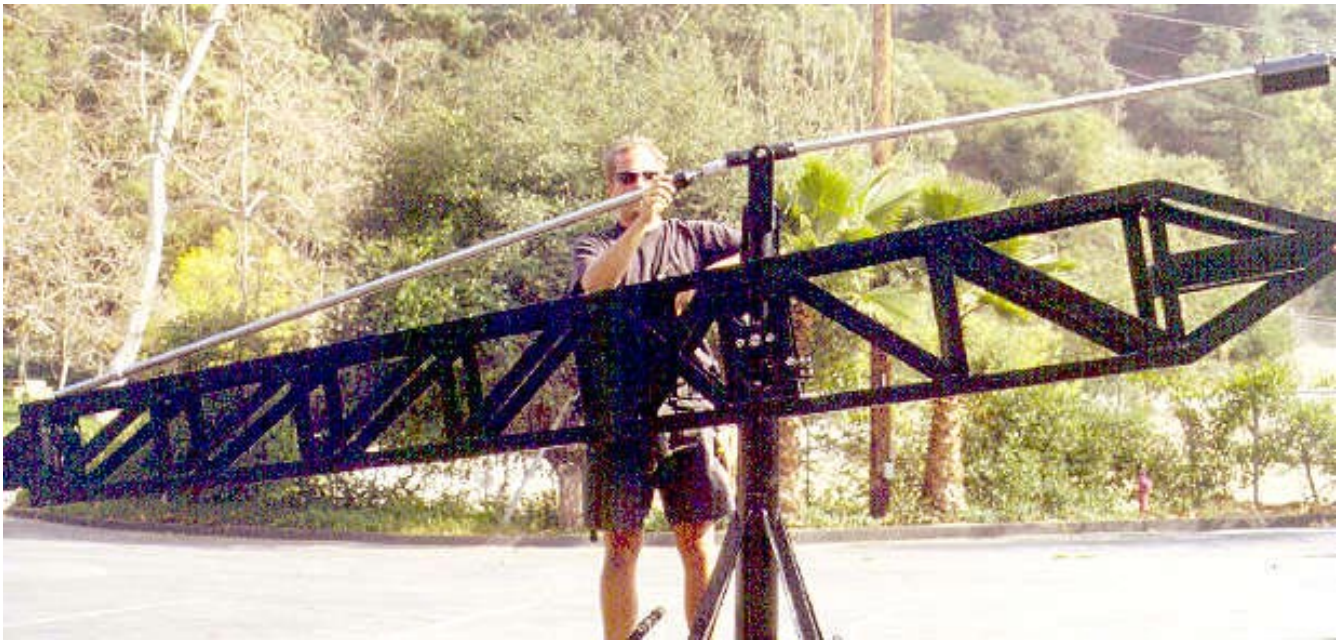
Mode 4 - Remote - Step 9: Attach Rod # 2 to the front of the pylon (at post) with the quikpin.
