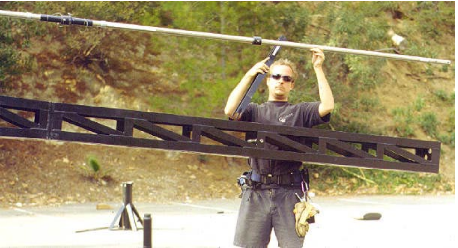
Mode 5 - Remote only - Step 17: Attach 2nd rod support bracket to the horizontal shaft inside Remote Boom and to the corresponding upper attachment on the Remote rod.
