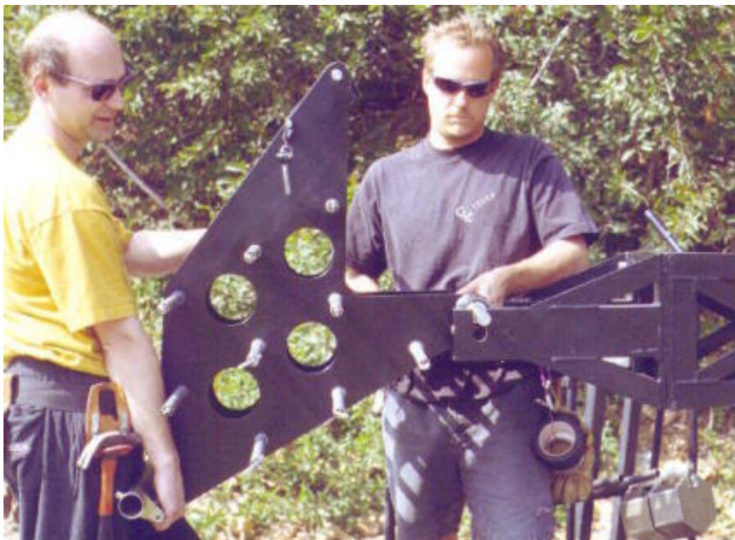
Mode 1 - Remote - Step 14: Place weight box into slots on mini bucket and tighten the two retaining bolts (don't overtighten!)
