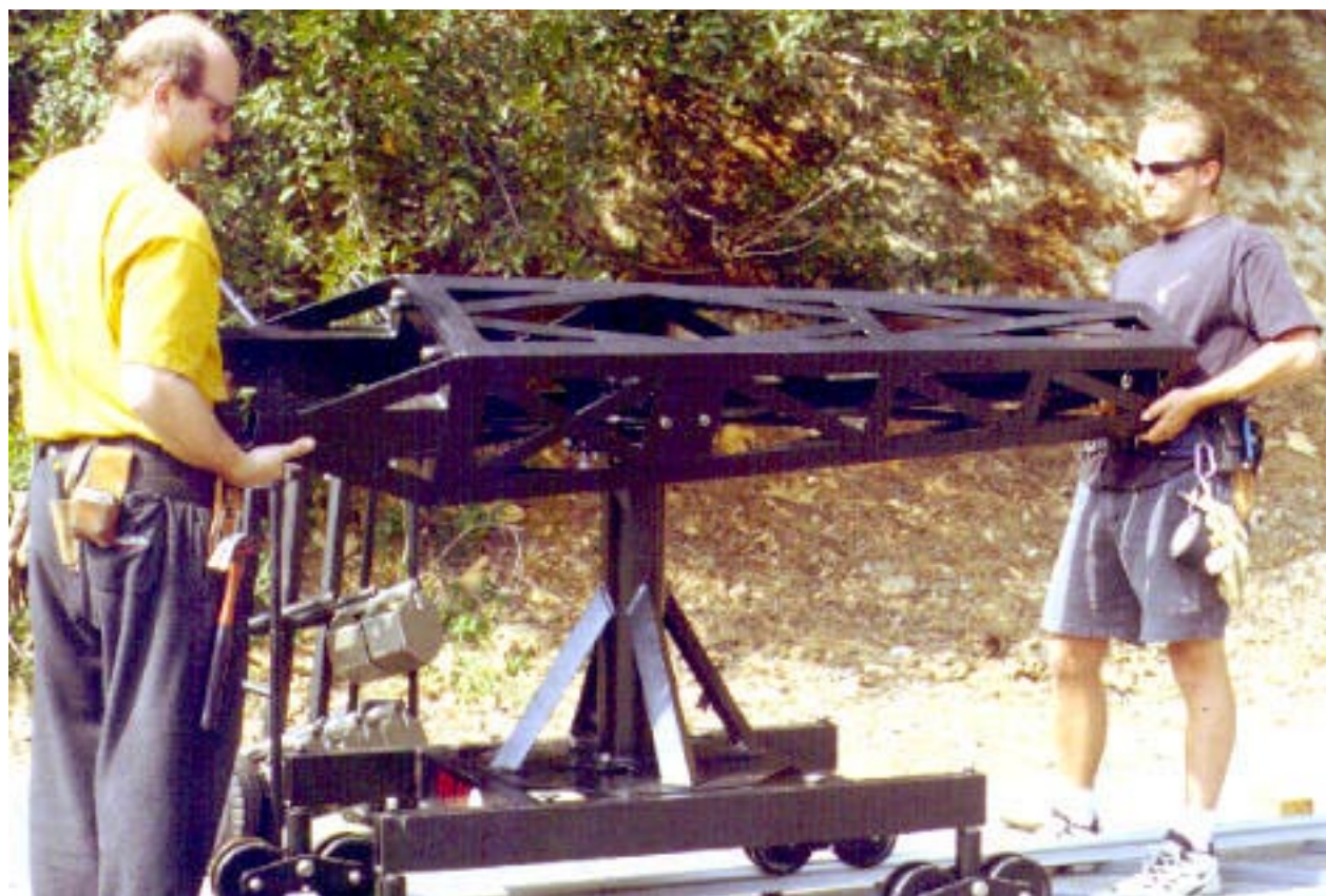
Mode 1 - Operating Platform - Step 12: Place Boom #3 with mini bucket attachment onto mini post making sure to angle Boom #3 so it fits over the mini post- place it onto the horizontal main shaft inside Boom #3.
