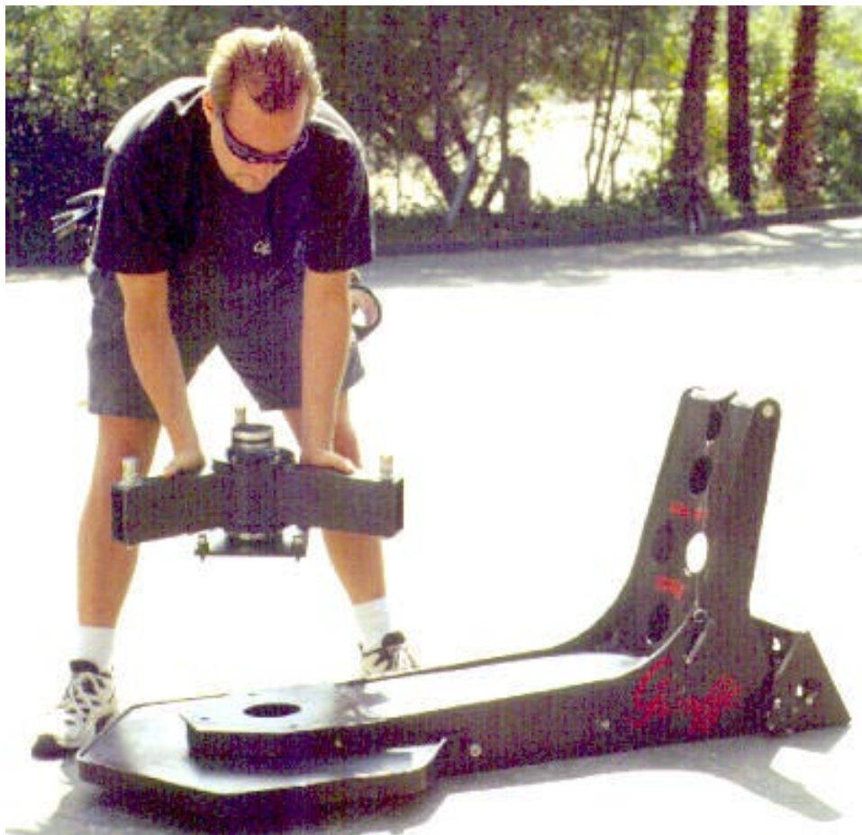
Dolly narrow mode - Step 4: Remove swivel seat unit.
