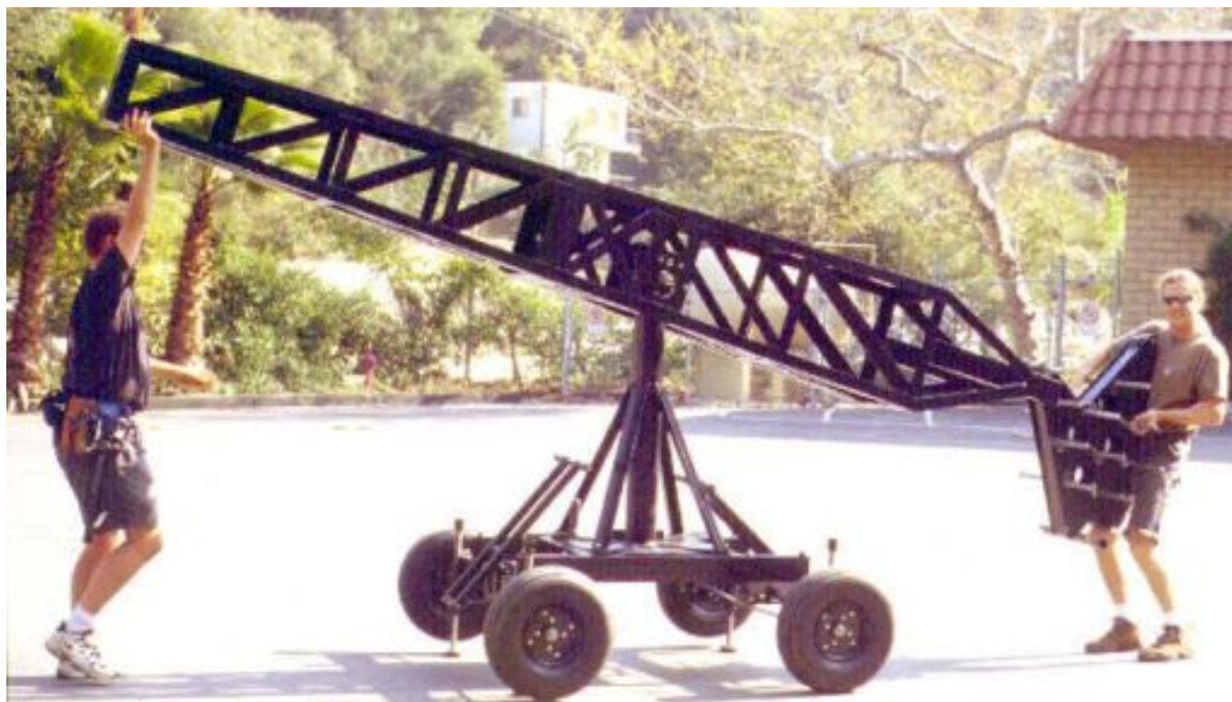
Mode 4 - Operating Platform - Step 6: Add weight box into the slots on the back of Boom #1 and tighten the two retaining bolts (make sure that the weight box shaft isn't resting on the 2 retaining bolts).
