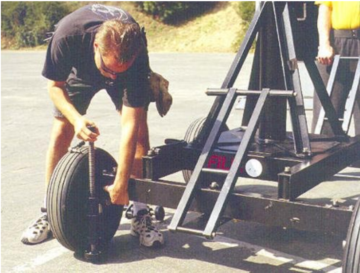
Leveling - Step 1: Fit levelling jack into main crossbar on crane base, just inside of Ruff wheel.
