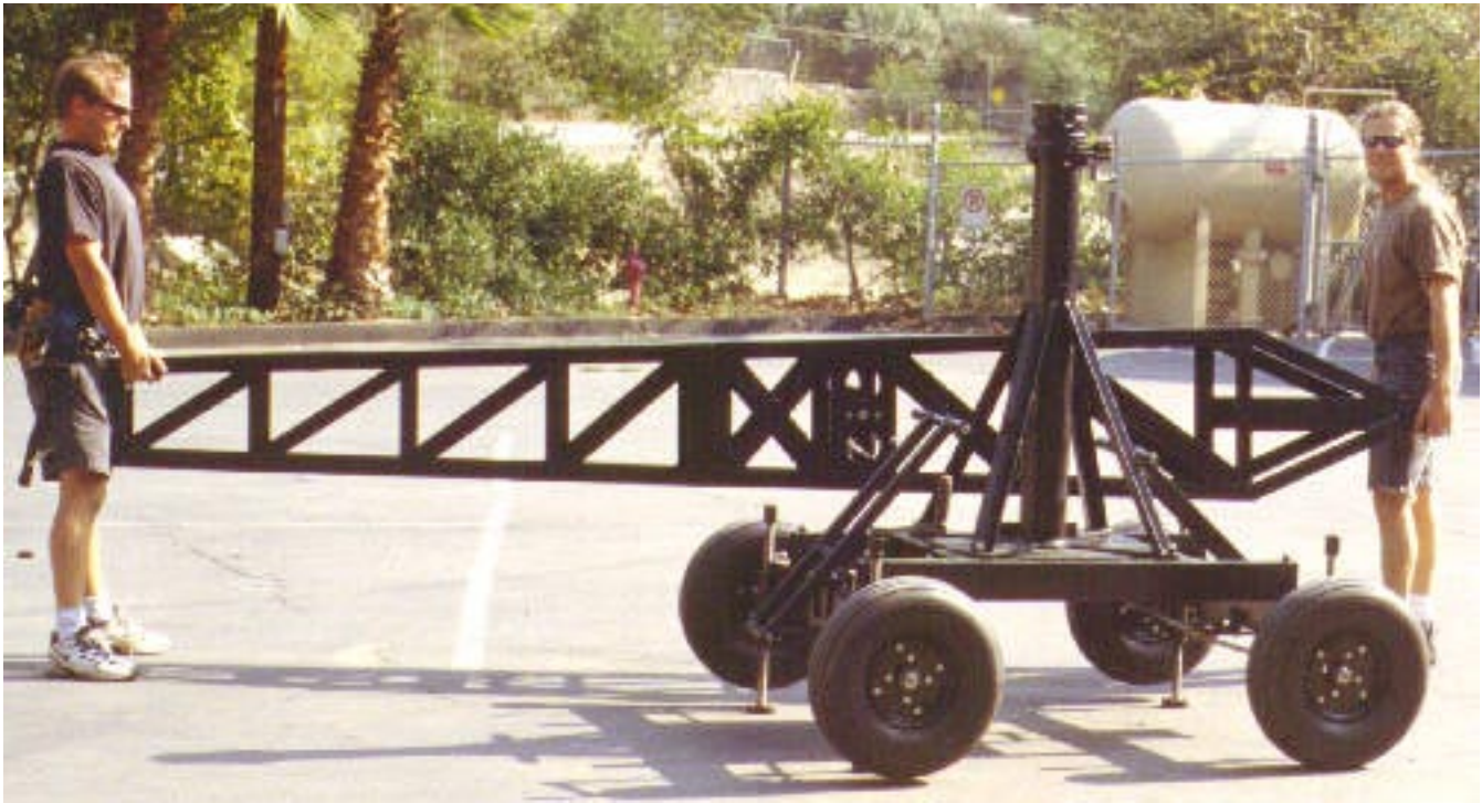
Mode 4 - Operating Platform - Step 3: Lift joined Boom #1 and Boom #2.
