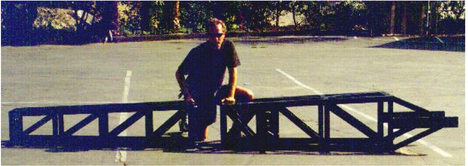
Mode 5 - Remote only - Step 1: Boom #1 and Boom #2 should be assembled on the ground.
