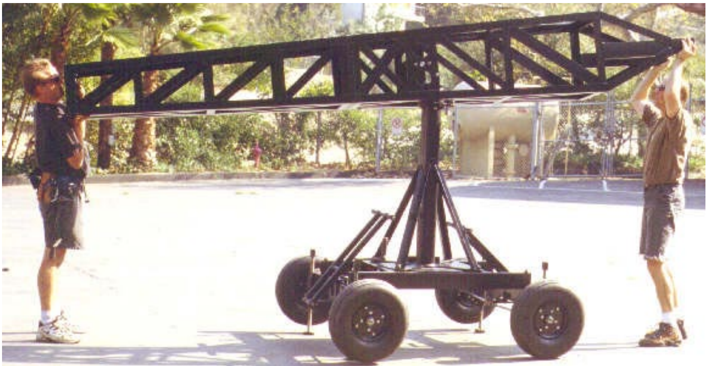
Mode 3 - Operation Platform - Step 4: Place horizontal main shaft from Boom #1 onto the main post and place the front of Boom #2 onto a ladder for support.
