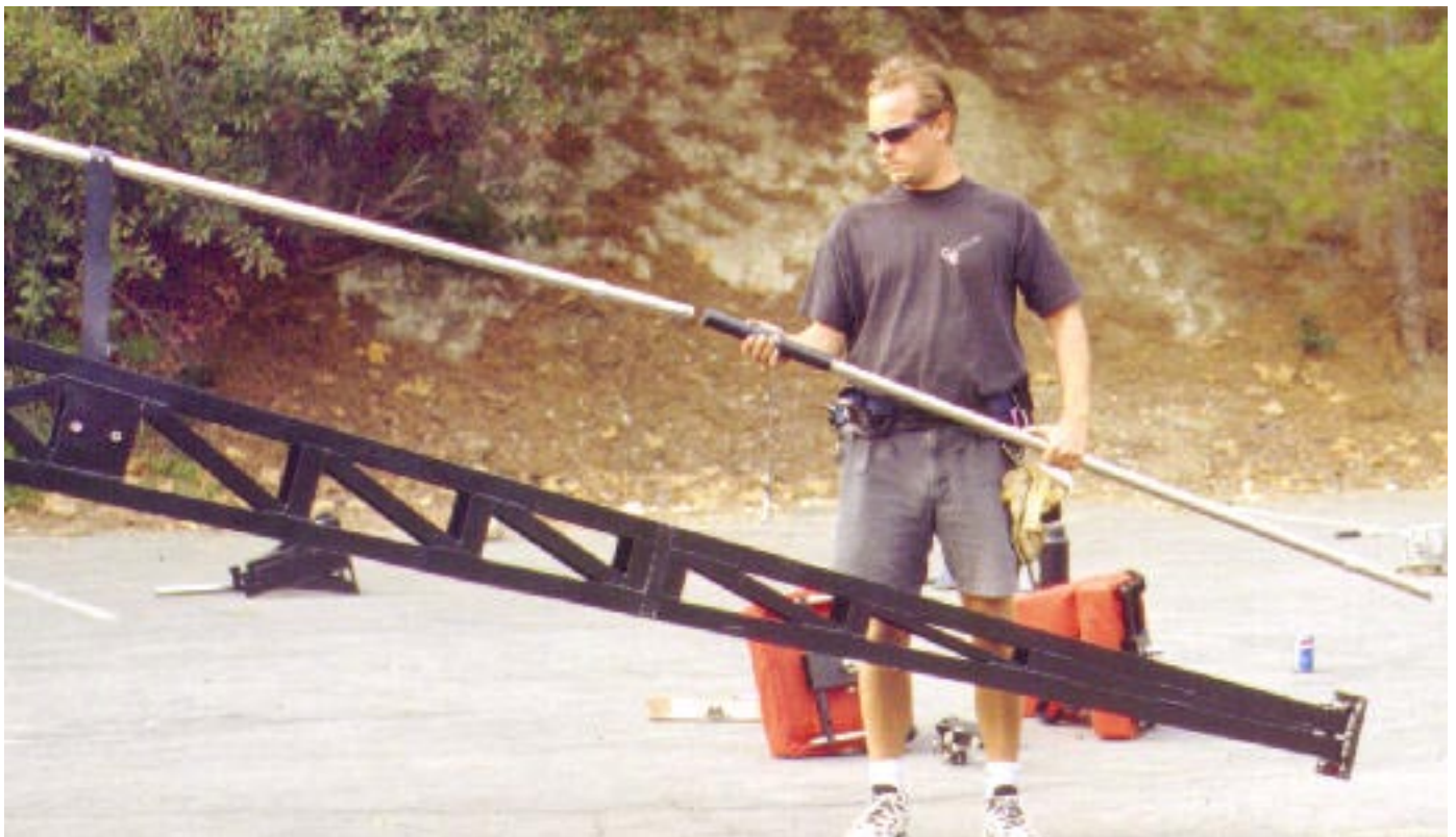
Mode 4 - Operating Platform - Step 16: Attach Rod #4 to the front of Rod #3 with the quikpin.
