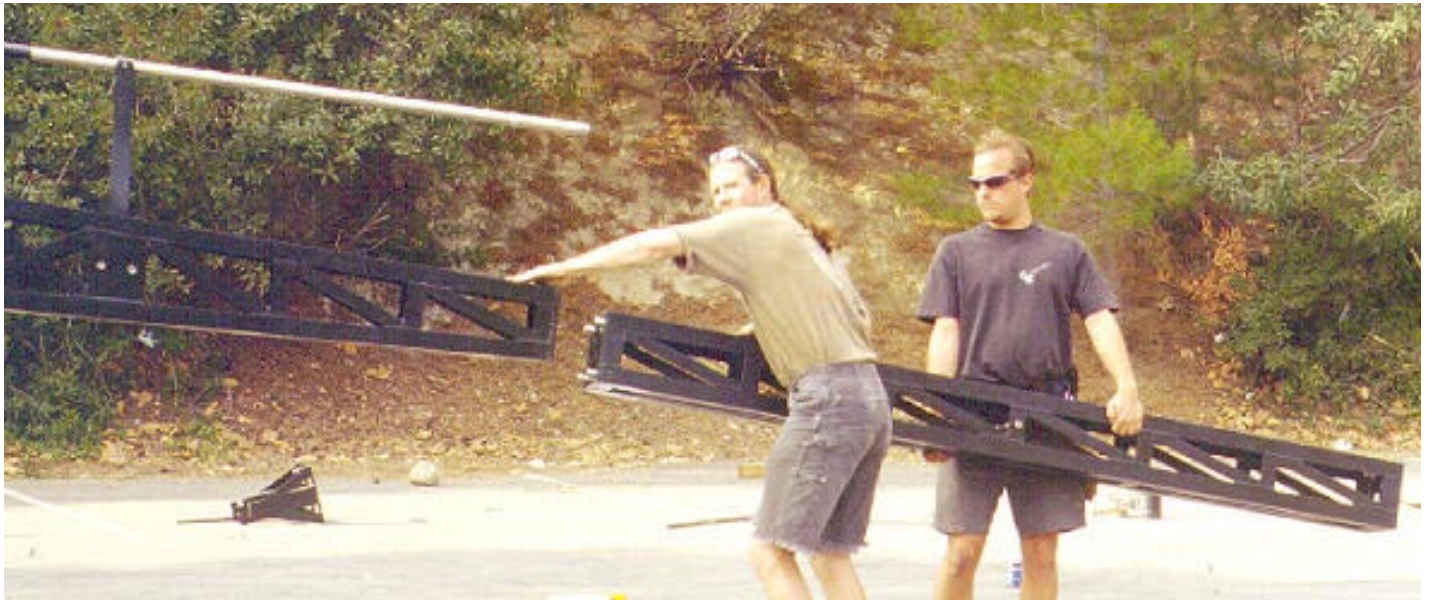
Mode 5 - Remote only - Step 15: Attach Remote Boom section (not tapered) to the front of Boom #3 and secure it with the 2 retaining bolts found inside Boom #3.
