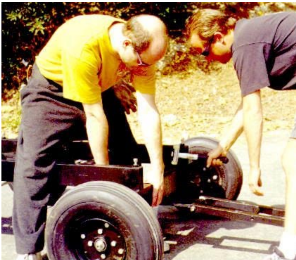
Mode 1+ - Remote Only - Step 2: Remove main crossbar from crane base.
