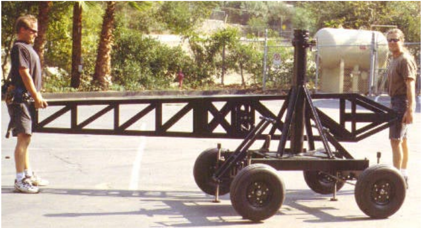
Mode 2 - Remote - Step 3: Lift joined Boom #1 and Boom #2.
