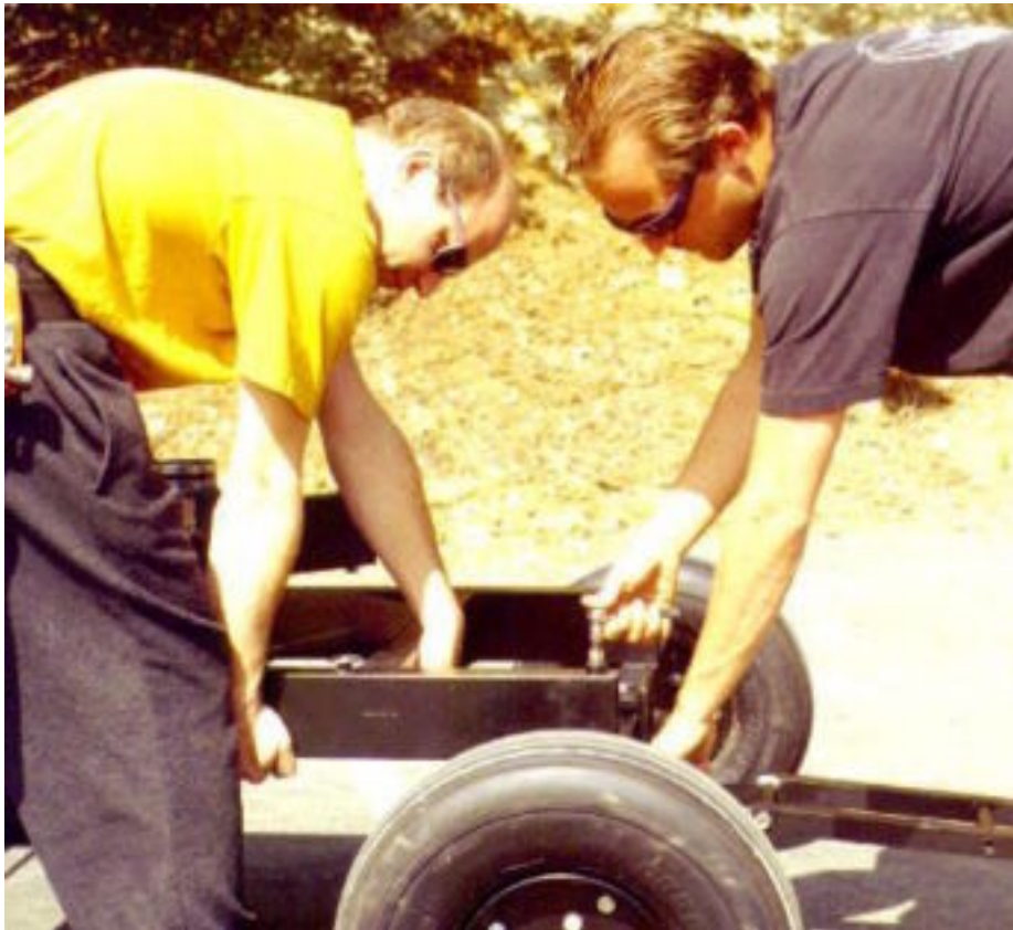
Mode 1+ - Remote Only - Step 1: Unbolt main crossbar from crane base.
