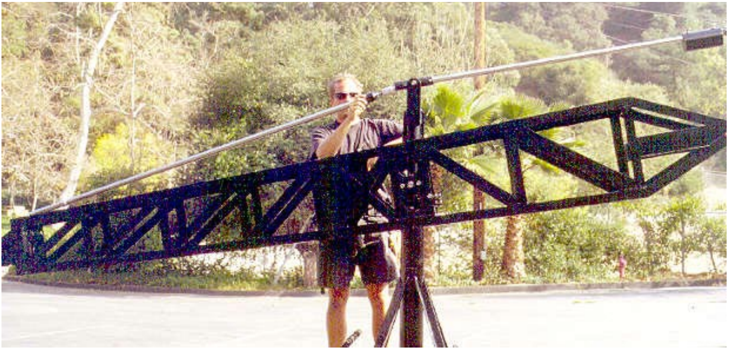
Mode 3 - Operation Platform - Step 9: Attach Rod # 2 to the front of the pylon (at post) with the quikpin.
