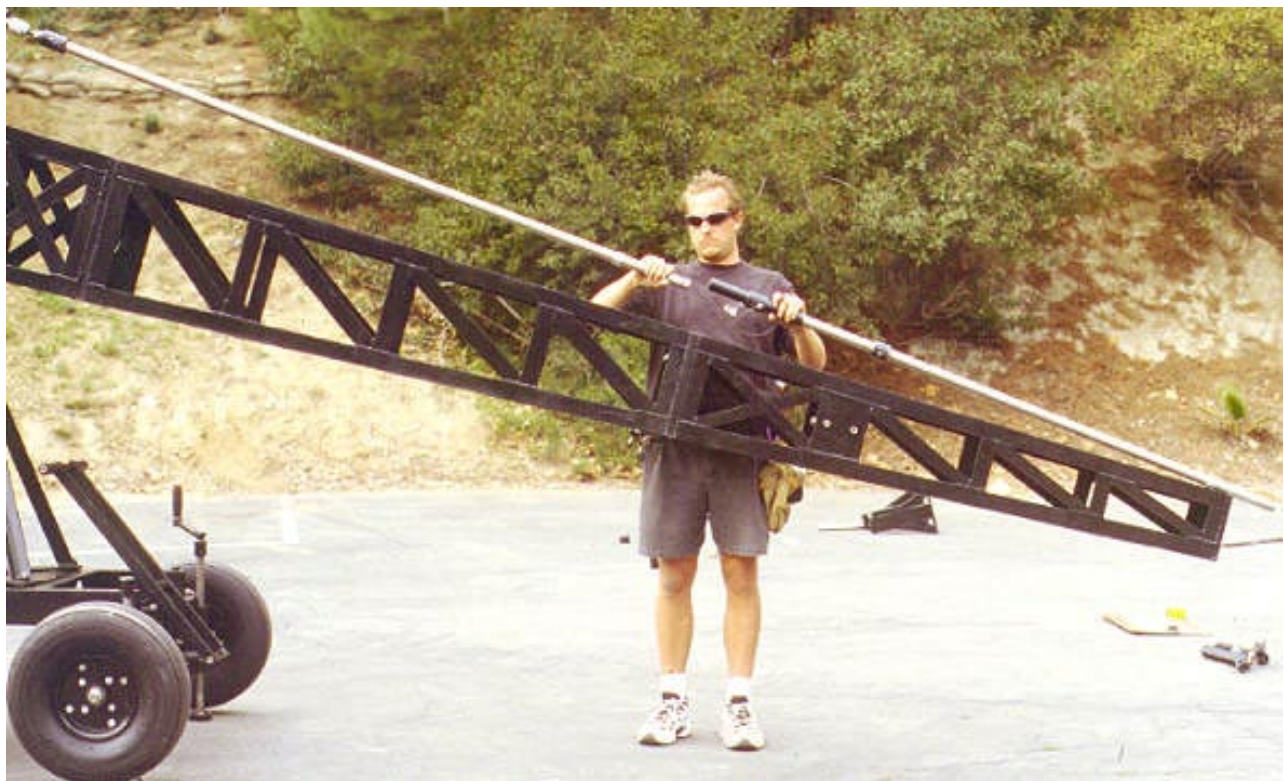
Mode 4 - Remote - Step 12: Add Rod #3 to the front of Rod #2 and secure with the quikpin.
