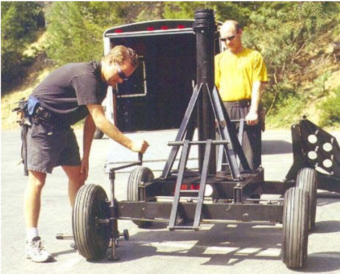
Leveling - Step 5: Turn handle clockwise to lower jack.
