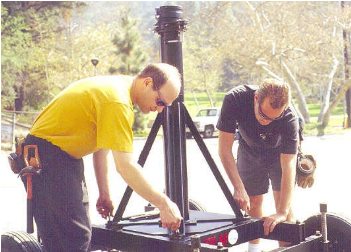
Mode 1 - Operating Platform - Step 3: Remove main crossbar from crane base.
