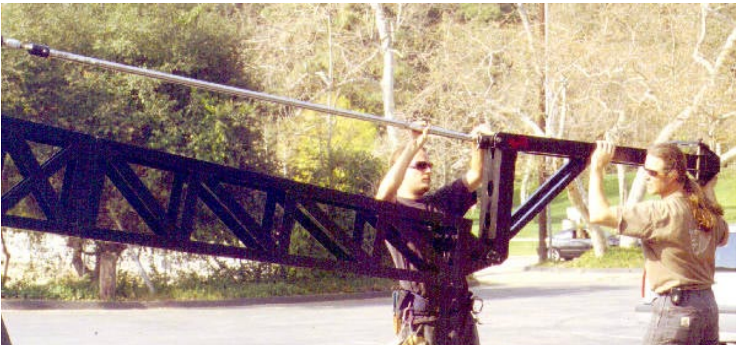
Mode 2 - Remote - Step 12: Secure Rod #2 to remote head section with the quikpin.
