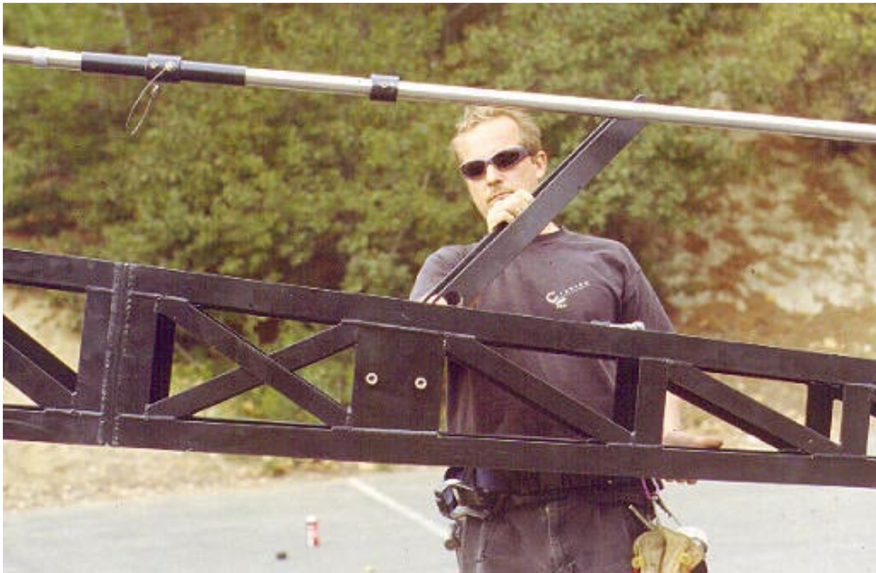
Mode 3 - Remote - Step 13: Place rod support bracket over the horizontal shaft an Boom #3.
