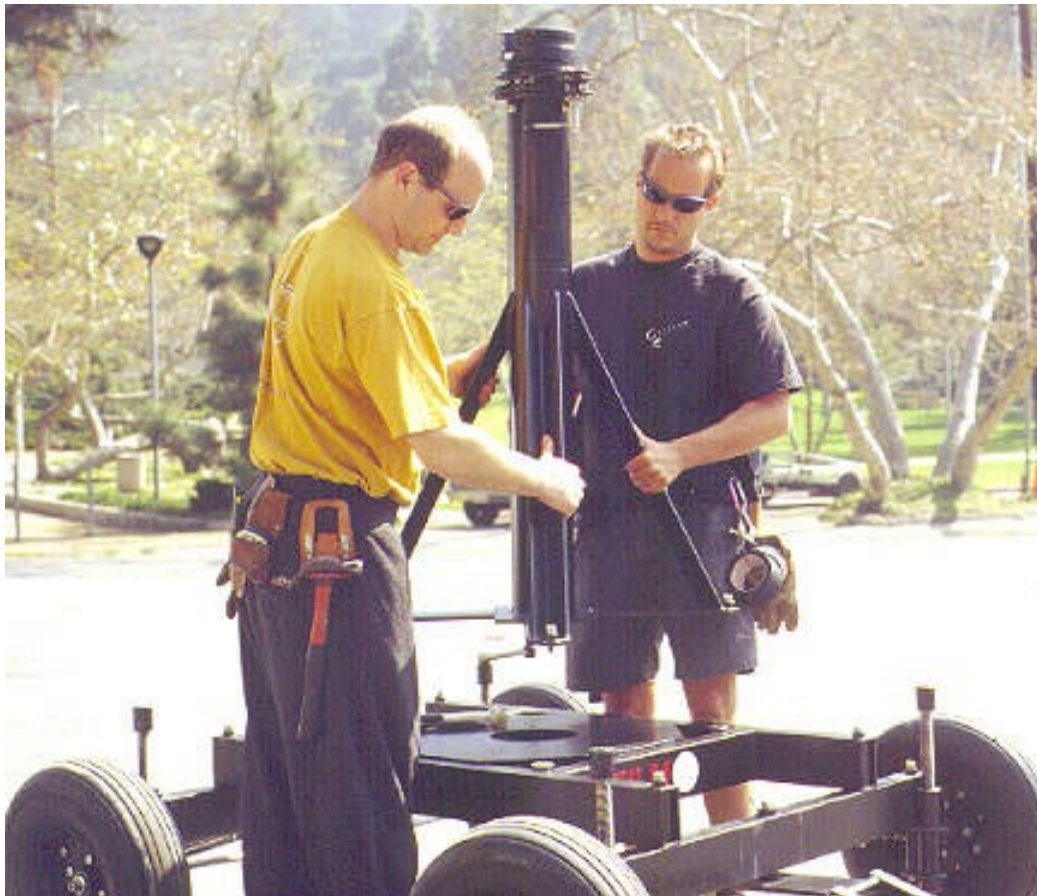
Mode 1 - Operating Platform - Step 4: Remove main post.
