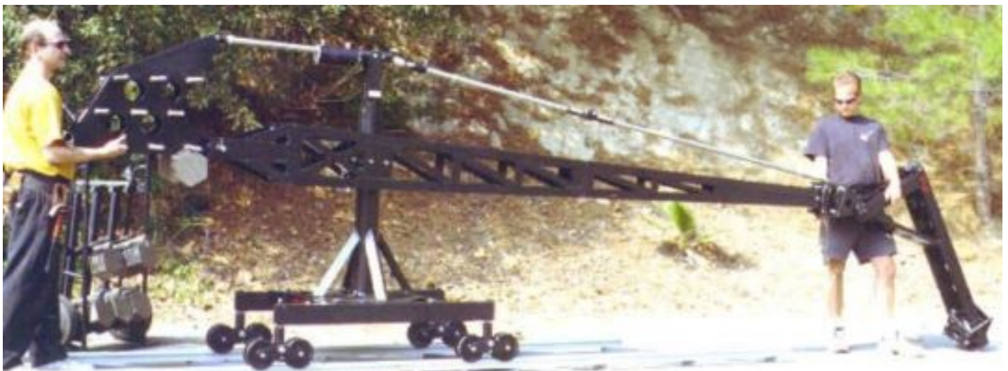
Mode 1+ - Remote Only - Step 18: Attach remote nose section only.
