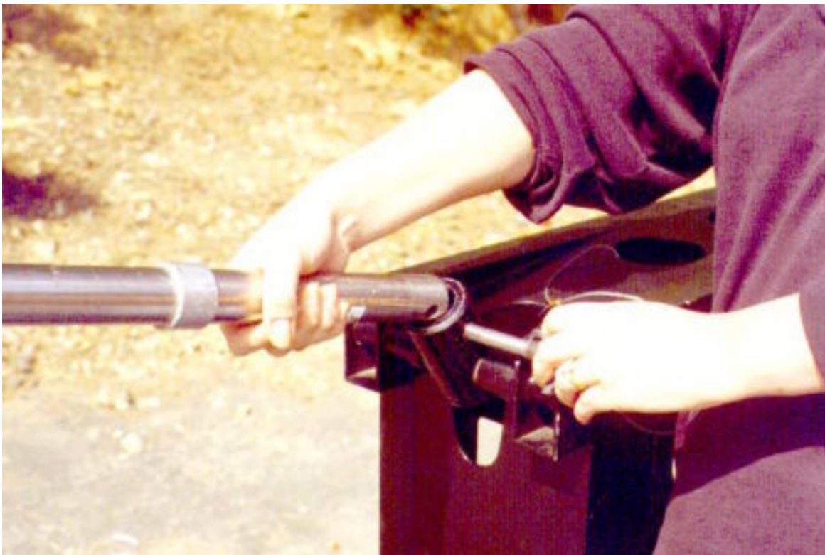
Mode 1 - Remote - Step 16: Now attach rod A to the pylon on the other side with the quikpin.
