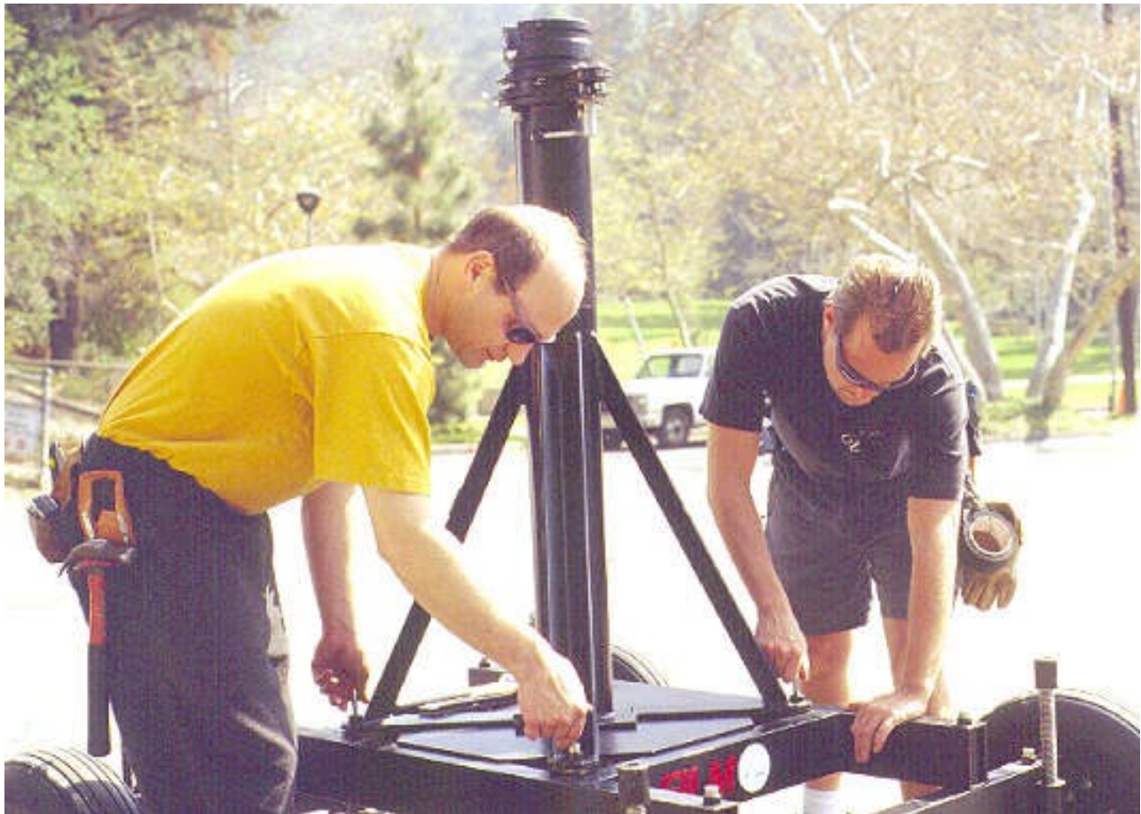
Dolly narrow mode - Step 1: Unbolt main post from crane base.
