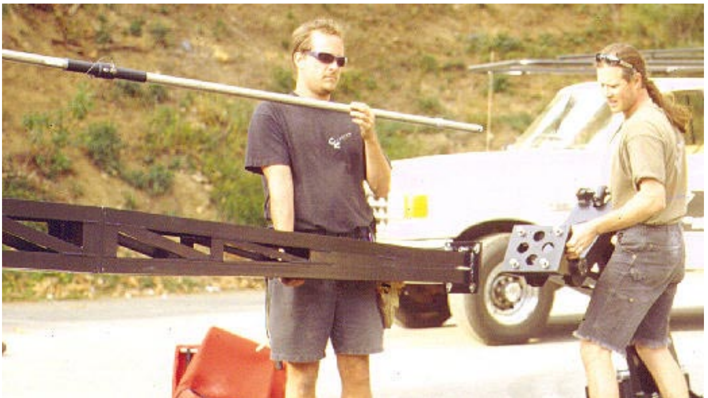
Mode 5 - Remote only - Step 20: Attach remote head section to the front of Boom #4 with the 2 retaining bolts found on the outside front of Boom #4.
