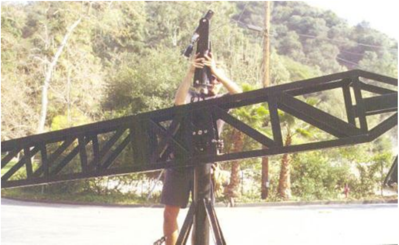
Mode 3 - Operation Platform - Step 5: Attach pylon assembly onto main post with 4 bolts, captivating the horizontal main shaft (make sure threaded end of pylon faces forward so you can level the Operating platform later!)
