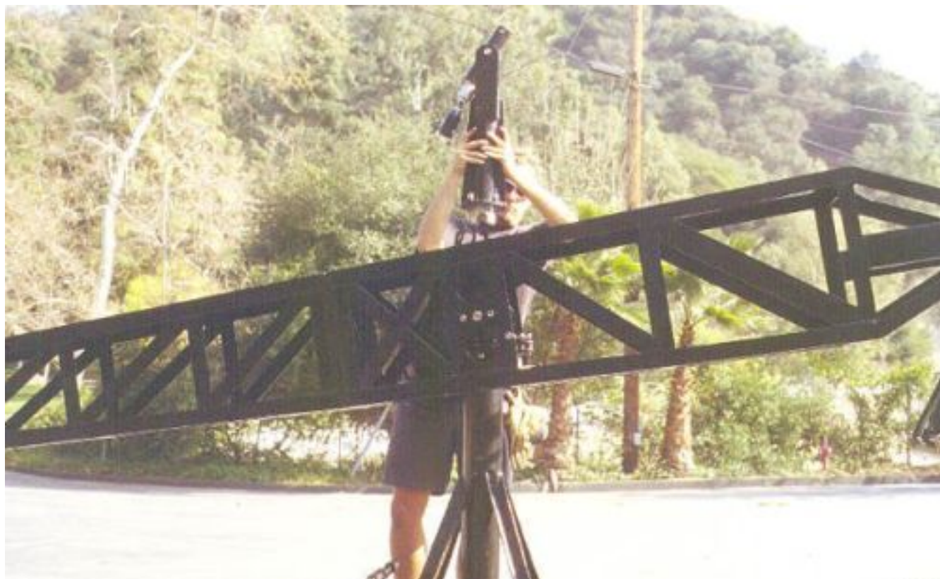
Mode 2 - Remote - Step 5: Attach pylon assembly onto main post with 4 bolts, captivating the horizontal main shaft (make sure threaded end of pylon faces forward so you can level the Operating platform later!)
