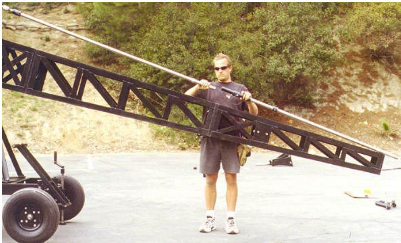
Mode 5 - Remote only - Step 12: Add Rod #3 to the front of Rod #2 and secure with the quikpin.
