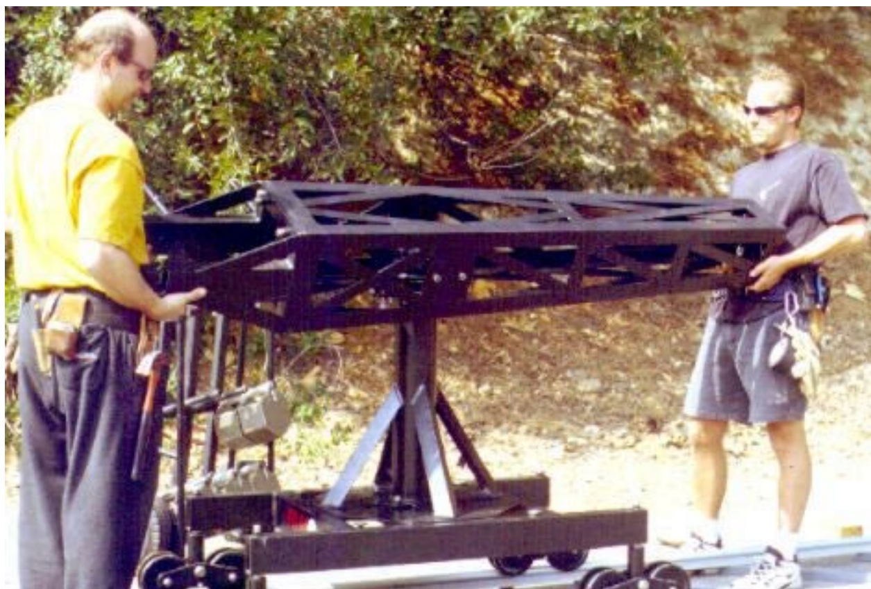
Mode 1+ - Remote Only - Step 12: Place Boom #3 with mini bucket attachment onto mini post making sure to angle Boom #3 so it fits over the mini post- place it onto the horizontal main shaft inside Boom #3.
