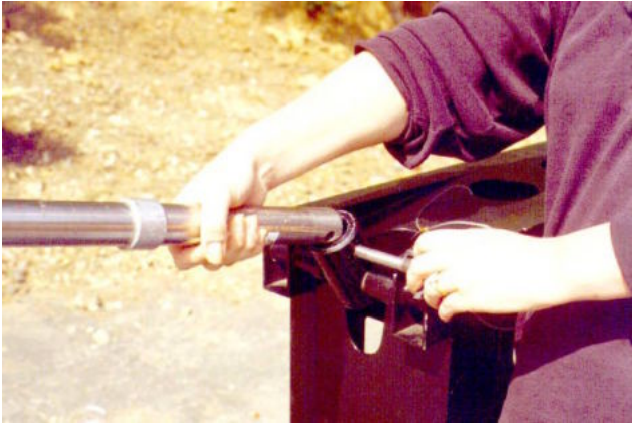
Mode 4 - Remote - Step 19: Secure Rod #4 to the remote head section.
