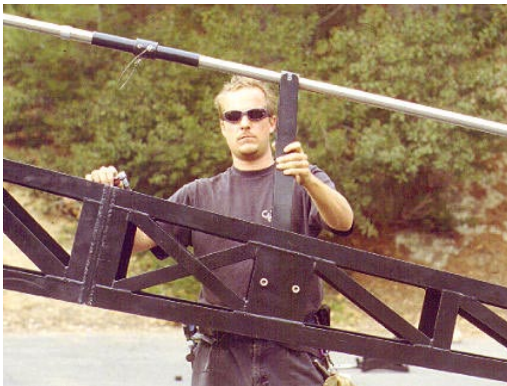
Mode 3 - Operation Platform - Step 14: Click Rod #3 into the top of the rod support bracket.
