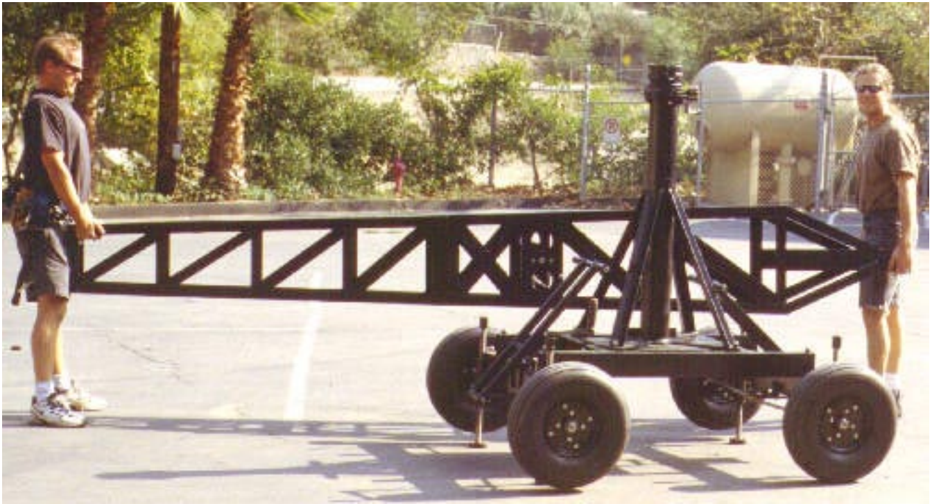
Mode 2 - Operating Platform - Step 3: Lift joined Boom #1 and Boom #2.
