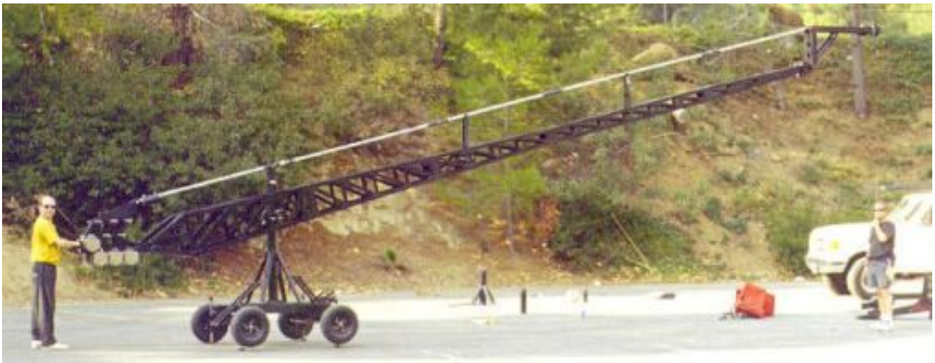
Mode 5 - Remote only - Step 22: Counterweight remote head section and all Booms. (Always keep the arm in balance as you build crane in any mode.)
