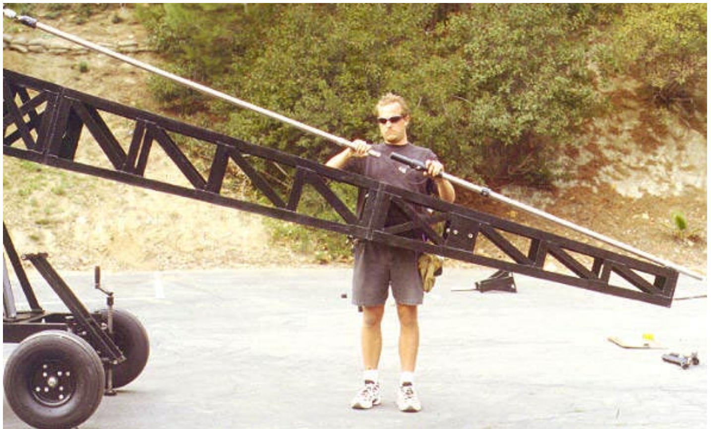
Mode 4 - Operating Platform - Step 12: Add Rod #3 to the front of Rod #2 and secure with the quikpin.
