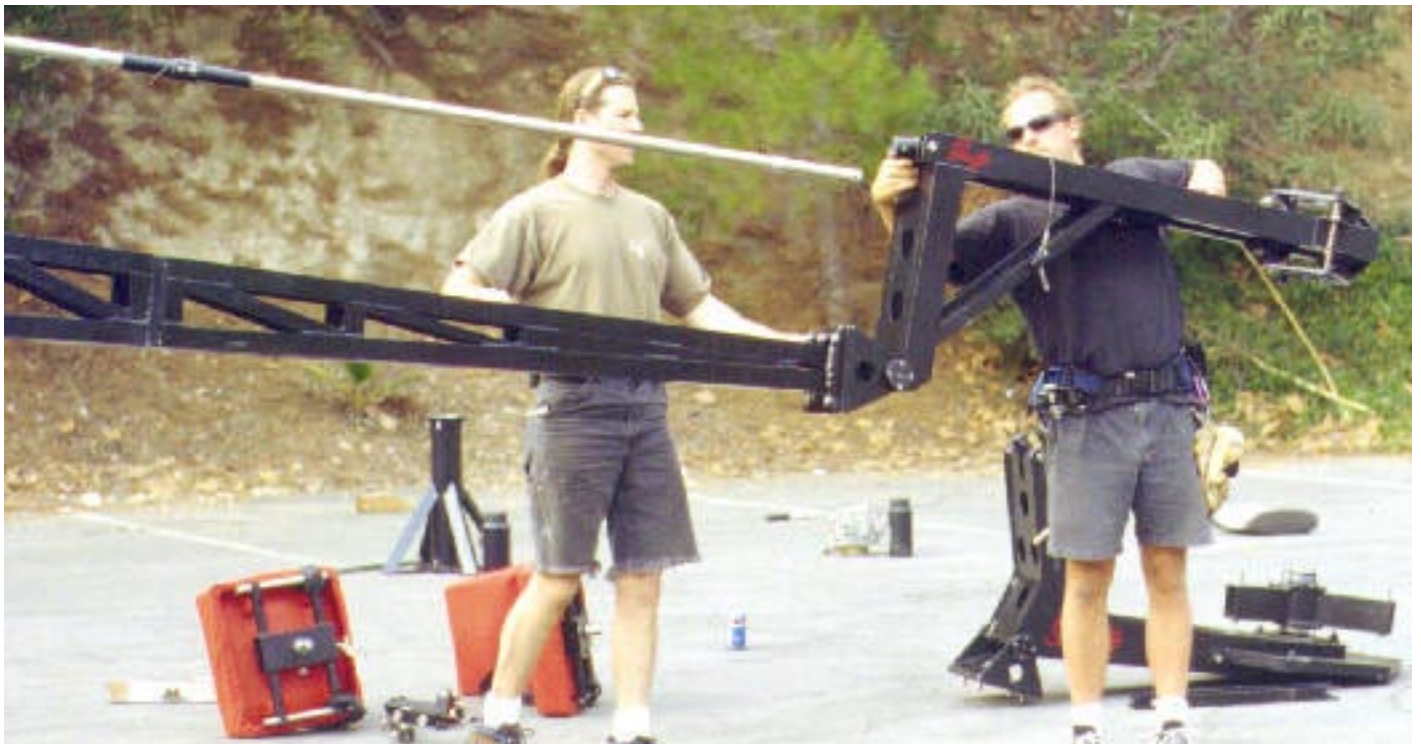
Mode 4 - Remote - Step 20: Secure it with quikpin.
