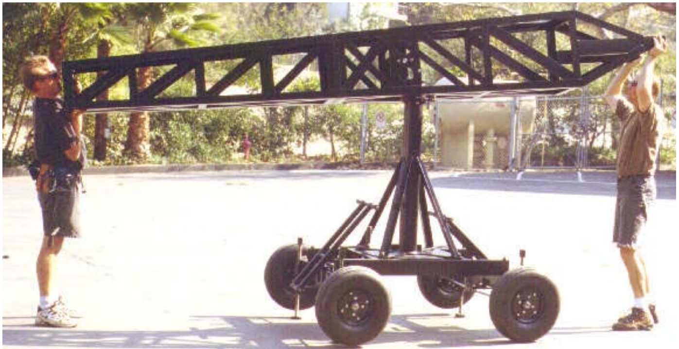
Mode 4 - Remote - Step 4: Place horizontal main shaft from Boom #1 onto the main post and place the front of Boom #2 onto a ladder for support.
