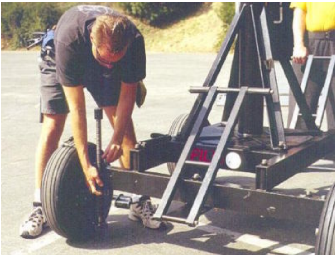
Leveling - Step 2: Hold jack up into receiving hole and hand-thread the bolt (on crossbar) into it.
