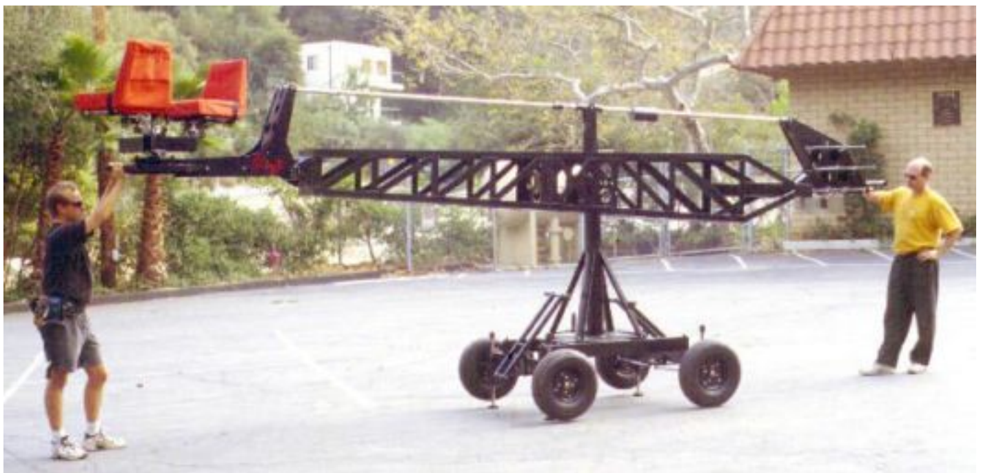
Mode 2 - Operating Platform - Step 14: Add seats, risers, 4-way leveling head, battery box, etc (always keep the arm in balance as you build crane in any mode). End of steps.
