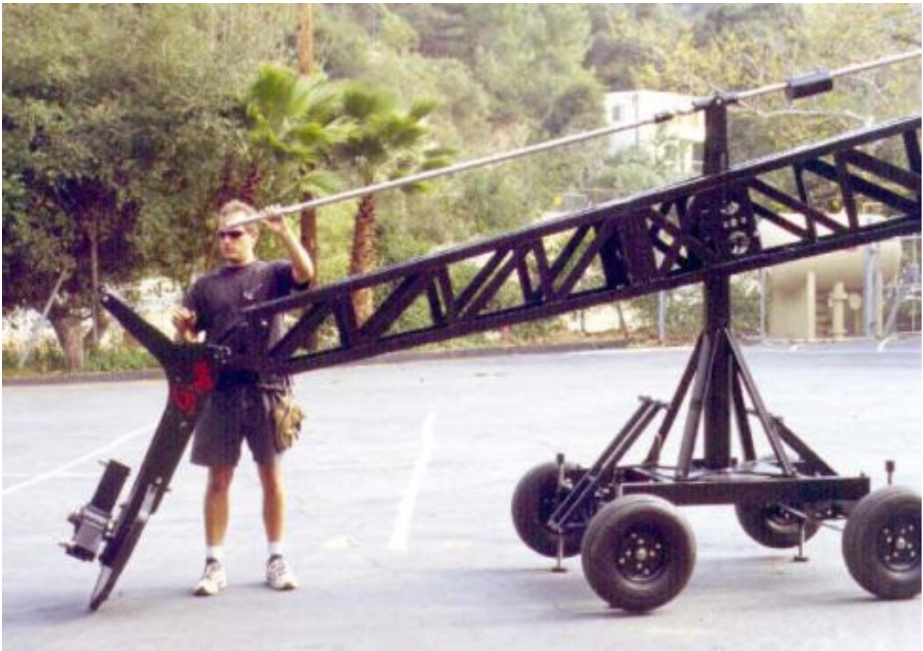
Mode 2 - Operating Platform - Step 11: Lift the front of the operating platform while another readies with the quikpin to attach it to Rod #2.
