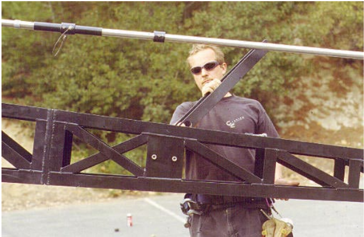
Mode 4 - Remote - Step 13: Place rod support bracket over the horizontal shaft an Boom #3.
