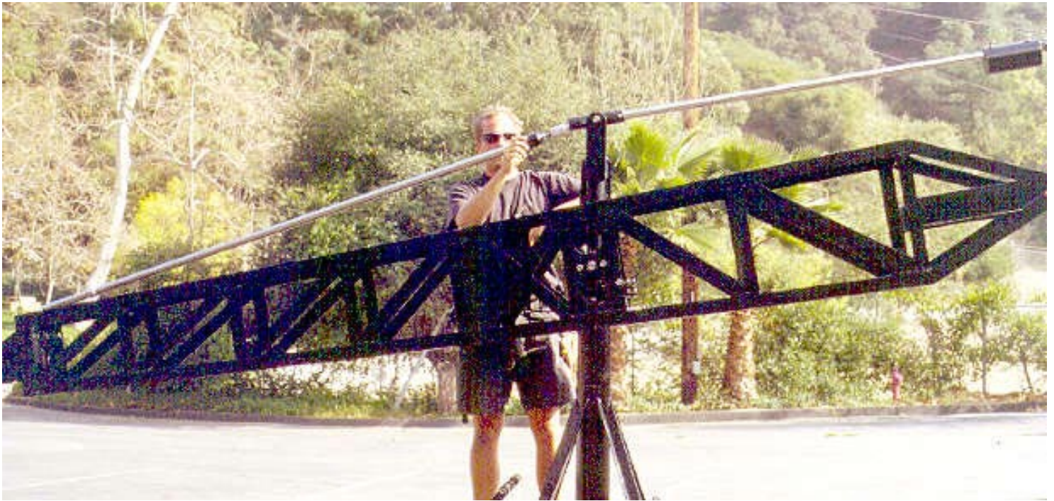
Mode 2 - Remote - Step 9: Attach Rod # 2 to the front of the pylon (at post) with the quikpin.
