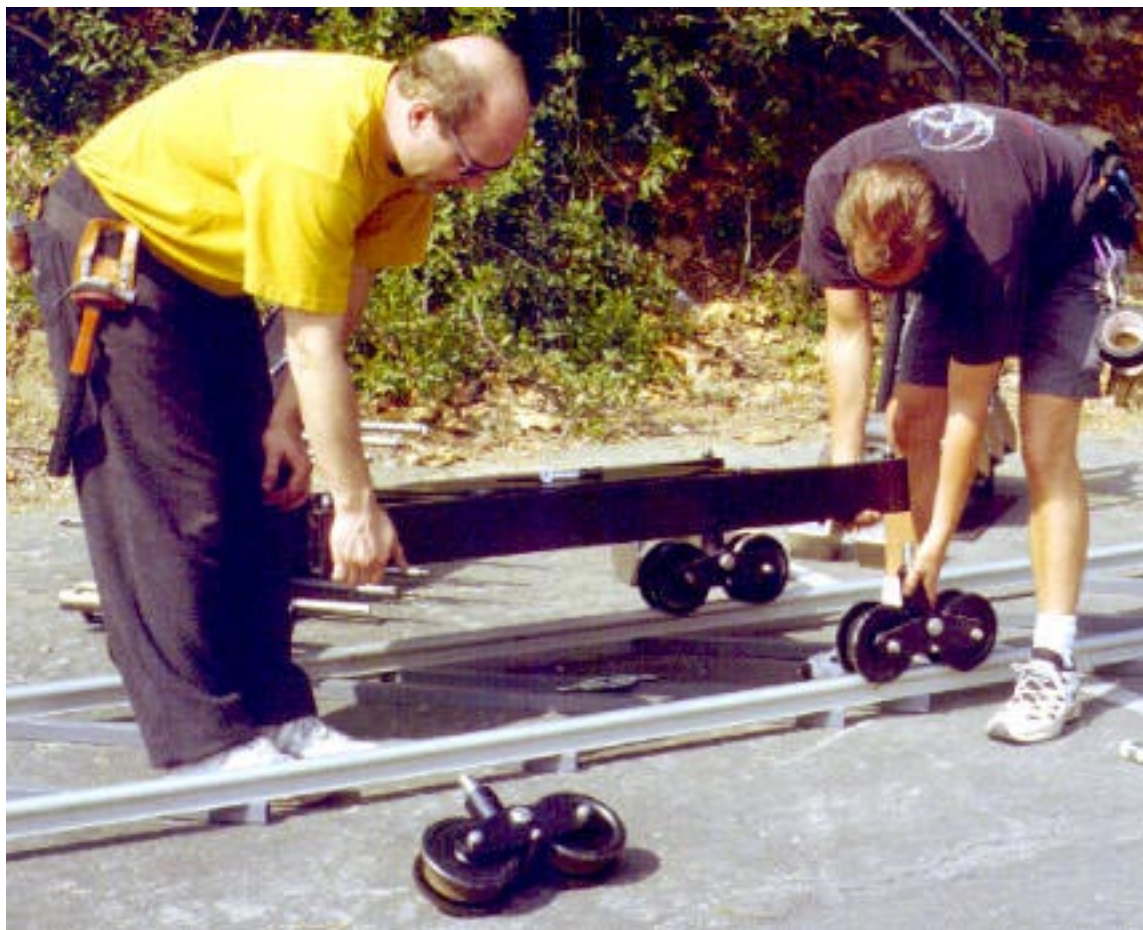
Mode 1 - Remote - Step 6: Attach track wheels to narrow base where main crossbar attached before its removal.
