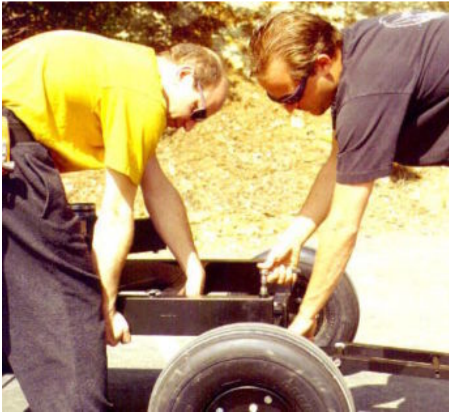
Mode 1 - Remote - Step 1: Unbolt main crossbar from crane base.
