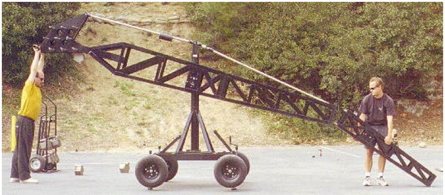
Mode 3 - Operation Platform - Step 10: Attach Boom #3 to the front of Boom #2.
