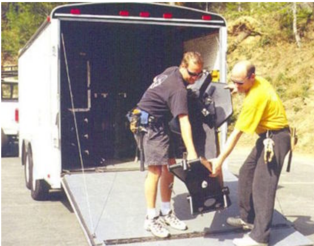
Trailer - Step 6: On Crane 1 remove Operating Platform next.
