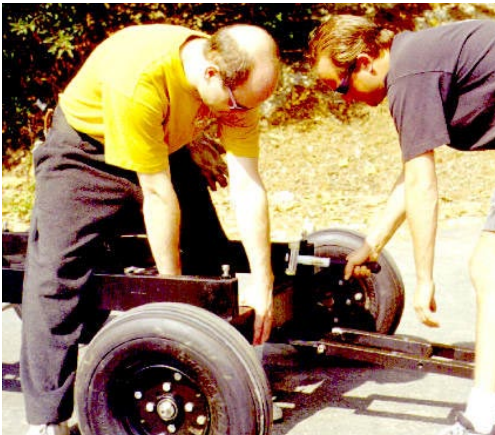
Mode 1 - Remote - Step 2: Remove main crossbar from crane base.
