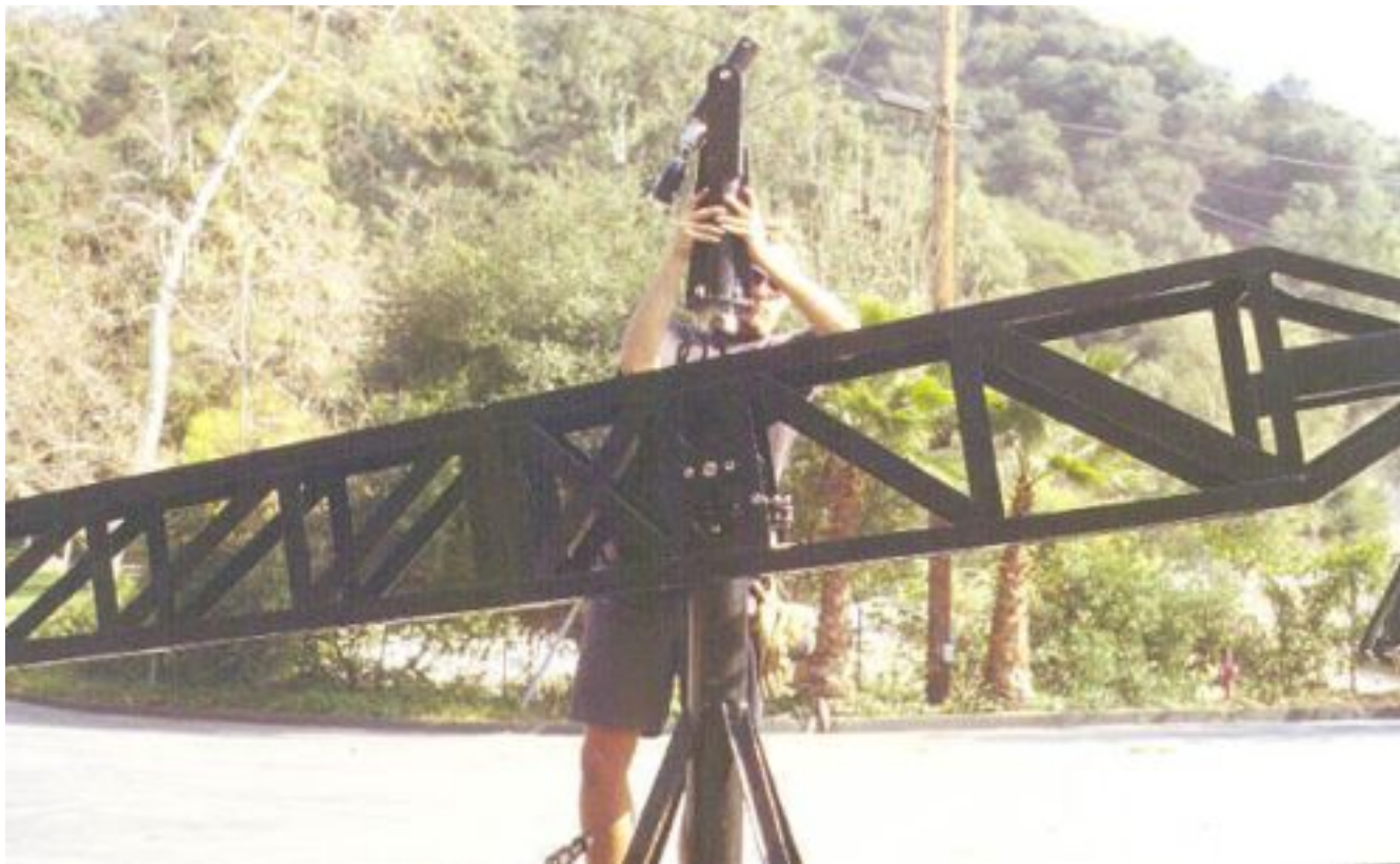
Mode 4 - Remote - Step 5: Attach pylon assembly onto main post with 4 bolts, captivating the horizontal main shaft (make sure threaded end of pylon faces forward so you can level the Operating platform later!)
