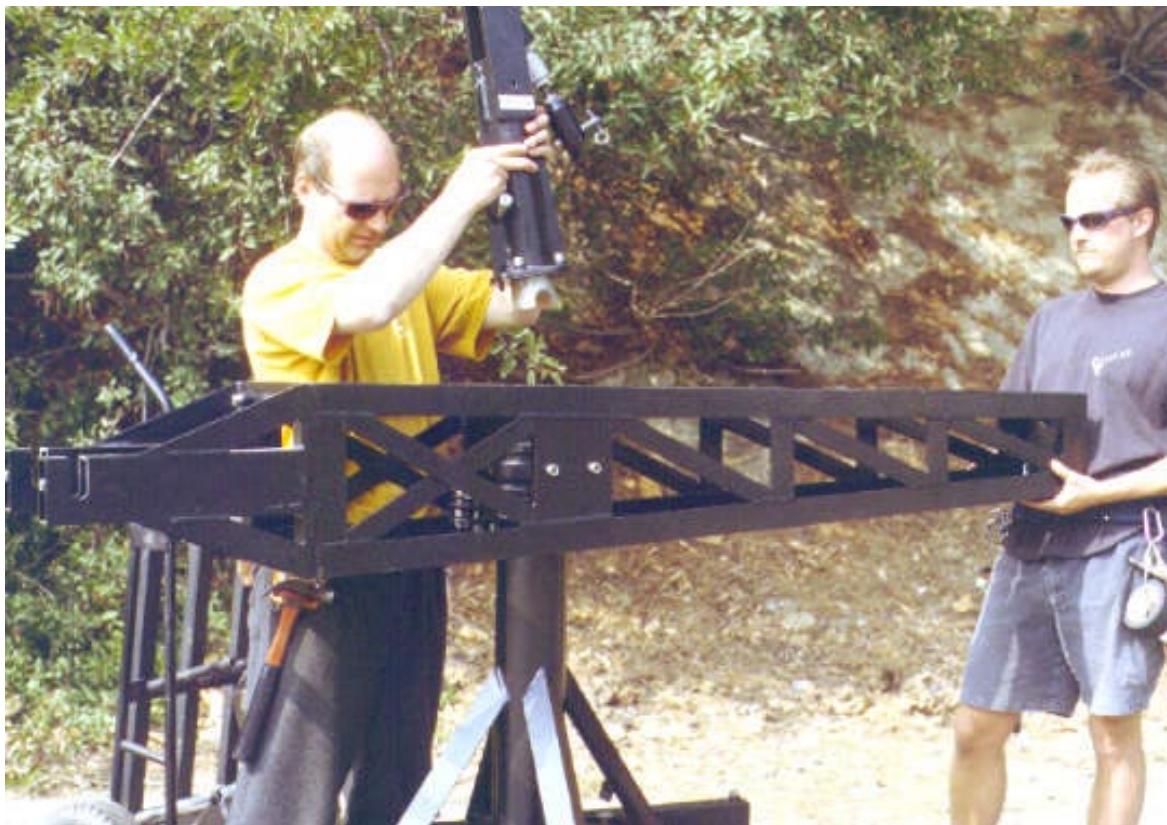
Mode 1 - Operating Platform - Step 13: Attach pylon assembly to mini post with 4 bolts in pylon. Horizontal shaft is then trapped into place (be sure that threaded end of the pylon rod section is facing towards the front- so you can level operating platform later!)
