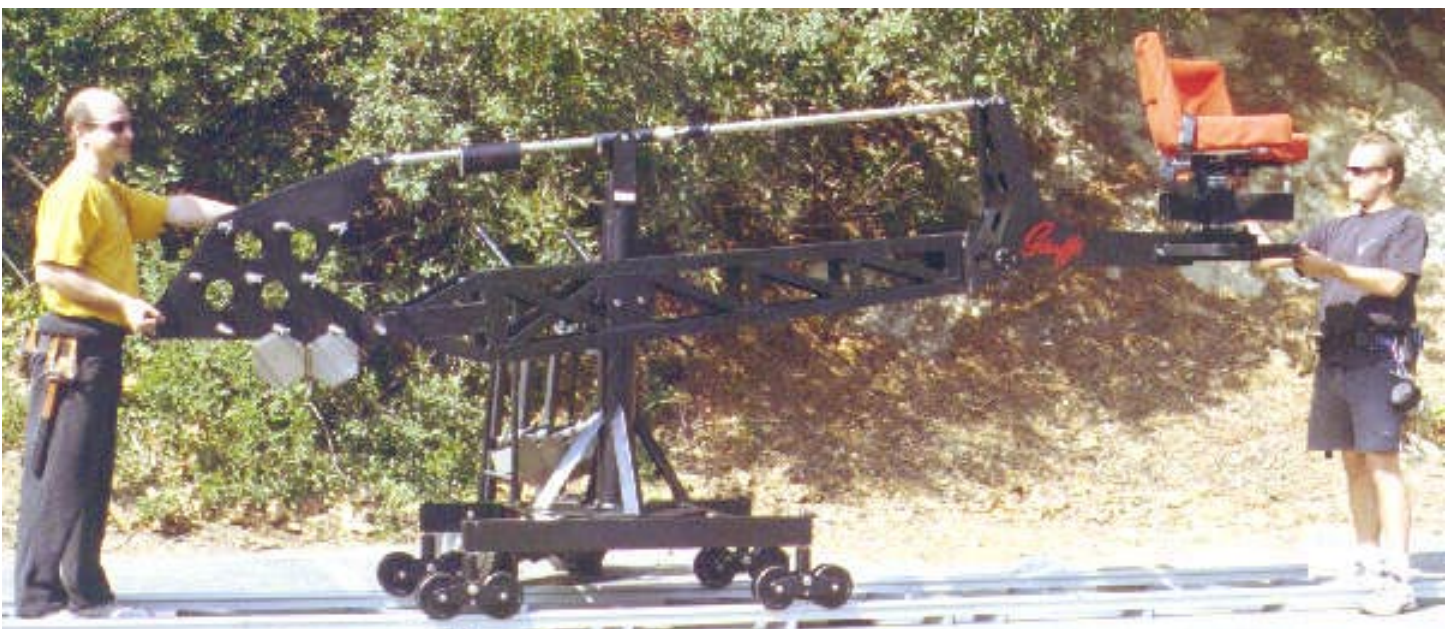
Mode 1 - Operating Platform - Step 18: Add seats, risers, 4-way leveling head, battery box, etc. (Always keep the arm in balance as you build cranes in any mode.)
