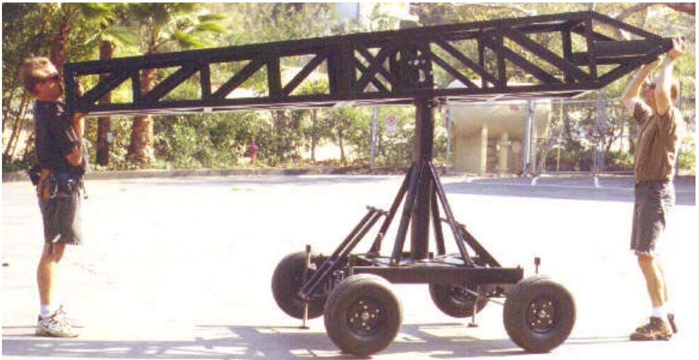
Mode 2 - Remote - Step 4: Place horizontal main shaft from Boom #1 onto the main post and place the front of Boom #2 onto a ladder for support.
