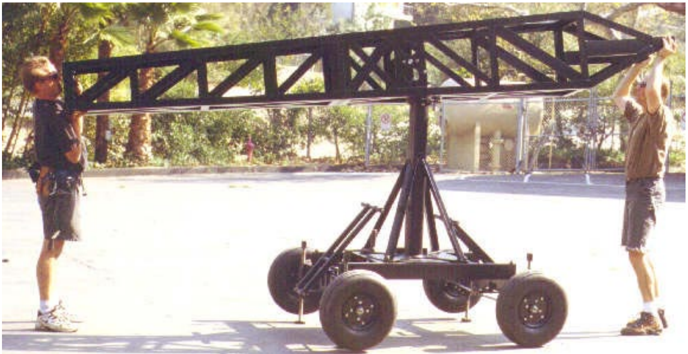
Mode 3 - Remote - Step 4: Place horizontal main shaft from Boom #1 onto the main post and place the front of Boom #2 onto a ladder for support.
