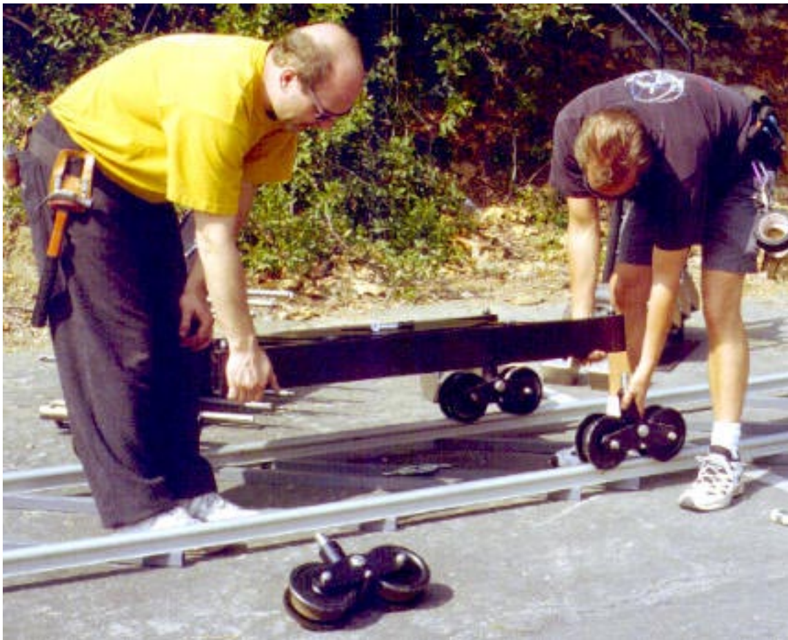
Mode 1 - Operating Platform - Step 6: Attach track wheels to narrow base where main crossbar attached before its removal.
