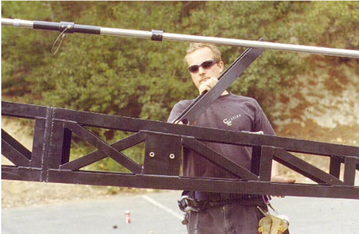
Mode 4 - Operating Platform - Step 13: Place rod support bracket over the horizontal shaft an Boom #3.
