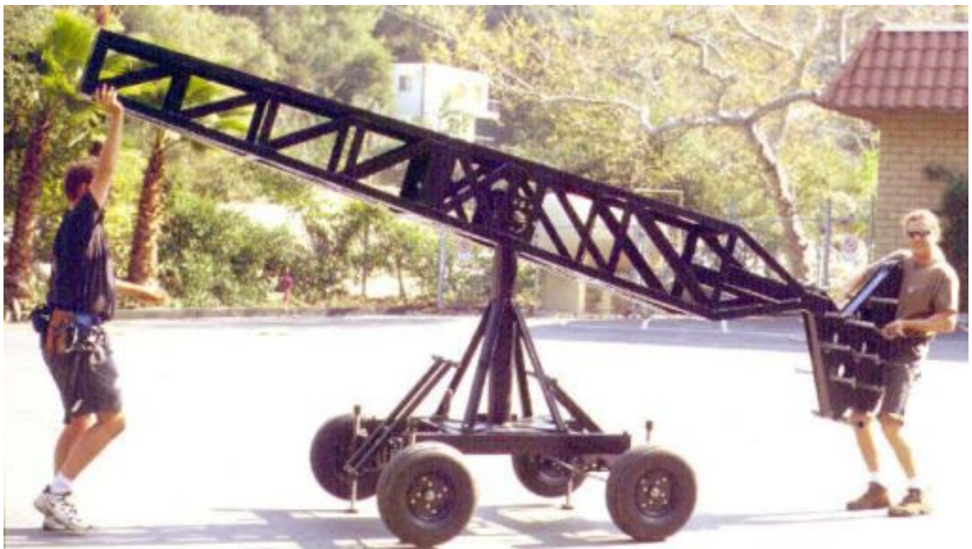
Mode 3 - Operation Platform - Step 6: Add weight box into the slots on the back of Boom #1 and tighten the two retaining bolts (make sure that the weight box shaft isn't resting on the 2 retaining bolts).
