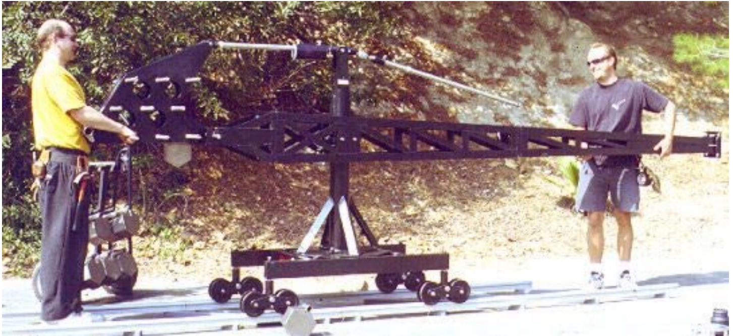
Mode 1+ - Remote Only - Step 16: Add Rod A and Boom section #4.
