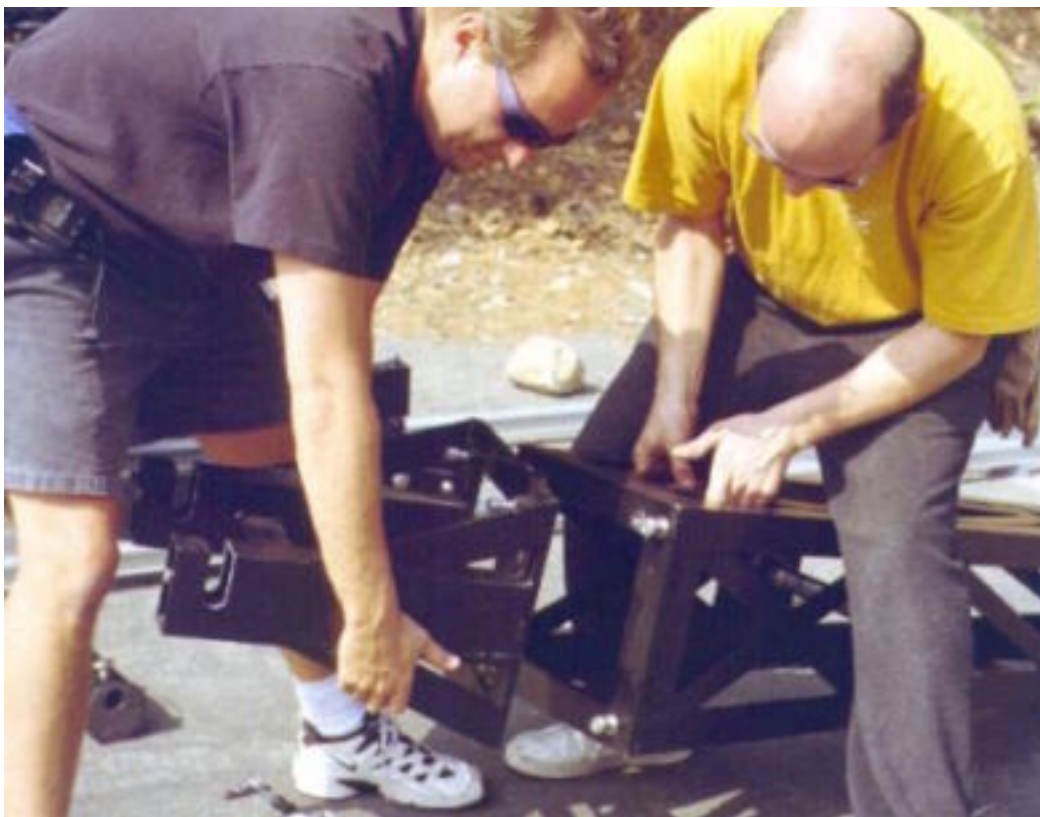
Mode 1+ - Remote Only - Step 11: Attach mini bucket to the back of Boom #3 with 2 retaining bolts on mini bucket.
