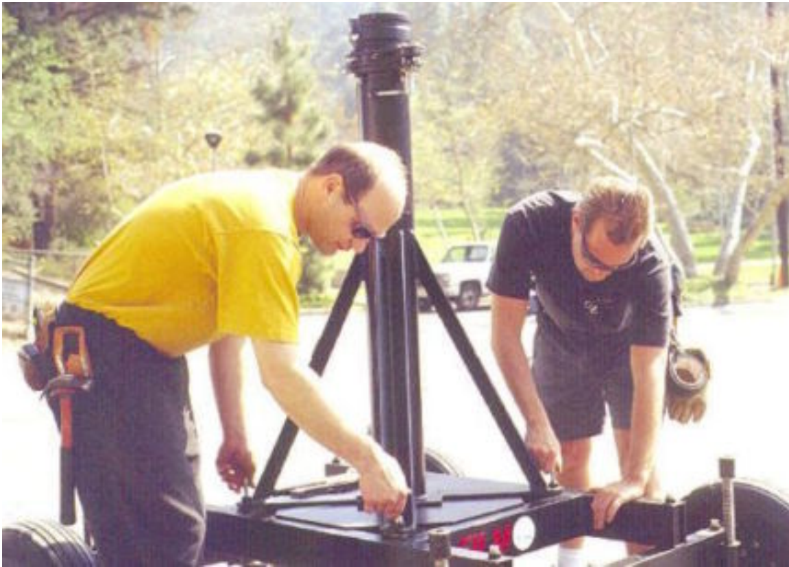
Mode 1+ - Remote Only - Step 3: Unbolt main post.
