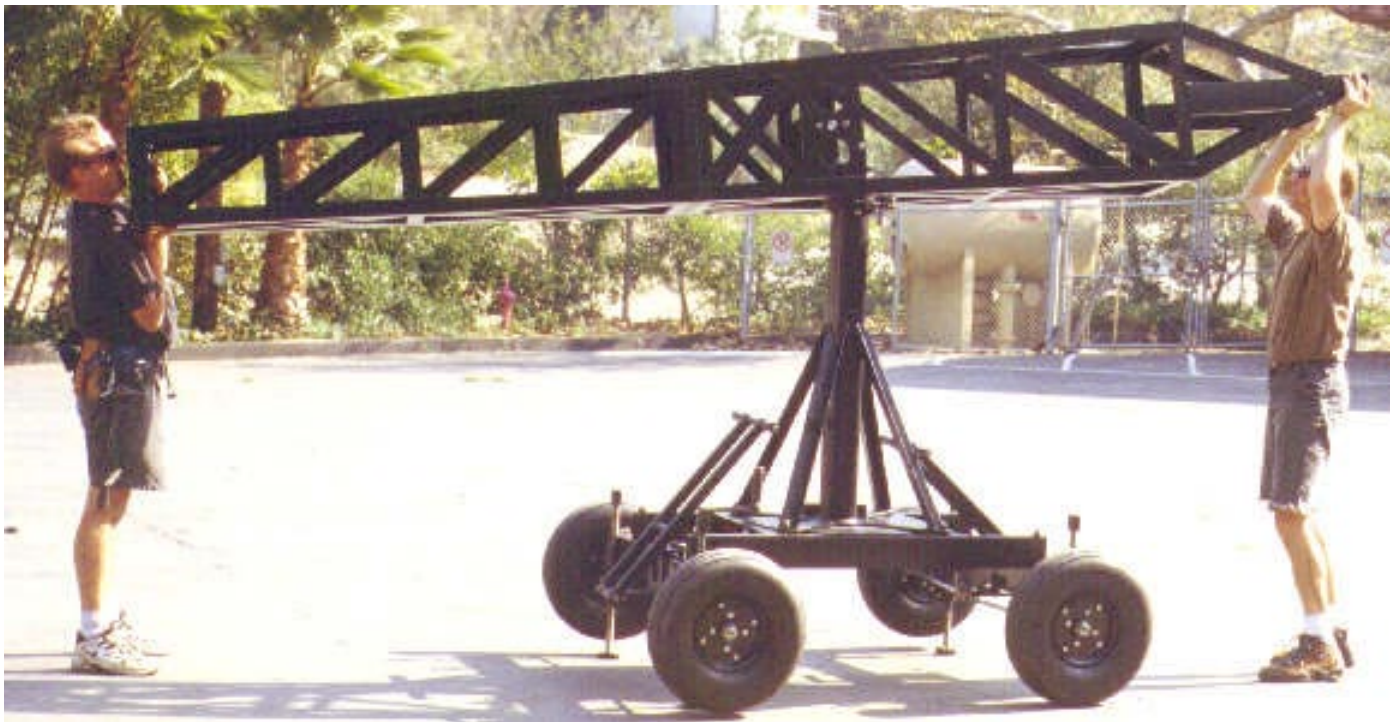
Mode 4 - Operating Platform - Step 4: Place horizontal main shaft from Boom #1 onto the main post and place the front of Boom #2 onto a ladder for support.
