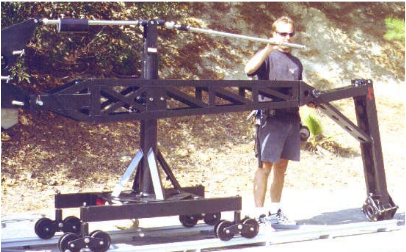
Mode 1 - Remote - Step 18: Add rod B (mini rod) between the front of the pylon and the remote head section with the quikpins.
