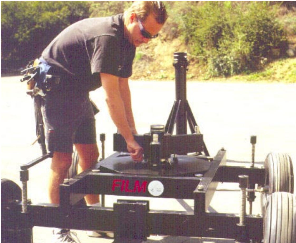
Dolly wide mode - Step 5: Place, then bolt swivel seat unit to the crane base.
