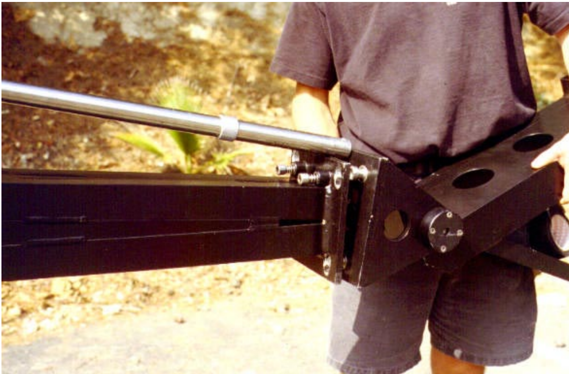
Mode 1 - Remote - Step 17: Attach remote head section to the front of boom #3 with 2 retaining bolts inside boom #3.
