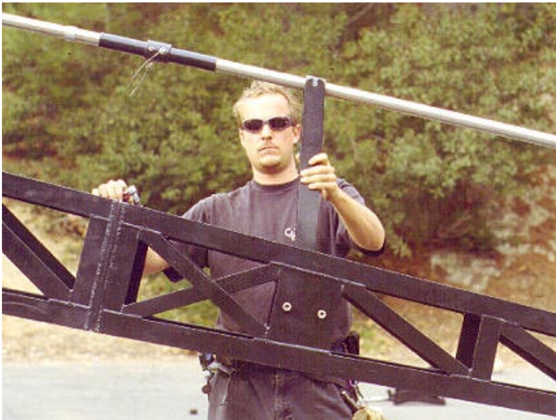
Mode 4 - Remote - Step 14: Click Rod #3 into the top of the rod support bracket.
