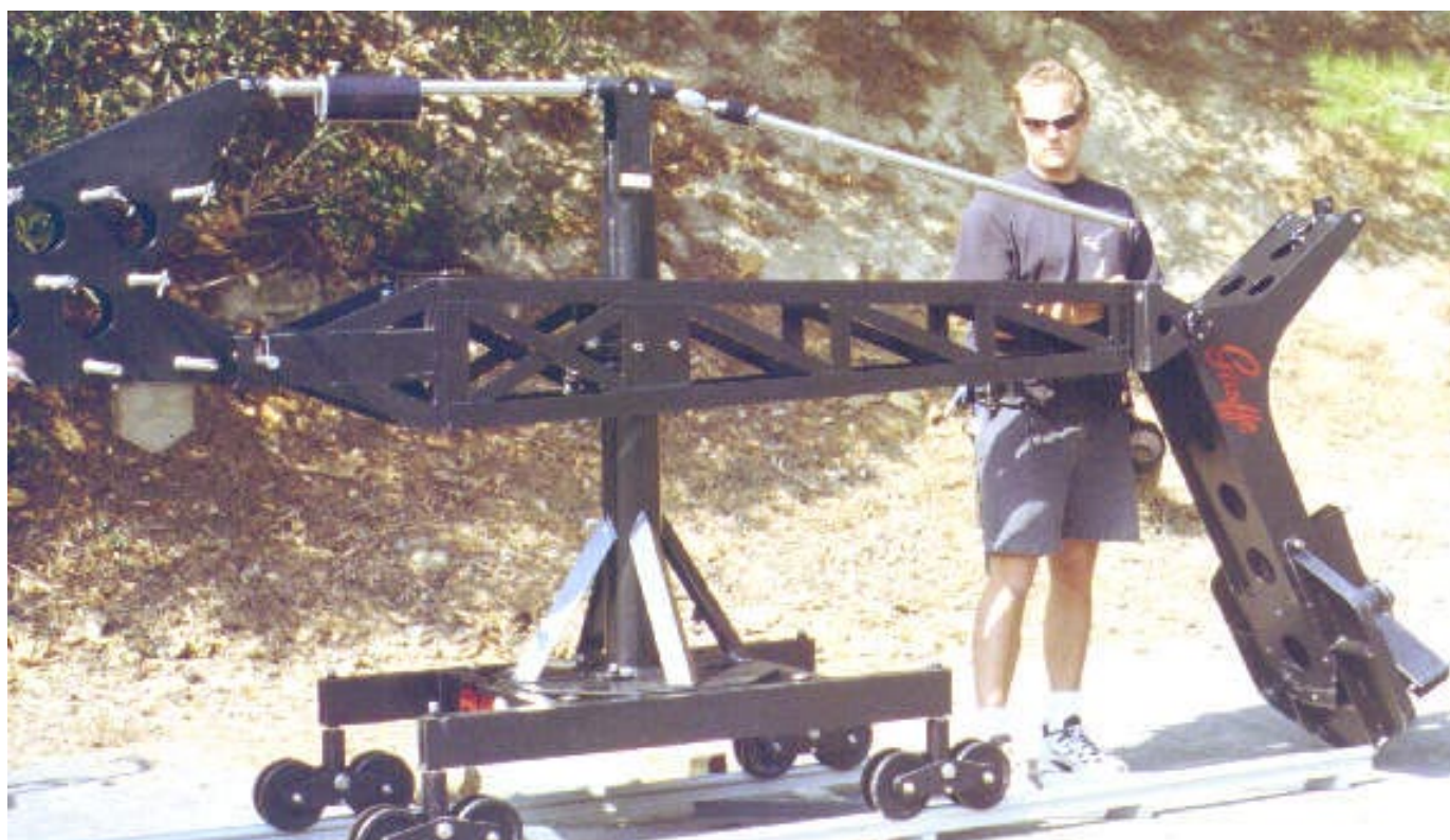
Mode 1 - Operating Platform - Step 16: Attach Operating Platform to the front of Boom #3 with the two retaining bolts found inside Boom #3.
