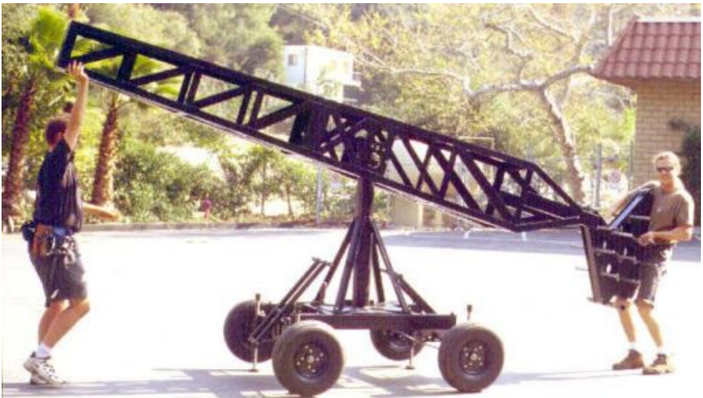
Mode 2 - Operating Platform - Step 6: Add weight box into the slots on the back of Boom #1 and tighten the two retaining bolts (make sure that the weight box shaft isn't resting on the 2 retaining bolts.)
