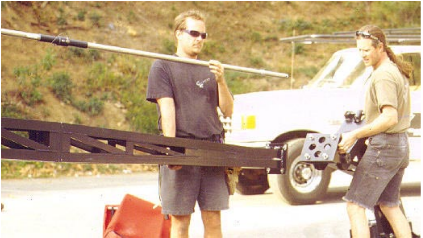
Mode 4 - Remote - Step 17: Attach remote head section to the front of Boom #4.
