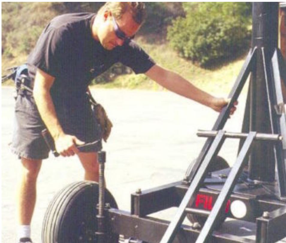
Leveling - Step 4: Place jack handle into top of jack.
