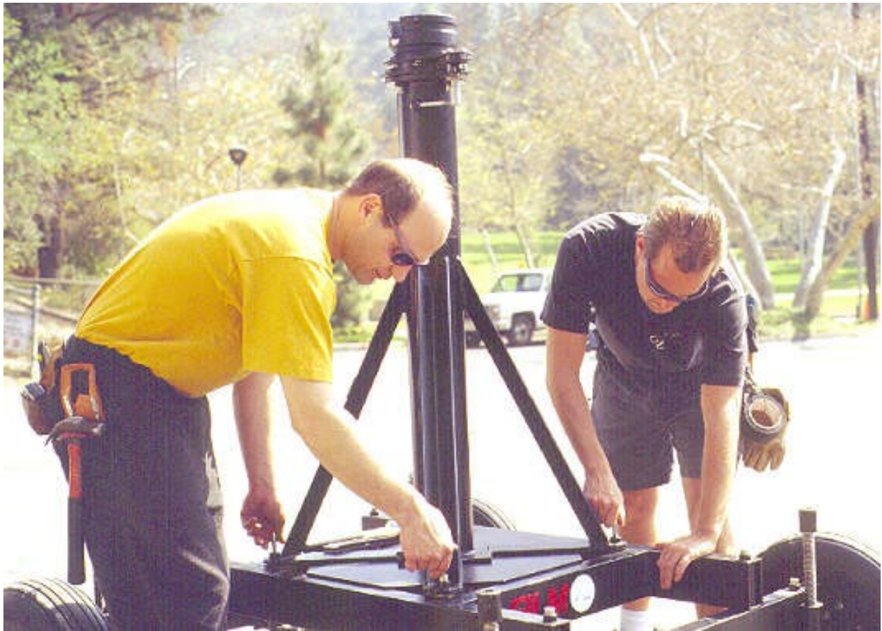
Dolly wide mode - Step 1: Unbolt main post from crane base.
