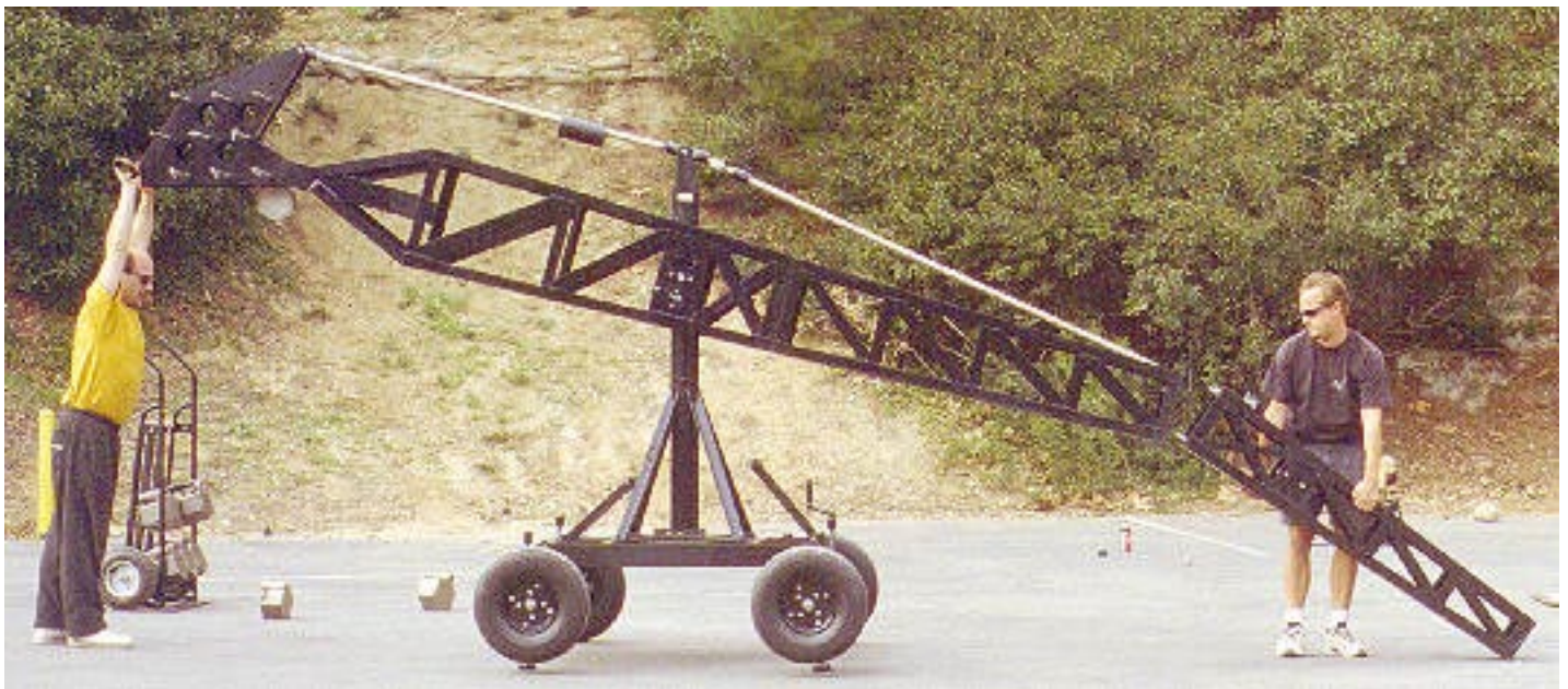
Mode 4 - Remote - Step 10: Attach Boom #3 to the front of Boom #2.
