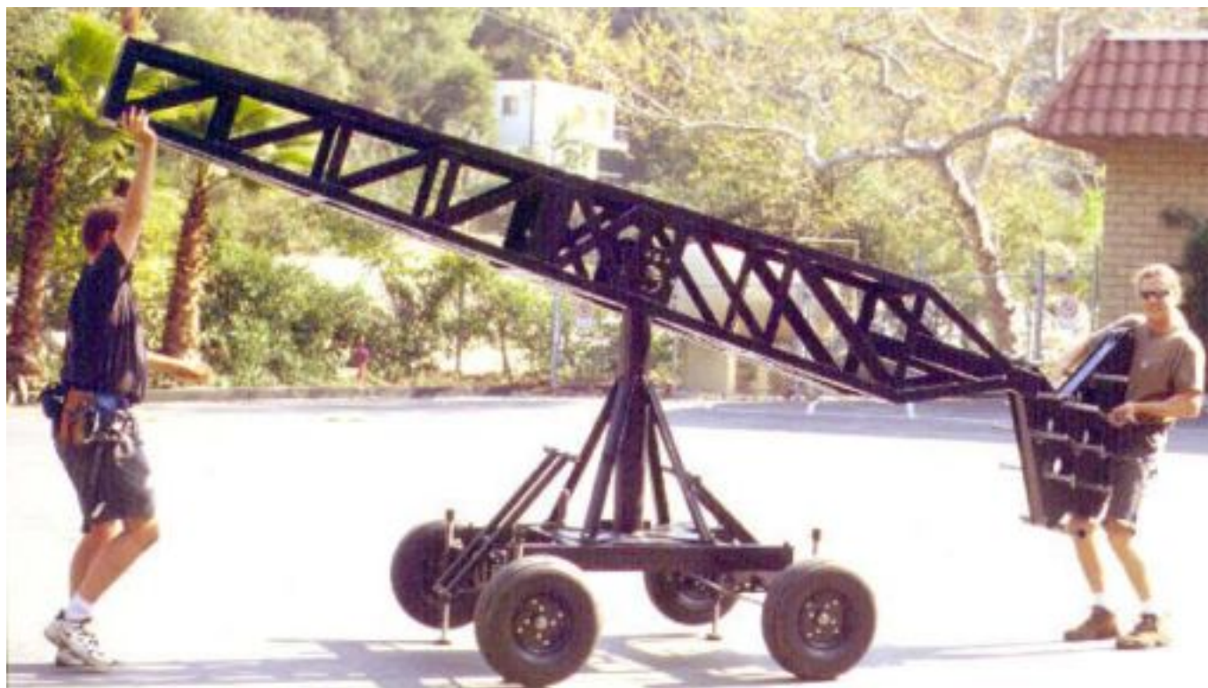
Mode 5 - Remote only - Step 6: Add weight box into the slots on the back of Boom #1 and tighten the two retaining bolts (make sure that the weight box shaft isn't resting on the 2 retaining bolts).
