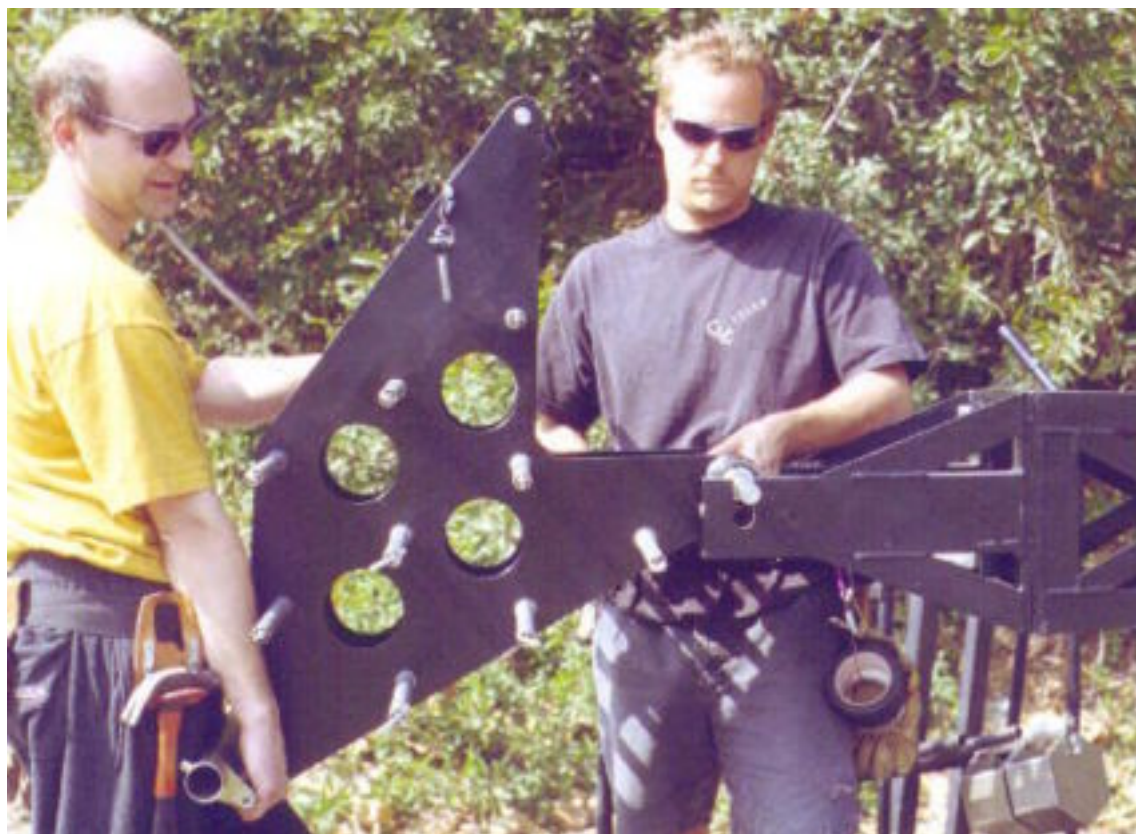
Mode 1 - Operating Platform - Step 14: Place weight box into slots on mini bucket and tighten the two retaining bolts (don't overtighten!)
