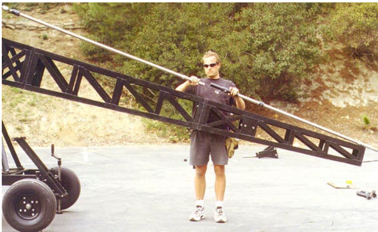
Mode 3 - Remote - Step 12: Add Rod #3 to the front of Rod #2 and secure with the quikpin.
