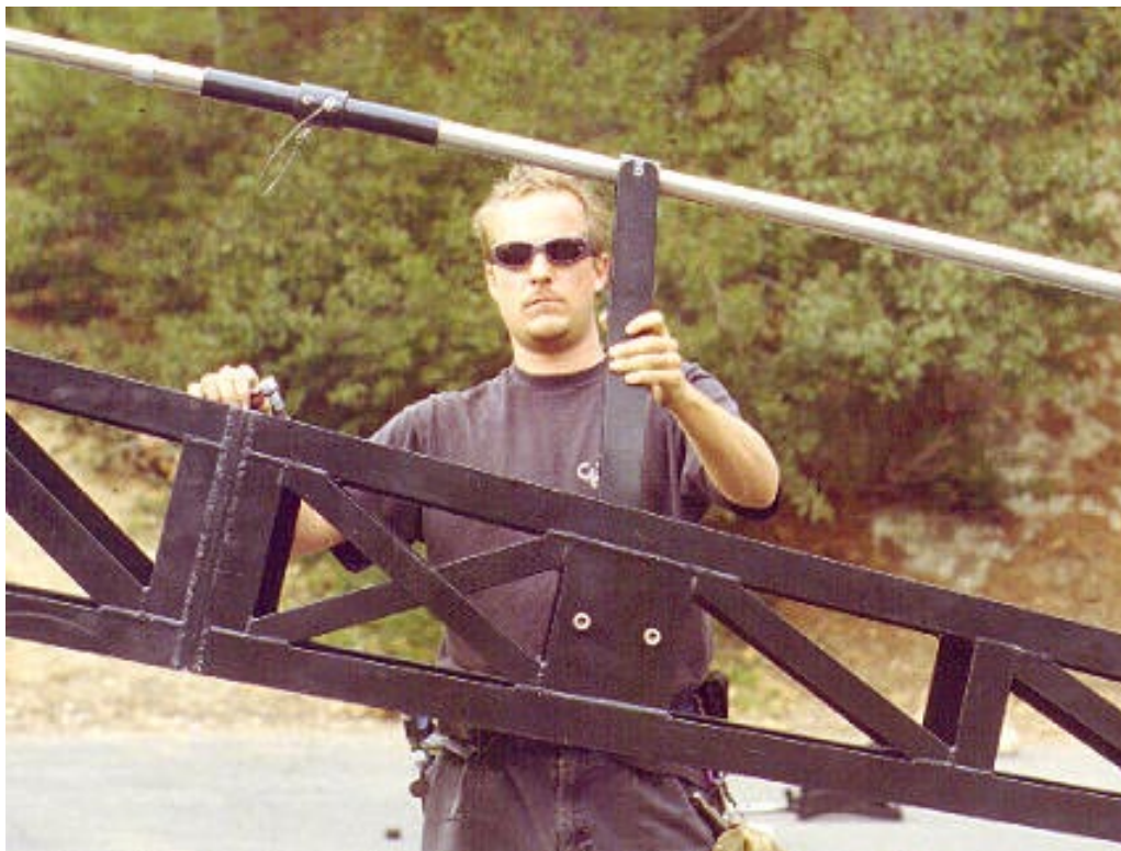
Mode 3 - Remote - Step 14: Click Rod #3 into the top of the rod support bracket.
