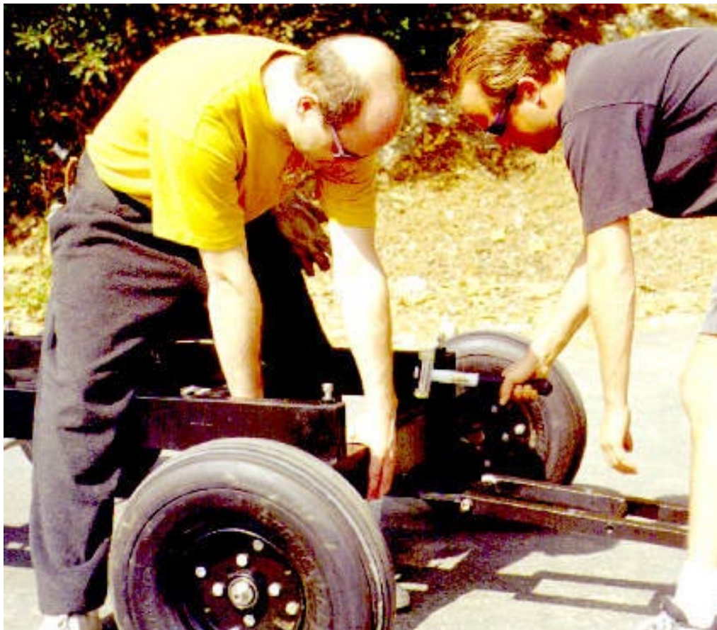
Mode 1 - Operating Platform - Step 2: Remove main crossbar from crane base.
