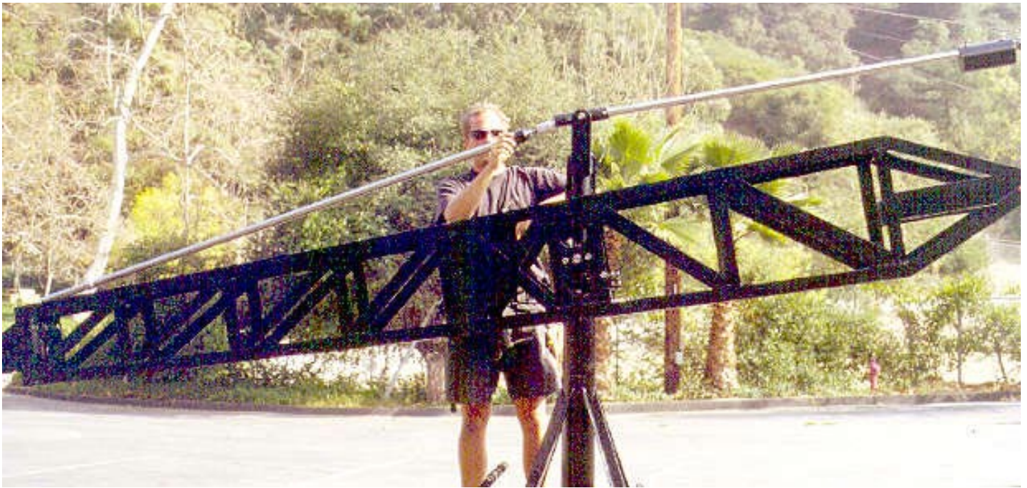
Mode 5 - Remote only - Step 9: Attach Rod # 2 to the front of the pylon (at post) with the quikpin.
