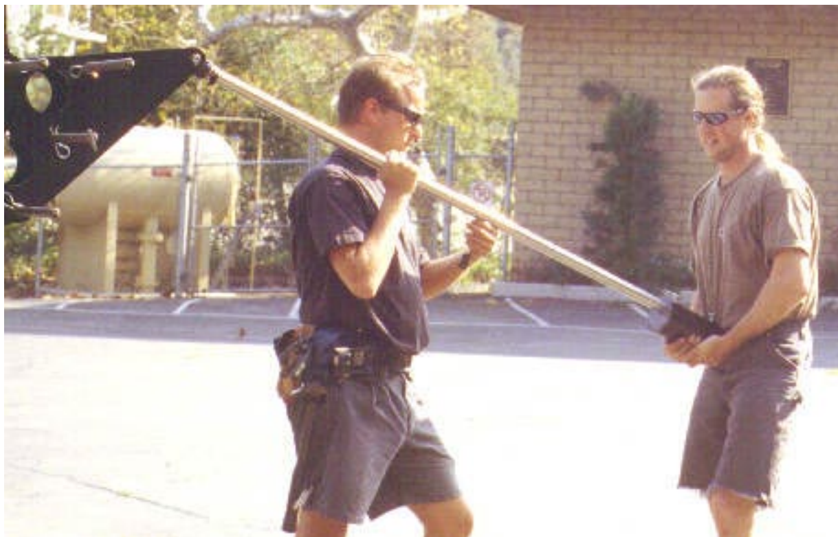
Mode 1 - Operating Platform - Step 15: Attach Rod A (mini rod) to weight box with the quikpin, then add the sliding trim weight. Now attach Rod A to the pylon on the other side with the quikpin.
