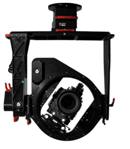
The **POWER-POD-PRIME** is a fully stabilized lightweight remote head that performs exceptionally well with Camera packages of up to 30 kg. Its modular design uses dovetail slides to easily change from 3 to 2 Axis in minutes. It can achieve perfect balance in Pan as well as Tilt Axis using these slides. The custom Zero Backlash drives give the stabilization excellent precision and performance.
